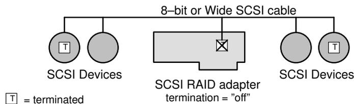
Figure 4. SCSI Single Cable Center Termination
