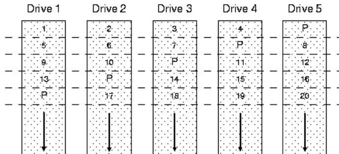
Figure 48. Data Redundancy – Rotating Parity
