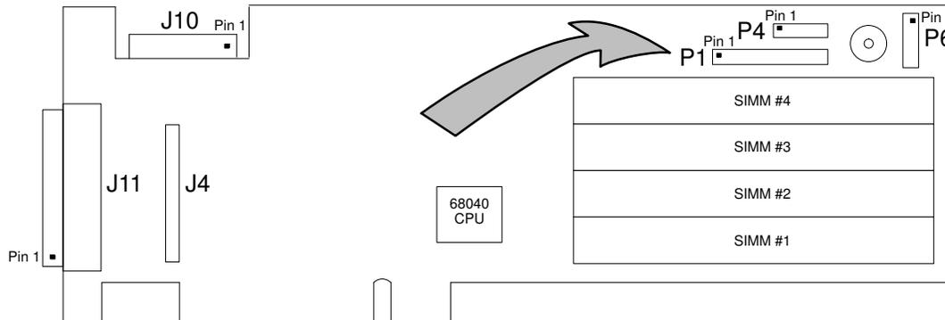
Figure 9. Installing Jumper on P1
