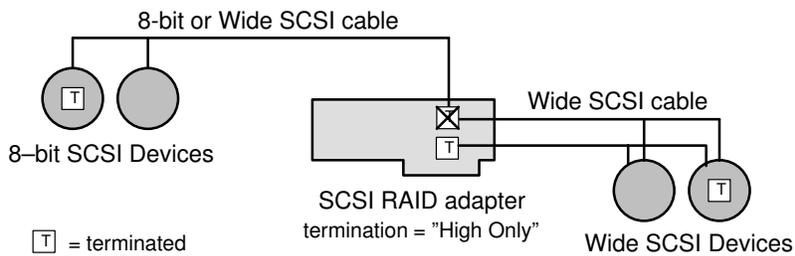
Figure 6. SCSI 8-bit/Wide Cables Termination
