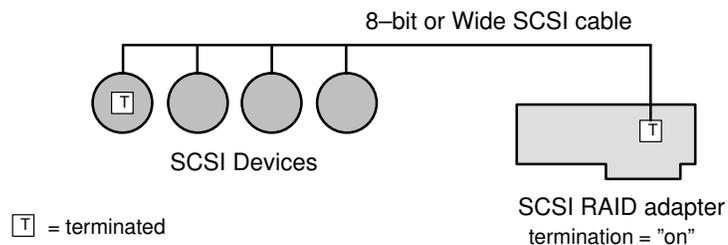
Figure 3. SCSI Single Cable End Termination
