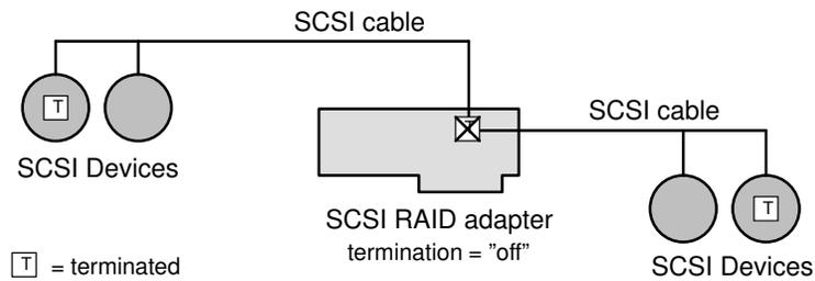
Figure 5. SCSI Two-Cable Termination
