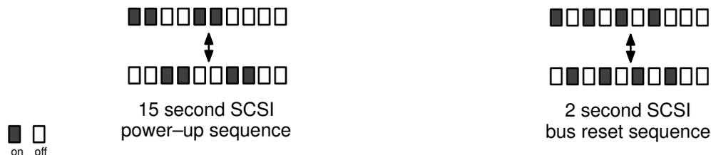
Figure 8. Power–up Sequence LED Display
