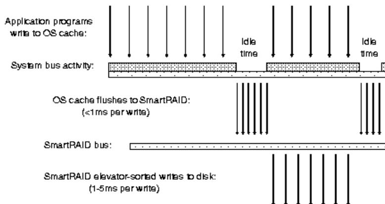
Figure 35. Flushing of OS Cache
