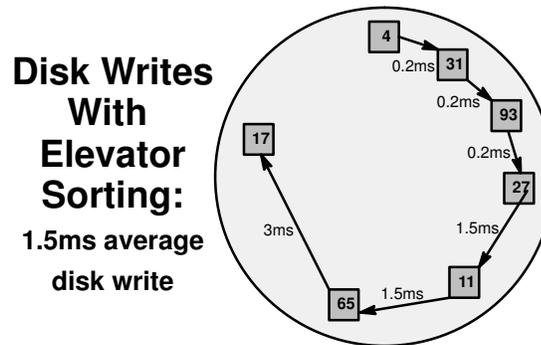
Figure 36. Disk Writes With Elevator Sorting
