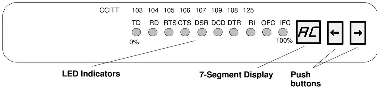
Figure 10. 16 port Concentrator (RAN) Front Panel
