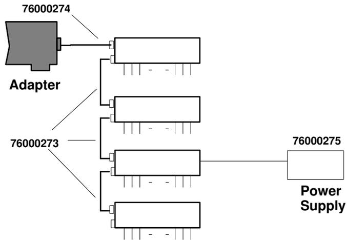
Figure 6. Connection of a 16-Port EIA-232 or RS-422A Concentrator
