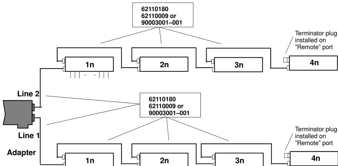
Figure 9. Eight C/CON-16 connected locally
