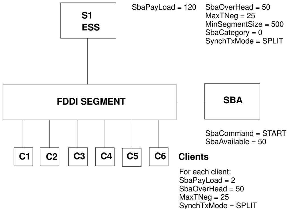
Figure 9. Static Mode Configuration – Example.
