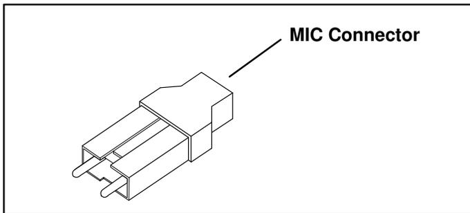
Figure 14. MIC Fiber Loopback Plug.
