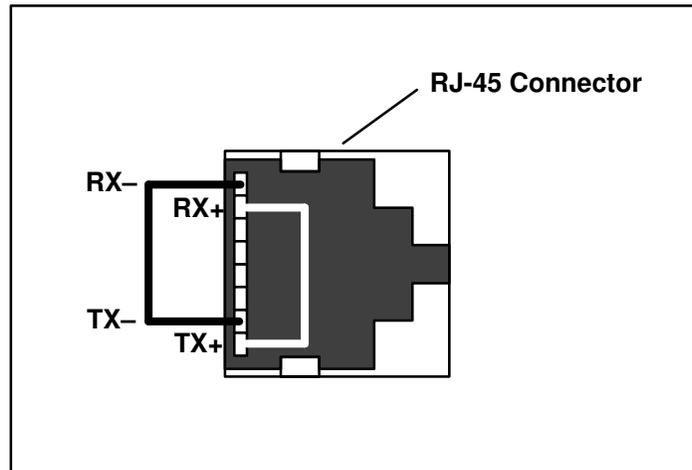
Figure 12. RJ-45 Pinout Showing Loopback.
