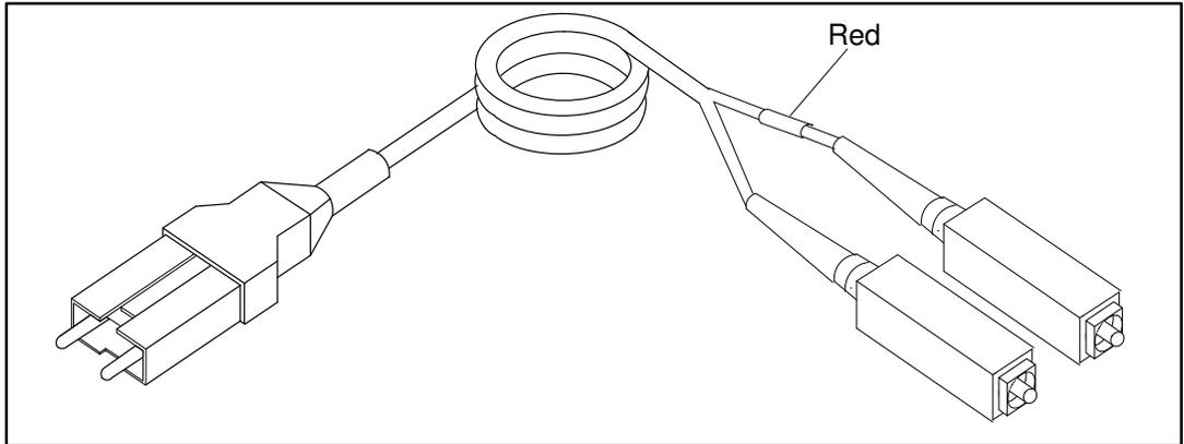
Figure 17. MIC/SC Fiber Cable.
