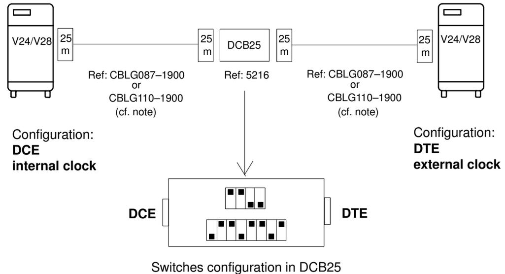
Figure 46. Two Configurations for V24/V28 Direct Connection Link
