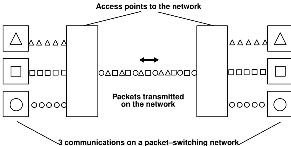
Figure 2. Packet-Switching Network
