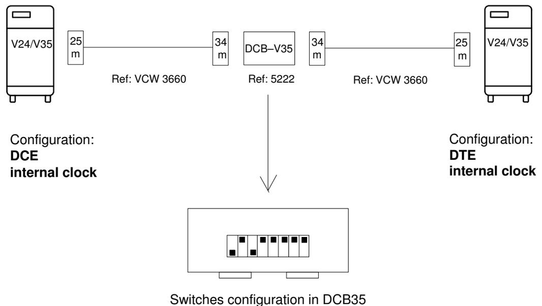
Figure 48. V24/V35 Direct Connection Link
