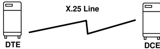
Figure 4. X.25 Direct Connection : DTE and DCE
