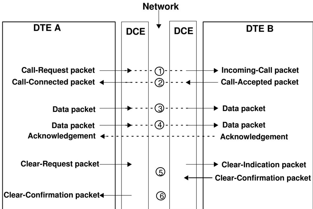
Figure 11. Sequence of packets in an example call over a switched virtual circuit
