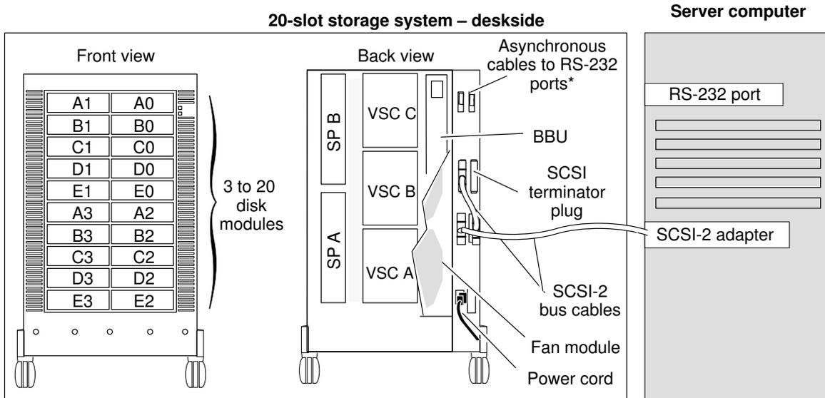
\* Asynchronous cables to RS-232 ports are not needed when you use the ArrayGUIDe utility.
