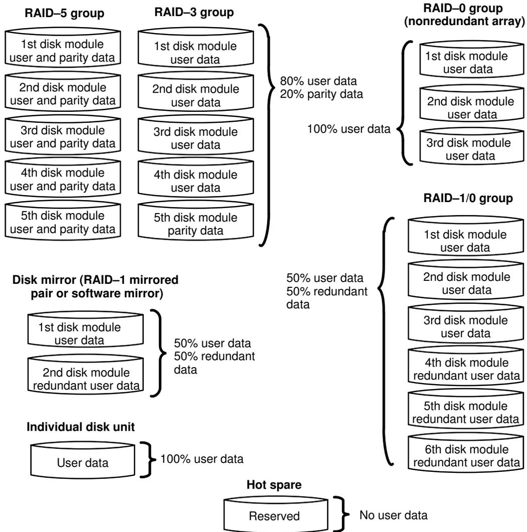
You can use AIX software mirroring for an individual unit or RAID-0 group. For a comparison of software and hardware mirroring, see the section on mirroring, page 24.
