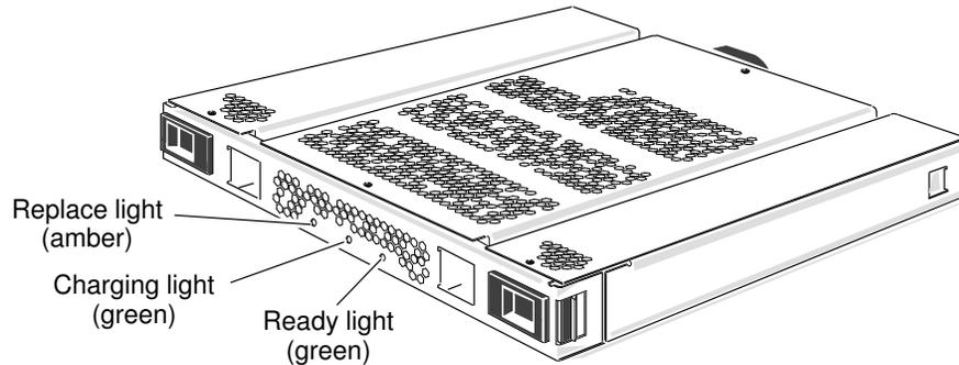
You can install or remove a BBU while the storage system is running.
