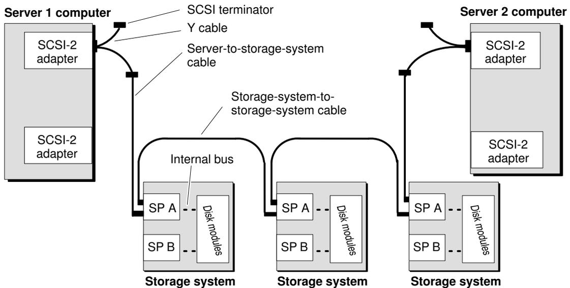
*Note: For the second SCSI bus (since the figure above is the basis for a dual-initiator/dual-bus configuration), the cables would be the same as for the first bus, above.*
