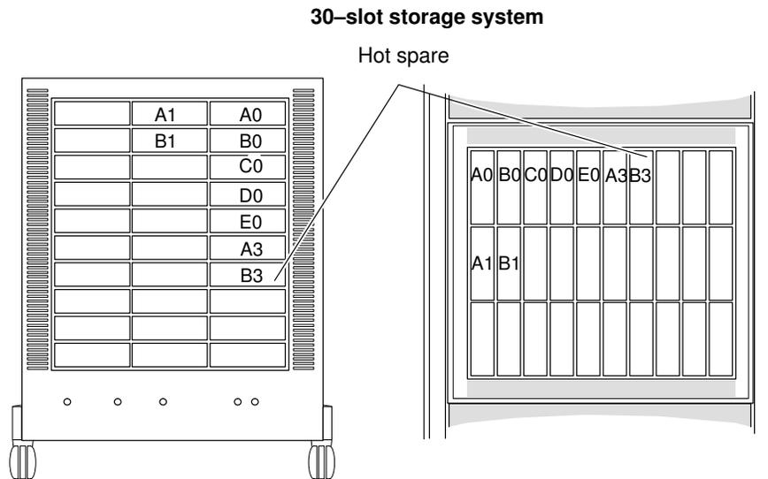
1. RAID-5 group is disk modules A0-E0; RAID-1 mirrored pair is modules A1 and B1; hot spare is module B3.
