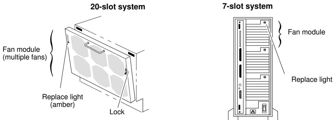
The storage system can continue running after one fan or failure. You can replace a failed fan module while the storage system is running.
