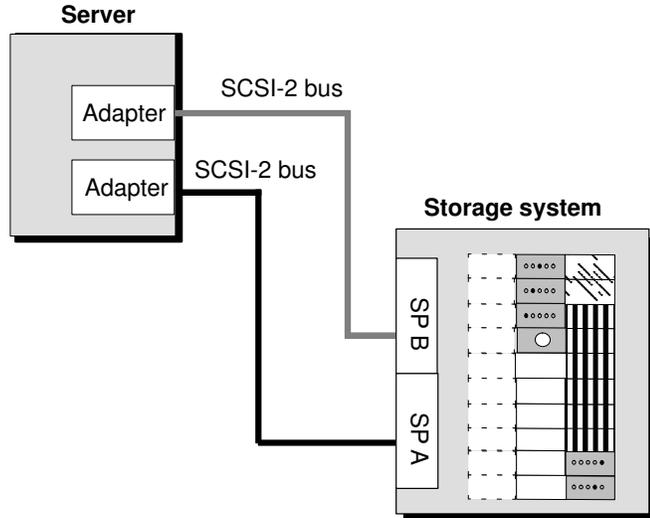
If each disk module shown holds 9 Gbytes, then the storage system provides 81 Gbytes of disk storage with 72 Gbytes highly available. The physical disk configurations are
