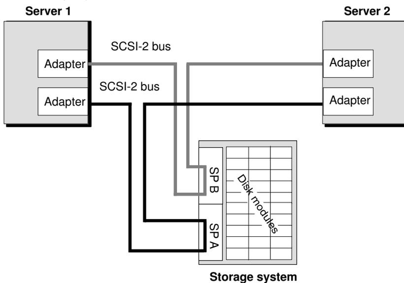
Either SP can control any LUN in the storage system, but only one SP at a time can control a LUN. If one SP cannot access a LUN it controlled (because of a failure), you can transfer control of the LUN to the other SP.
