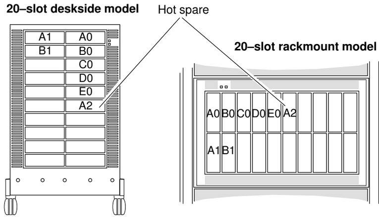
1. RAID-5 group is disk modules A0-E0; RAID-1 mirrored pair is modules A1 and B1; hot spare is A2.
