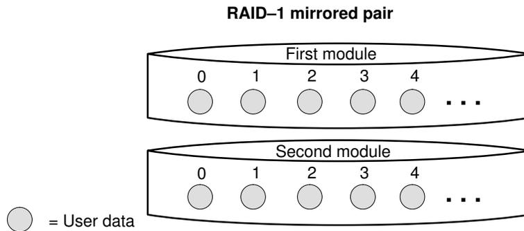
For the most highly available mirror of any type, we recommend that you configure the mirror with each disk module on a different internal SCSI bus.
