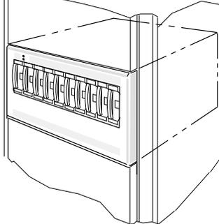
**7-slot disk-array storage system (150 series)**
