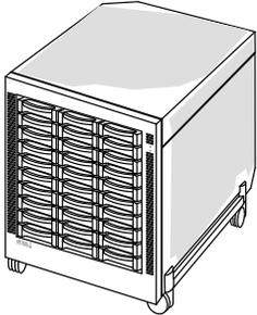
DAS systems let you configure terabytes of disk storage on high-end server systems. And you can easily make this storage highly available using disk arrays and clusters of servers.
