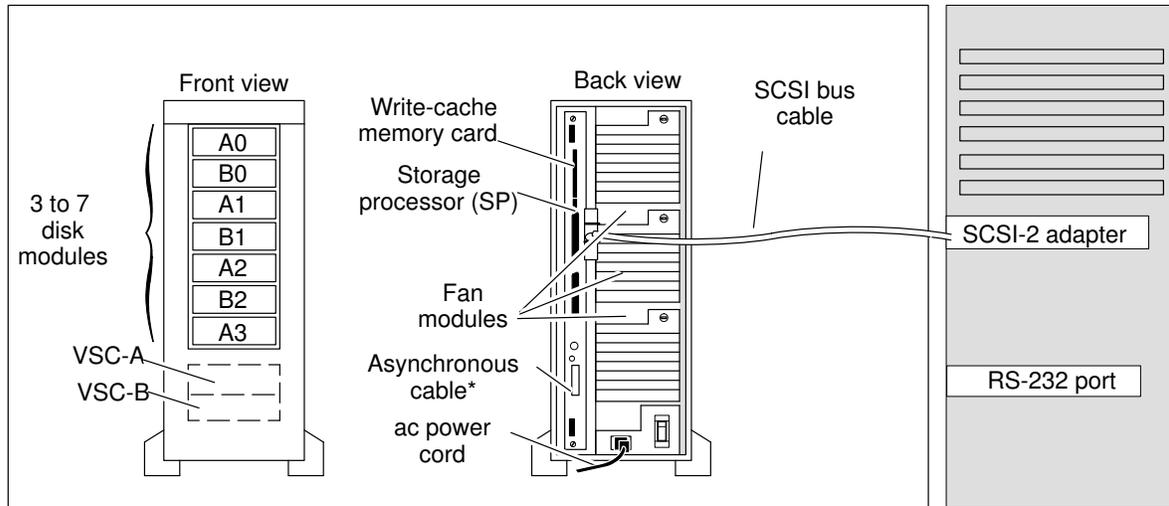
\* Asynchronous cables to RS-232 ports are not needed when you use the ArrayGUIde utility.
