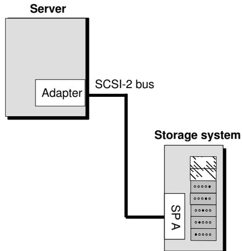
If each disk module shown holds 9 Gbytes, then the storage system provides 45 Gbytes of disk storage, all highly available. The physical disk configurations are
