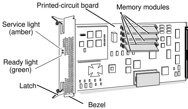
With a specific minimum amount of SP memory, the storage system can support storage-system caching. Storage-system caching enhances performance.
