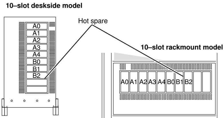
1. RAID-5 group is disk modules A1-A4 and B1; RAID-1 mirrored pair is modules A0 and B0; hot spare is B2.
