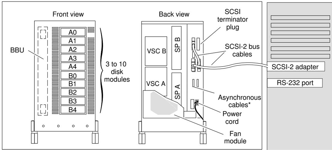
\* Asynchronous cables to RS-232 ports are not needed when you use the ArrayGUIde utility.
