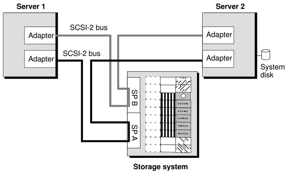
If each disk module shown holds 9 Gbytes, then the storage system provides Server 1 with 54 Gbytes of disk storage, 45 Gbytes highly available; it provides Server 2 with 36 Gbytes of storage, all highly available. Each server has its own SP, which controls that server's storage-system disks; those disks remain primary to that server. The disk configurations are
