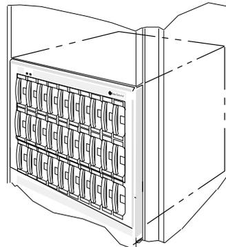
**20-slot disk-array storage system (2x00 series)**
