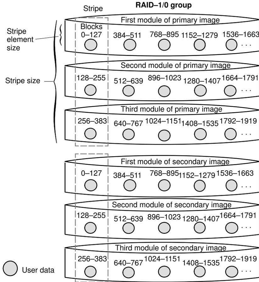
A RAID-1/0 group can survive the failure of multiple disk modules, providing that one module in each image pair survives. So you should bind the modules in each image pair on different internal SCSI buses.
