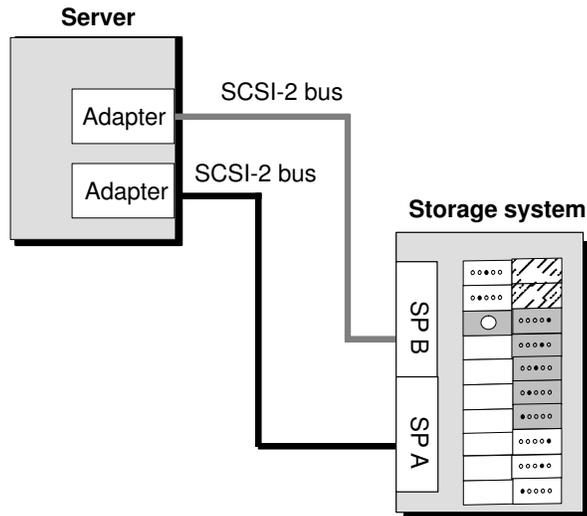
If the disk modules shown here hold 9-Gbytes, then the storage system will provide 36 Gbytes of disk storage with 32 Gbytes highly available. The disk configurations are as follows:
