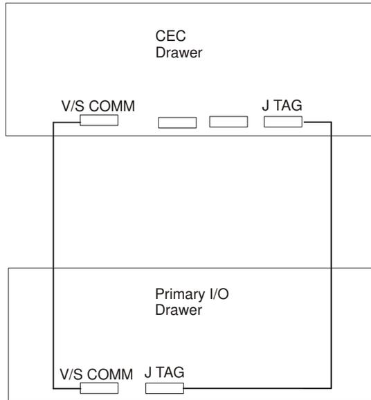
**Note:** The V/S COMM cable includes SPCN signals in addition to other signals.
