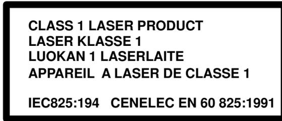
The optical drive in this system unit is certified in the U.S. to conform to the requirements of the Department of Health and Human Services 21 Code of Federal Regulations (DHHS 21 CFR) Subchapter J for Class 1 laser products. Elsewhere, the drive is certified to conform to the requirements of the International Electrotechnical Commission (IEC) 825 (1st edition 1984) and CENELEC EN 60 825:1991 for Class 1 laser products.
