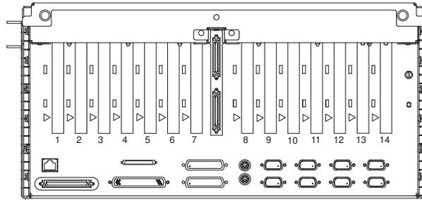
(System Unit Rear View with Numbered Slots)
