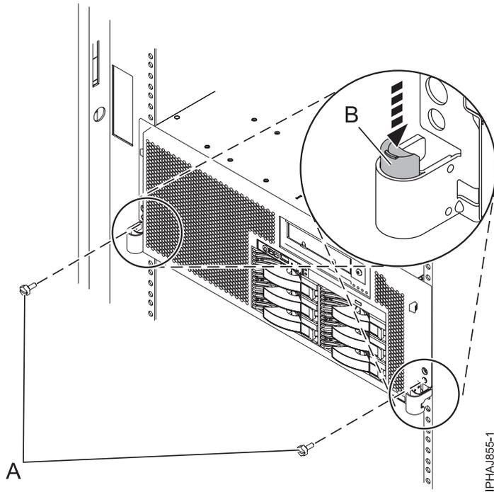
Figure 180. Releasing the rack latches
