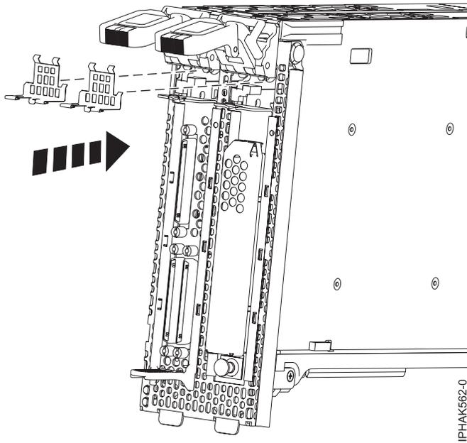
13. Install the cassette assembly into the I/O expansion unit as described in the following substeps:
