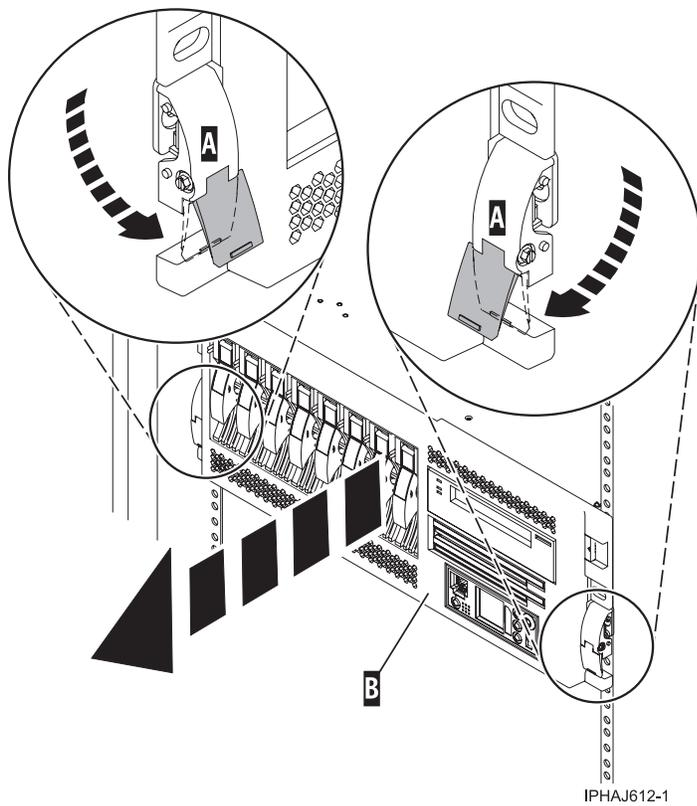
Figure 177. Releasing the rack latches
