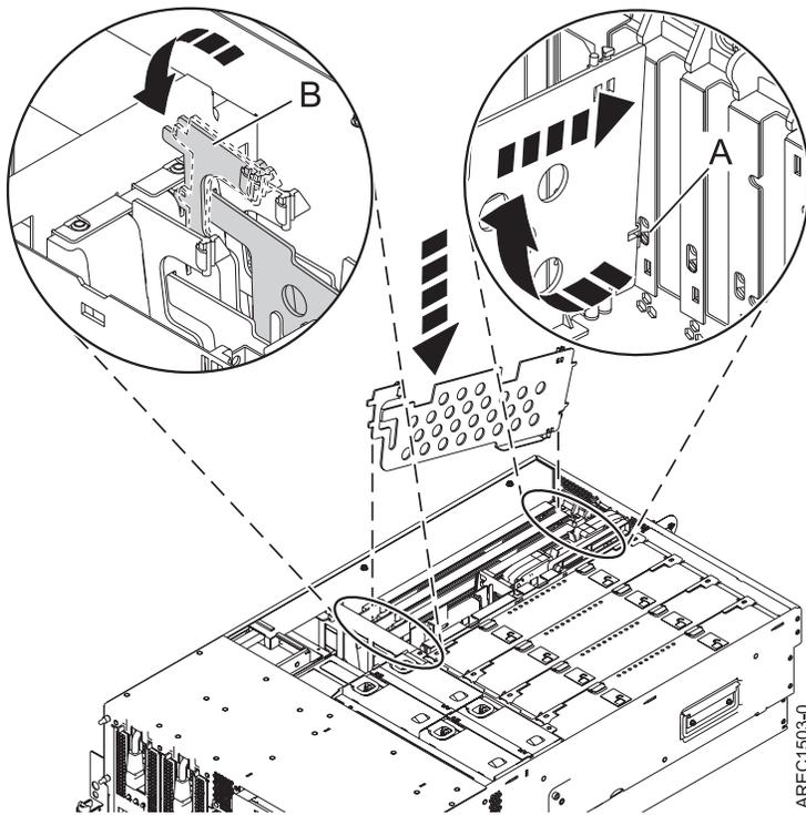
Figure 34. PCI-adapter divider replaced in the system unit
