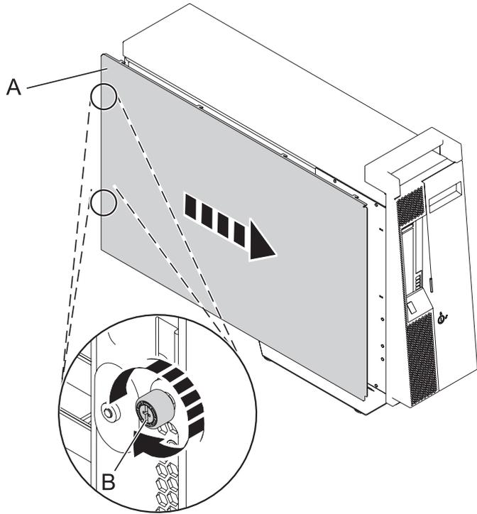
Figure 169. Installing the service access cover on a stand-alone model
