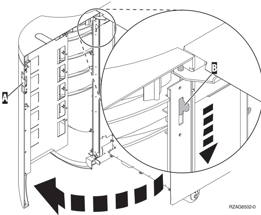
Figure 161. Removing the expansion unit rear door
