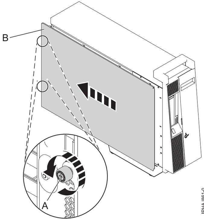
Figure 168. Removing the service access cover from the stand-alone model
