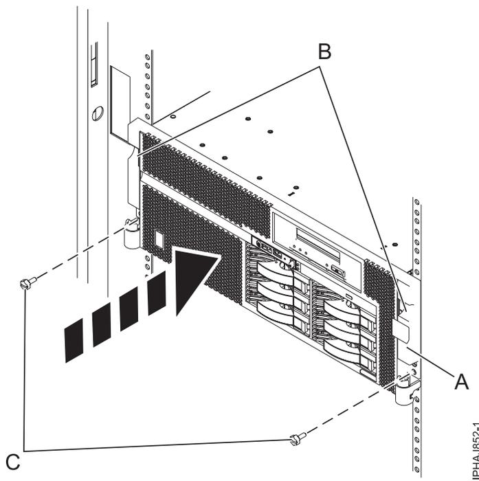
Figure 182. Replacing the thumbscrews
