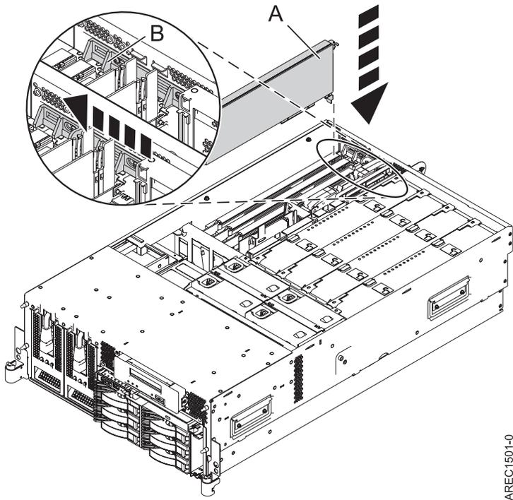
Figure 23. PCI adapter replaced in the rack-mounted system unit
