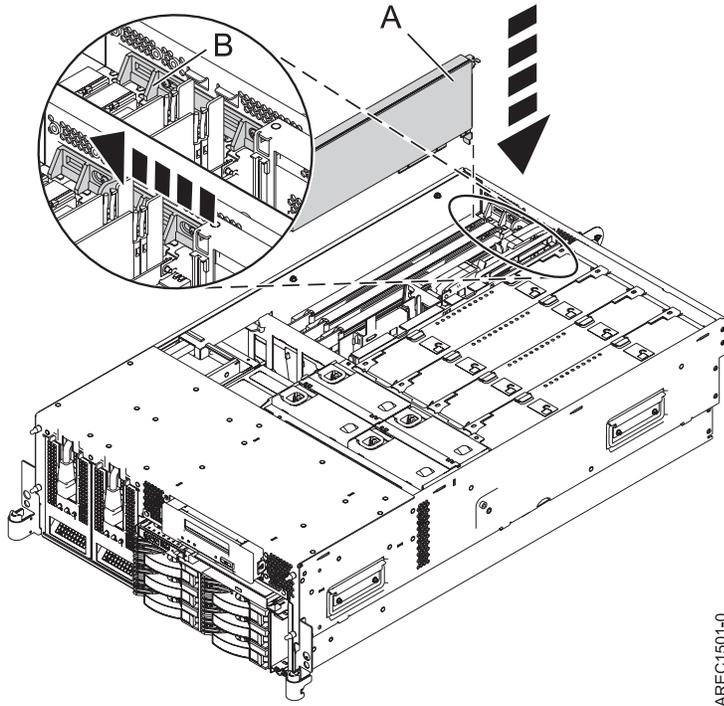
Figure 21. PCI adapter replaced in the rack-mounted system unit
