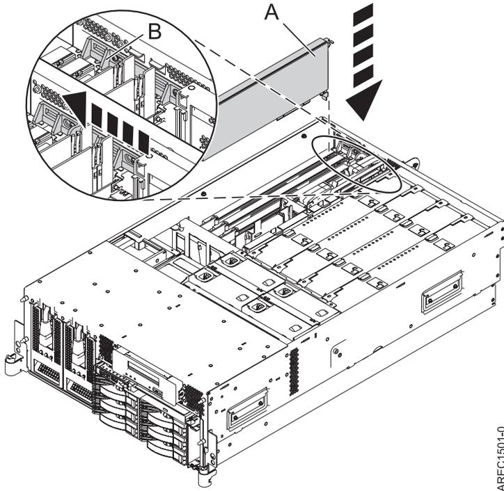
Figure 32. PCI adapter replaced in the rack-mounted system unit
