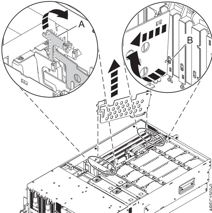
Figure 33. PCI-adapter divider removed from the system unit
