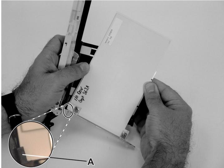
Remove the adapter or blank filler from the cassette linkage assembly by rotating the bottom of the tailstock **A** out, as shown in the illustration. Store the adapter or blank filler in a safe place.
