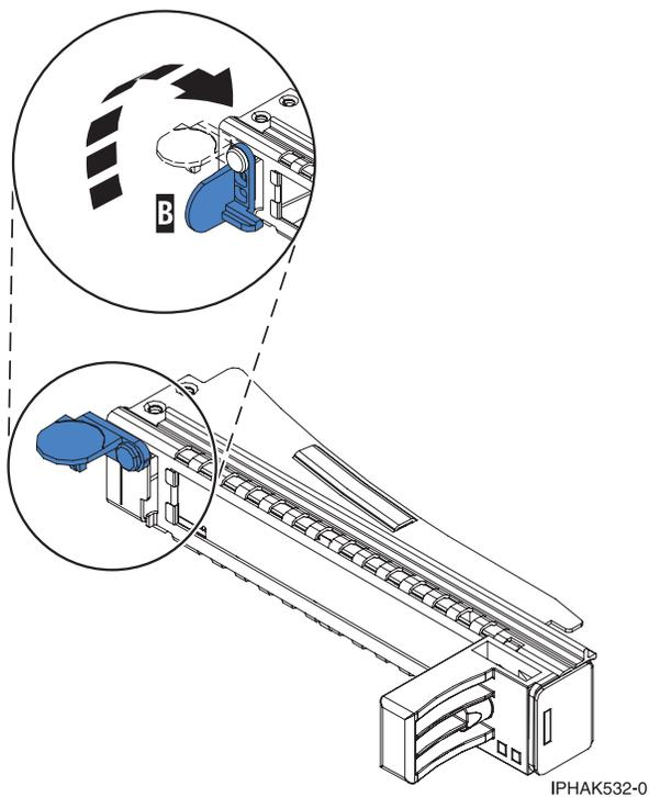
Figure 81. Tailstock clamp in the open position
