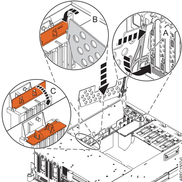
Figure 14. PCI-adapter divider installed in the system unit
