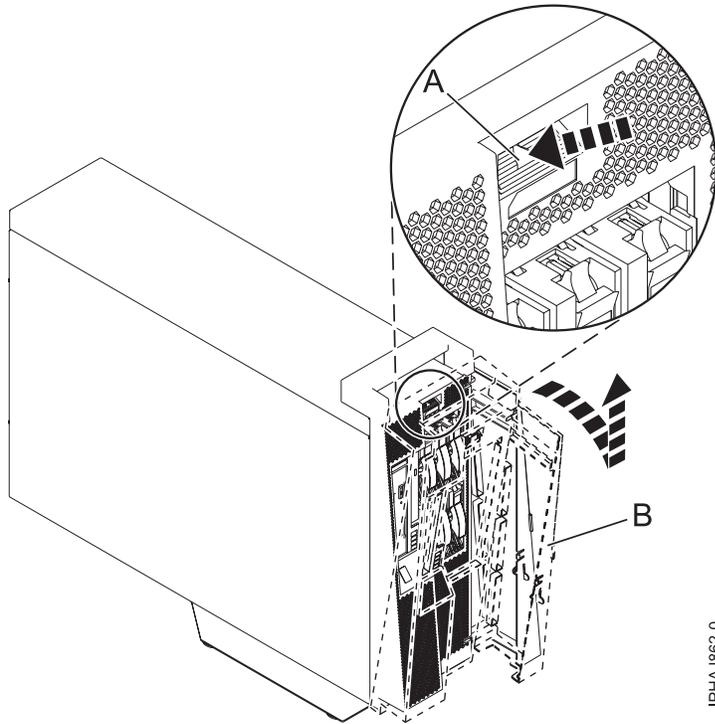
Figure 172. Remove the door from the model
