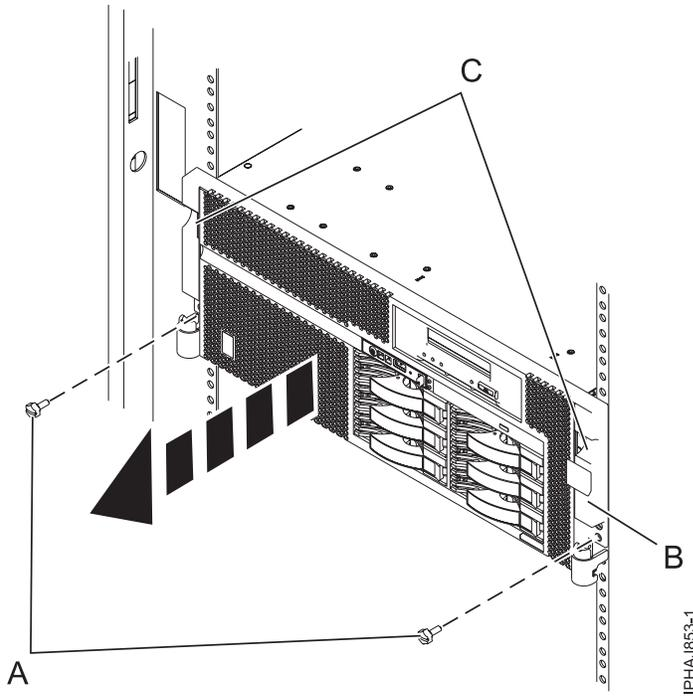
Figure 170. Removing the front cover from a rack-mounted model
