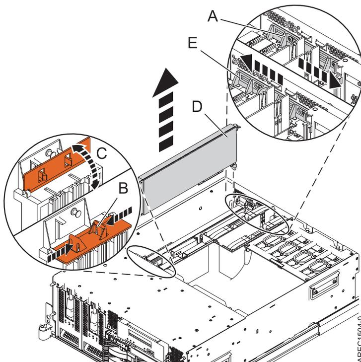
Figure 10. PCI adapter removal
