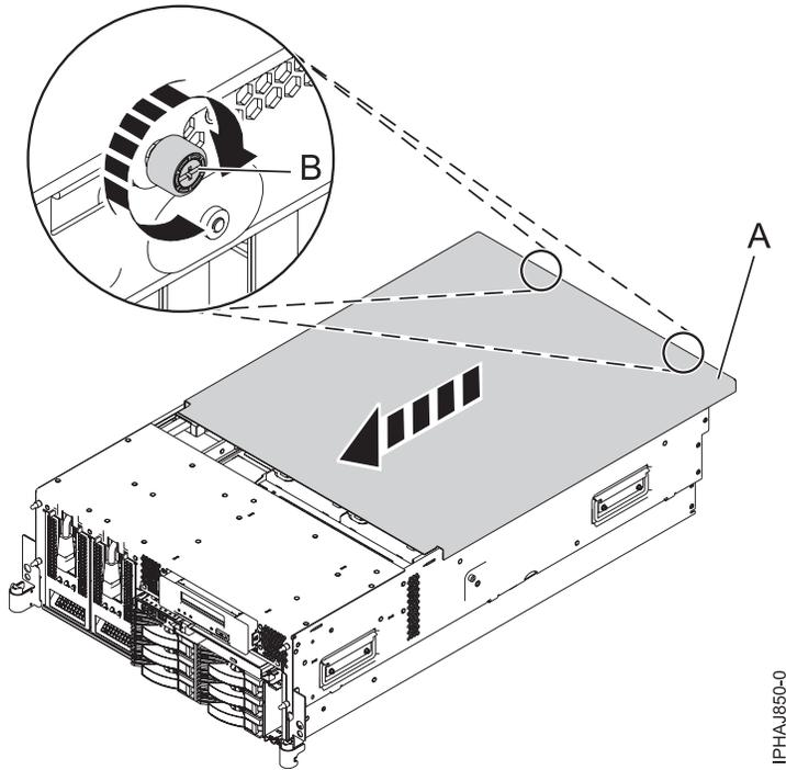
Figure 167. Install the service access cover on the rack-mounted model
