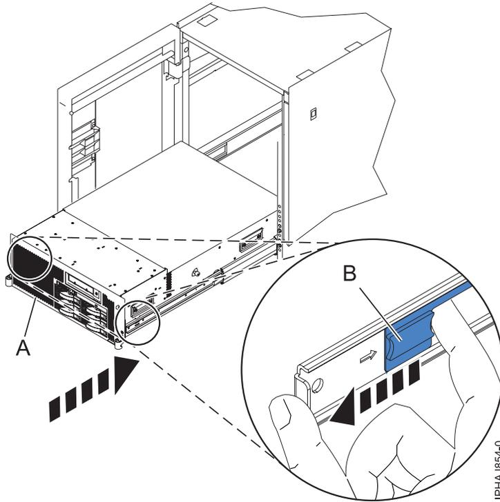
Figure 181. Releasing the rail safety latches
