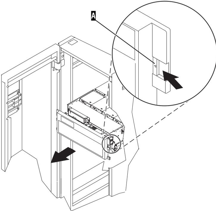
Figure 165. Removing the front cover
