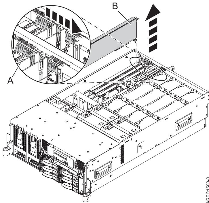
Figure 26. PCI adapter or filler plate removed from the rack-mounted system unit
