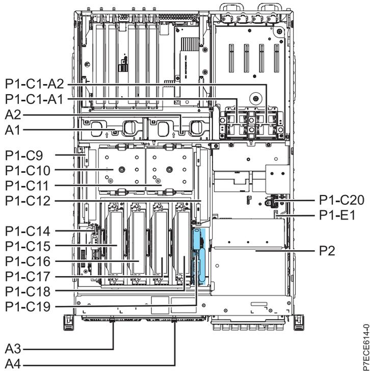
Figure 3. Slot locations of the RAID-10 storage controller (P1-C19) for the 02E/4C, 02E/4D, 05E/6C, or 05E/6D
