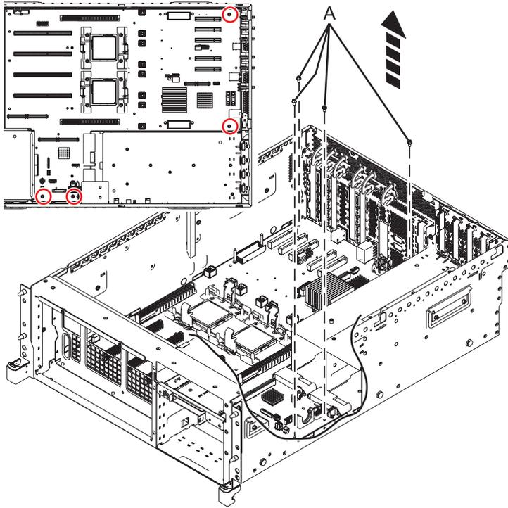
Figure 39. Removing the system backplane from the 02E/4B or 05F/6B
