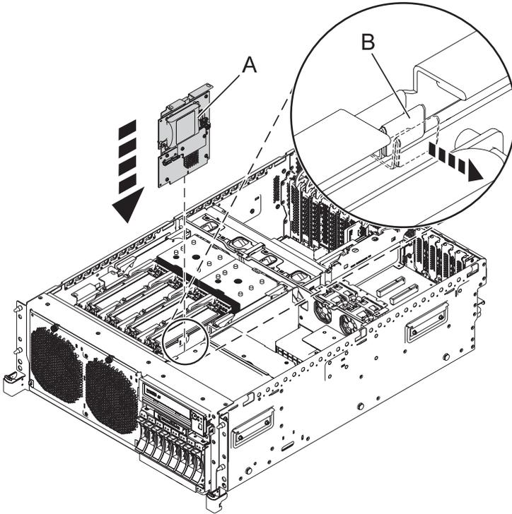
Figure 2. Rack-mounted model RAID-10 storage controller replacement
