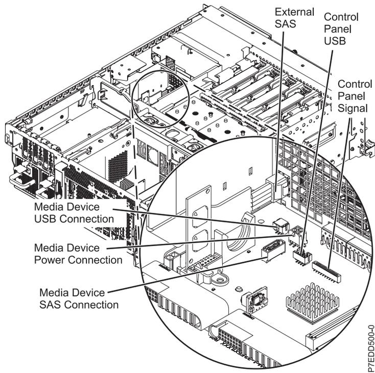
Figure 30. Disconnecting the internal cables
