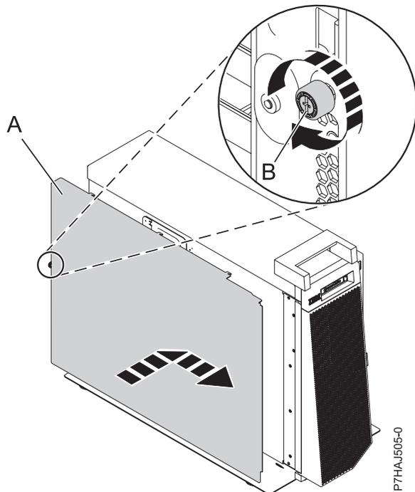
Figure 66. Installing the outside service access cover
