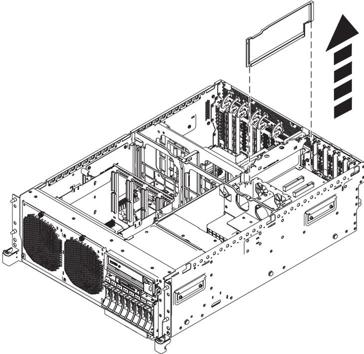
Figure 32. Removing the PCI riser air divider
