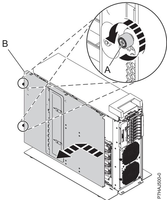
Figure 63. Removing the inside service access cover
