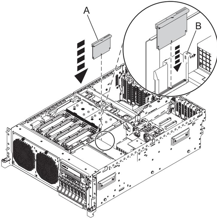
Figure 7. Rack-mounted model RAID enablement card replacement
