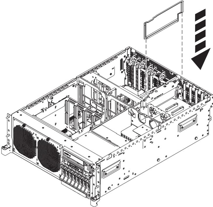
Figure 49. Replacing the PCI riser air divider
