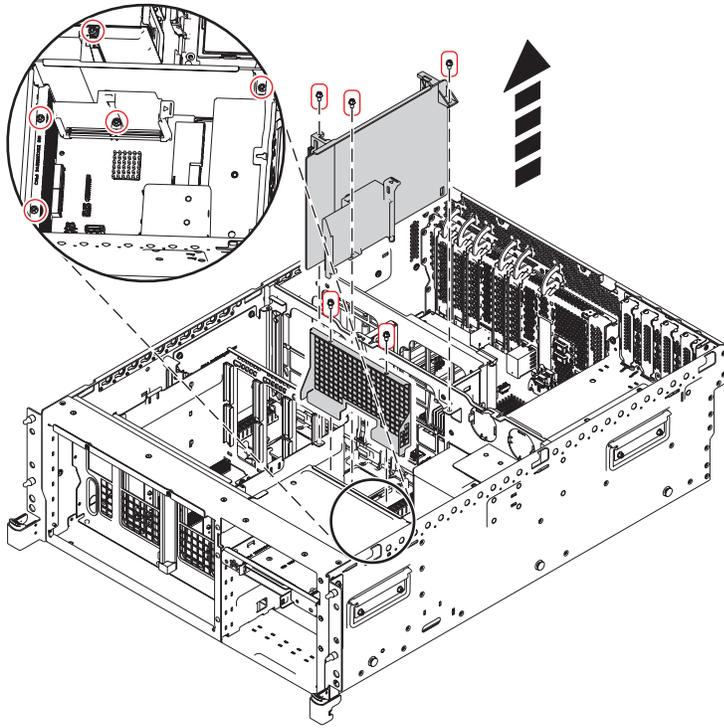
Figure 34. Removing the disk-drive cage shield from the 02E/4B or 05F/6B
