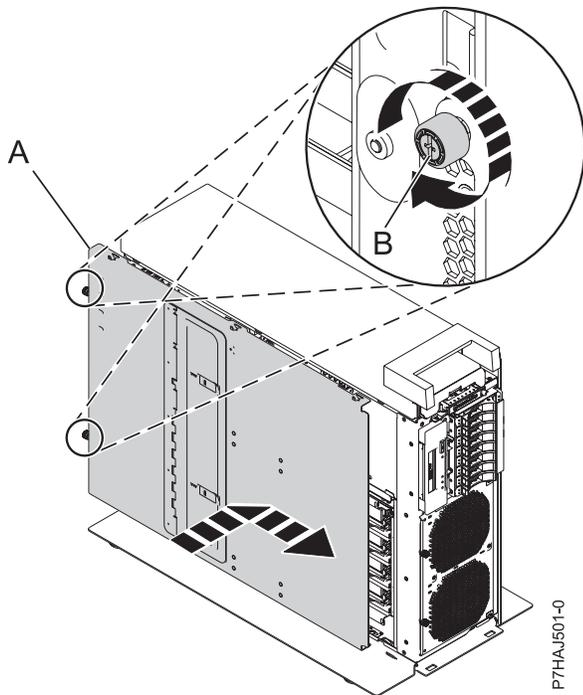
Figure 65. Installing the inside service access cover
