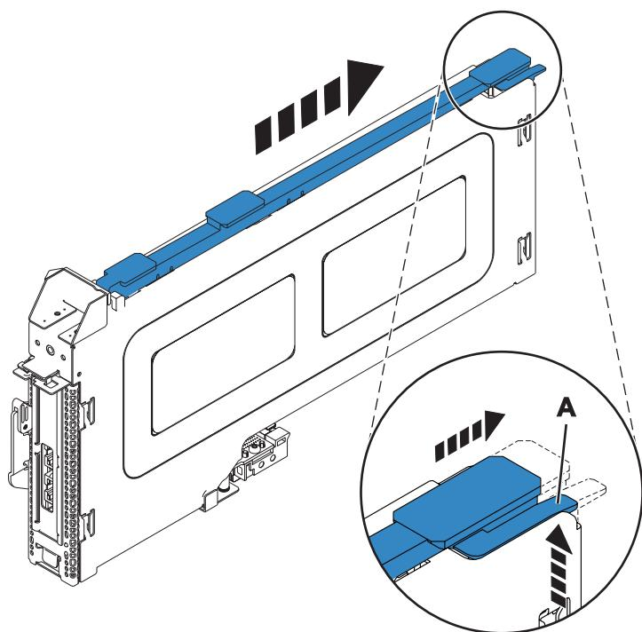
Figure 15. PCI adapter cassette guide rail removed
