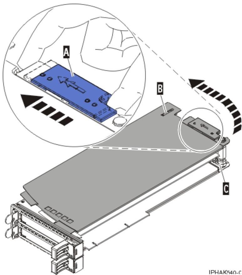
Figure 143. PCI adapter cassette cover replaced
