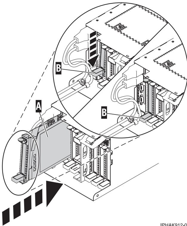
Figure 84. PCI adapter cassette installed in the system unit
