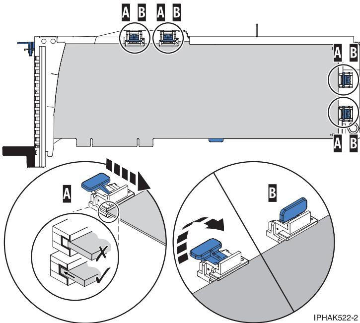
Figure 106. Large adapter in the PCI adapter cassette with the supports and stabilizer in place
