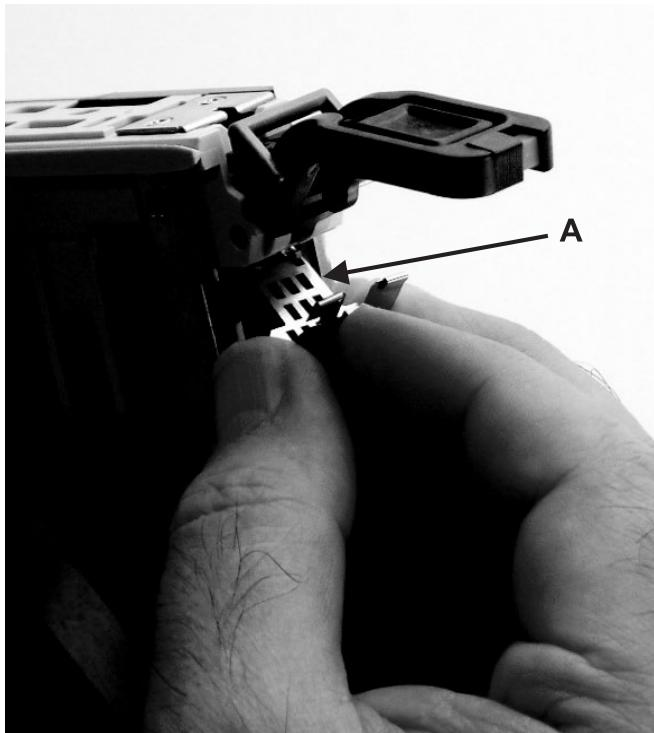
Remove the metal EMC shield **A** from the top of the tailstock.
