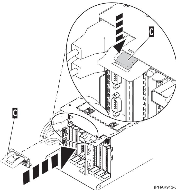
Figure 85. PCI adapter EMC shield in the closed position
