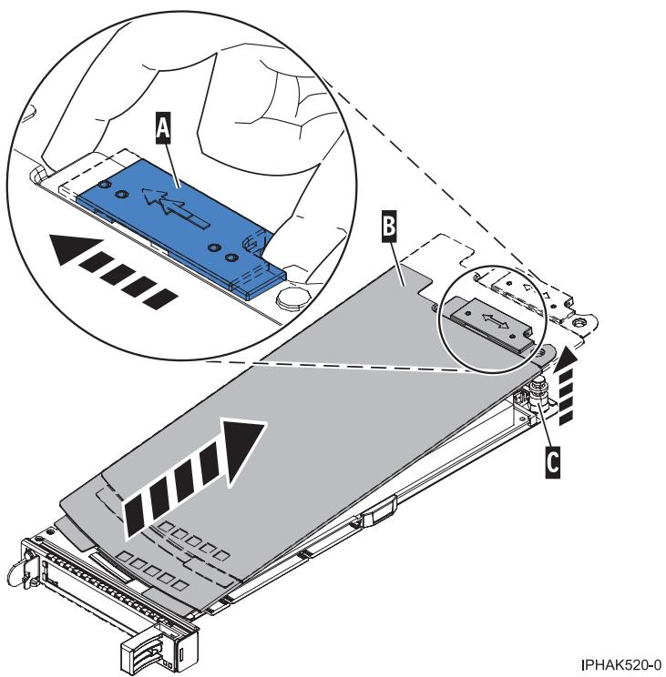
Figure 110. PCI adapter single-width cassette cover removed
