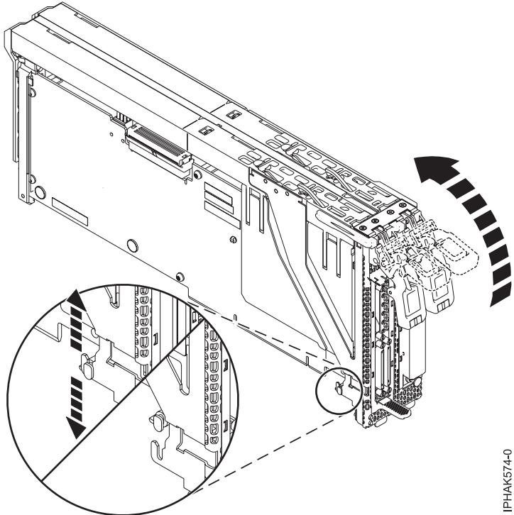
Figure 67. Detaching the face plate
