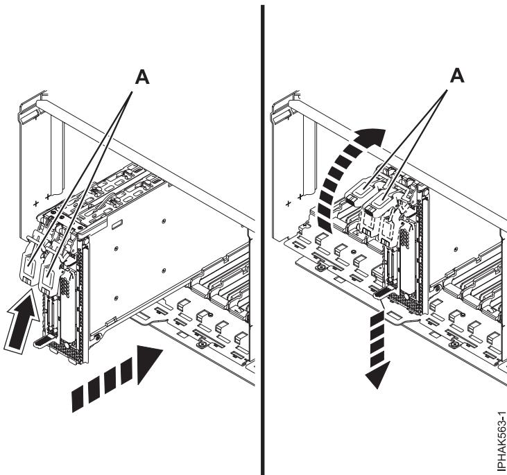
*Figure 61. Installing the cassette assembly into the I/O expansion unit*
