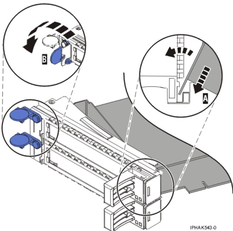
Figure 122. Adapter replaced in the PCI adapter cassette
