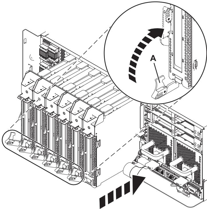
Figure 6. PCI adapter cassette installed in the system unit
