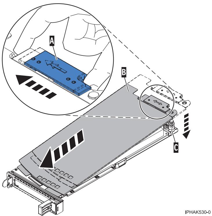
Figure 32. PCI adapter cassette cover replaced
