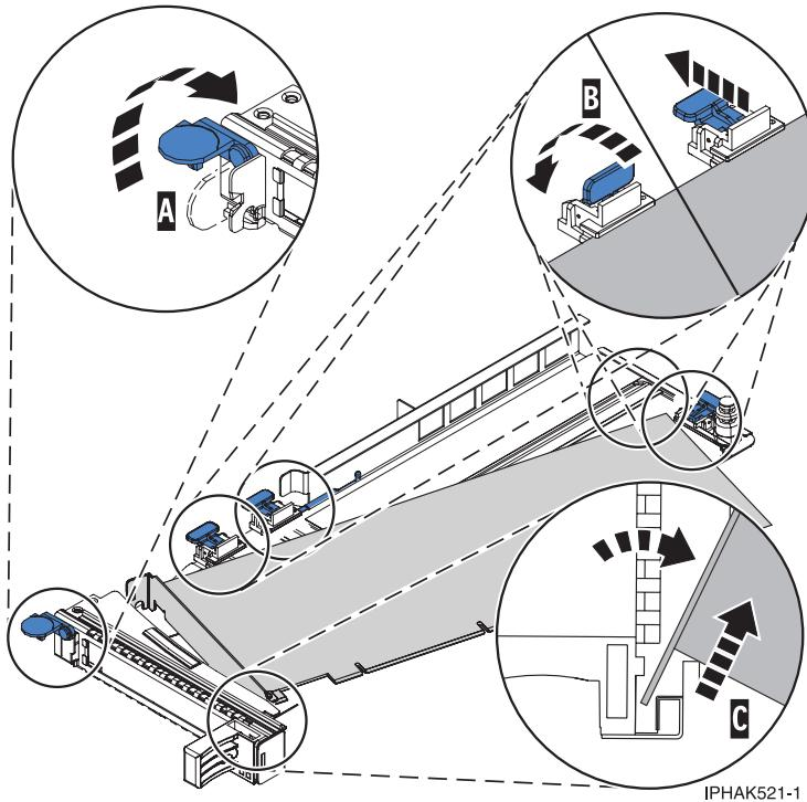
*Figure 116. Adapter removed from the PCI adapter cassette*
