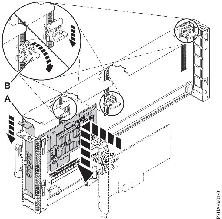
Figure 17. Adapter installed into the PCI adapter single-width cassette
