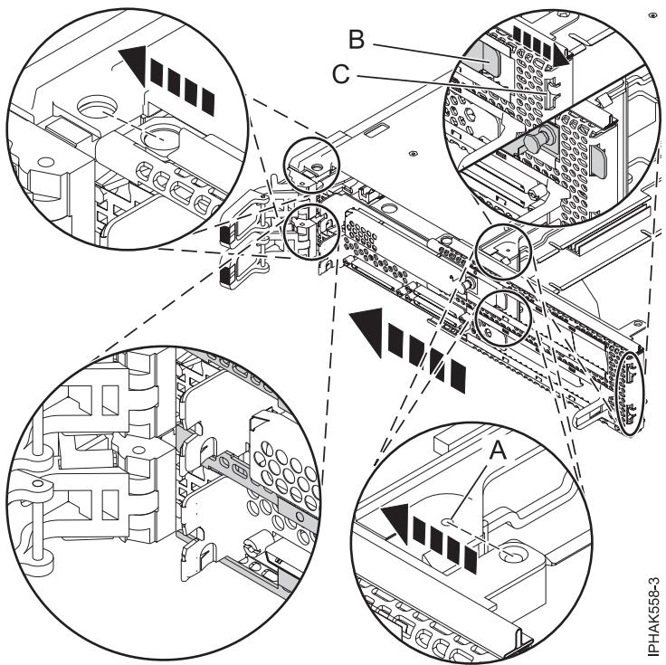
Figure 56. Attaching the face plate
