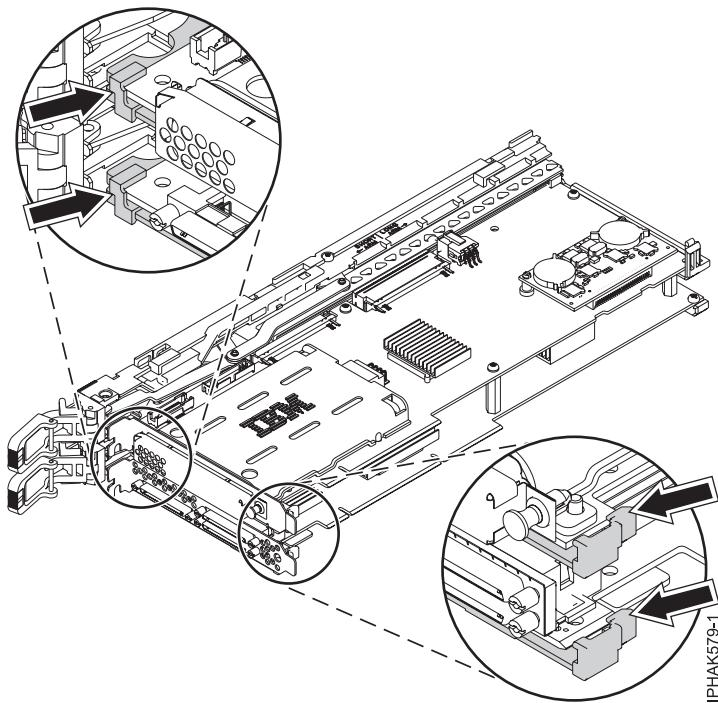
*Figure 71. Detaching the corners of the cassette assembly*
