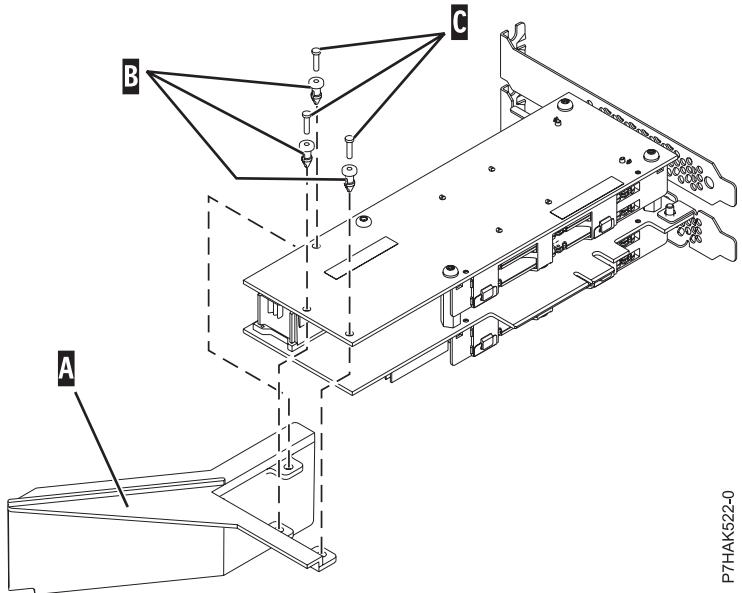
*Figure 145. Installing an air dam onto the new PCIe RAID and SSD SAS adapter*
