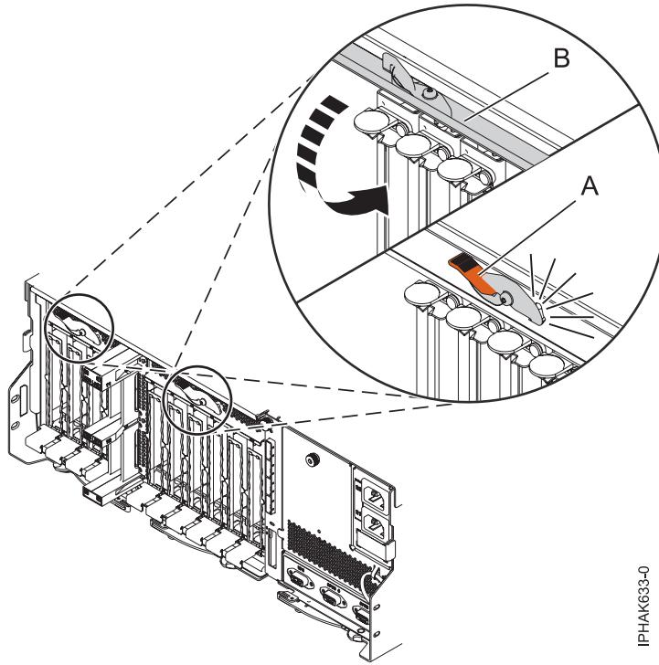
*Figure 126. Closing the access door*
