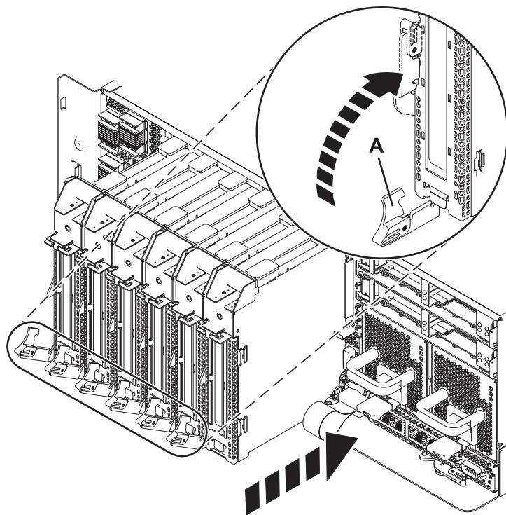
Figure 14. PCI adapter cassette installed in the system unit
