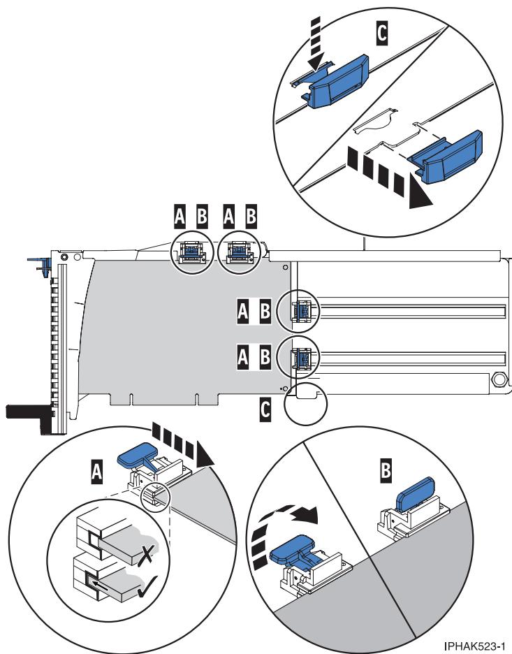
Figure 107. Medium-length adapter in the PCI adapter cassette with the supports in place
