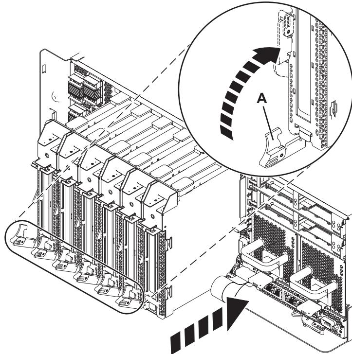
Figure 11. PCI adapter cassette installed in the system unit
