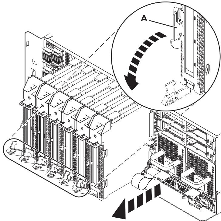
*Figure 5. PCI adapter cassette removed from the system unit*
