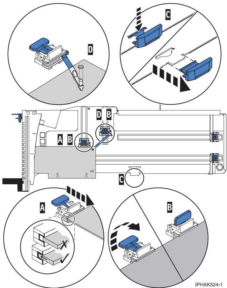
Figure 108. Small adapter in the PCI adapter cassette with the supports and the hookarm in place
