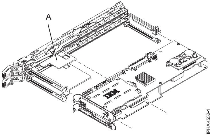
Figure 51. Placing the double-wide adapter in the cassette assembly
