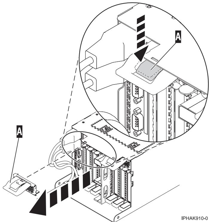
Figure 82. Remove the EMC shield
