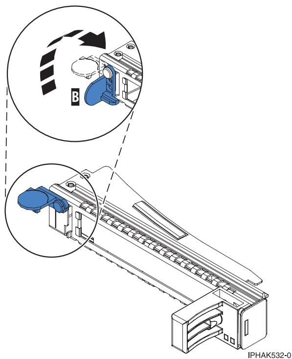
*Figure 27. Tailstock clamp in the open position*
