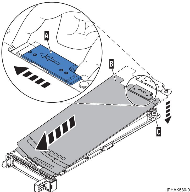
Figure 109. PCI adapter cassette cover replaced
