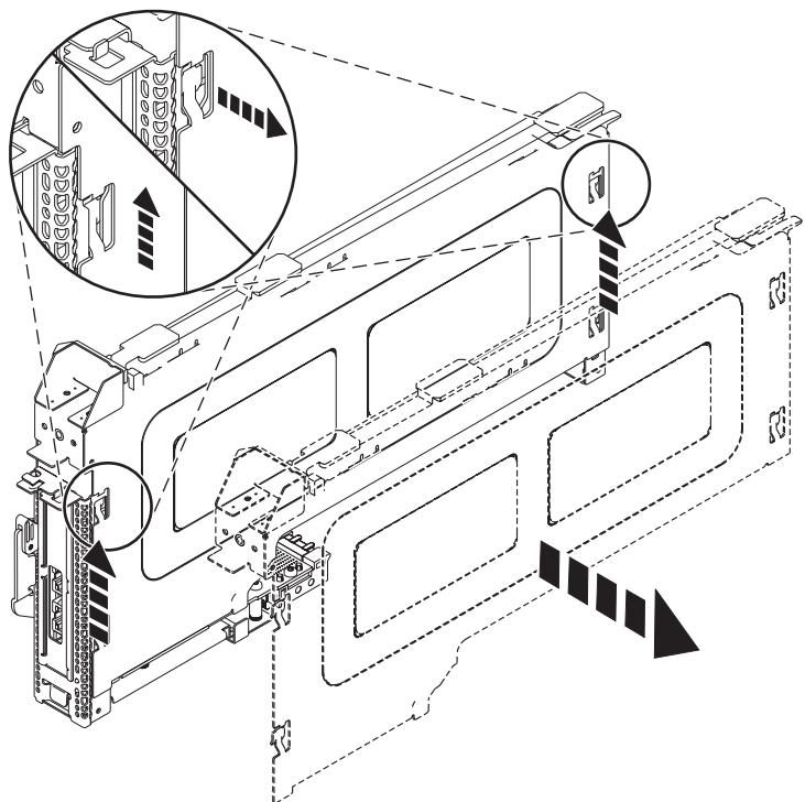
Figure 16. PCI adapter cassette cover removed
