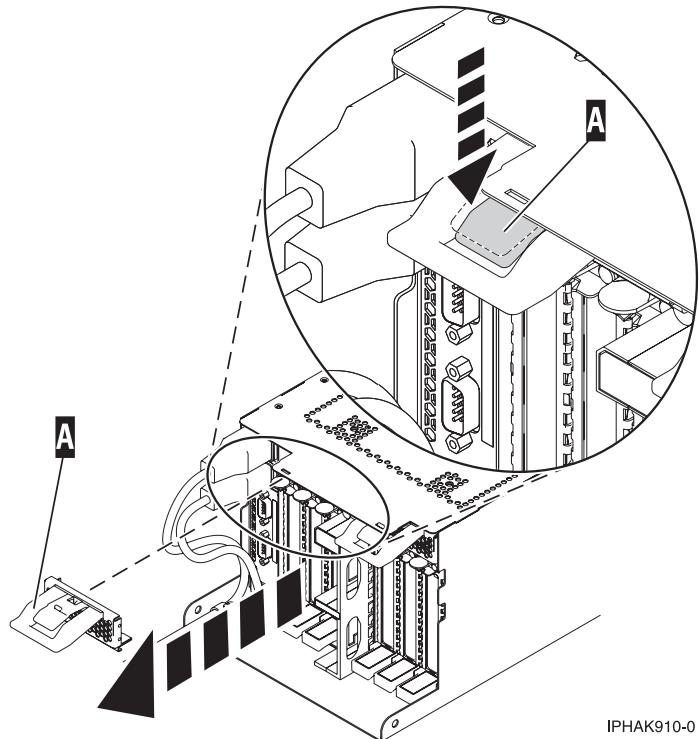
Figure 74. Remove the EMC shield
