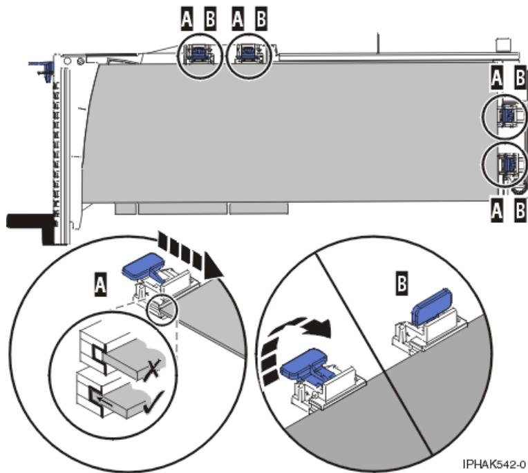
Figure 123. Long adapter in the PCI adapter cassette with the supports and stabilizer in place
