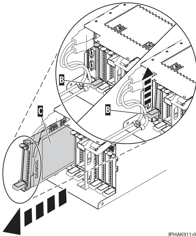
Figure 87. PCI adapter cassette removed from the system unit
