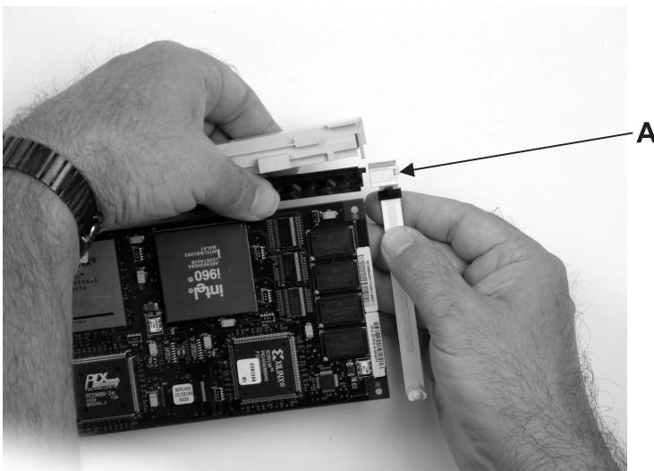
Each adapter arm has a release tab **A** that allows the arm to be moved away from the adapter in the cassette assembly. Use your fingernail to lift the tab, which allows the arm to be moved away from the adapter. Lift the release tab on the large adapter arm, and slide it off the cassette linkage assembly.
