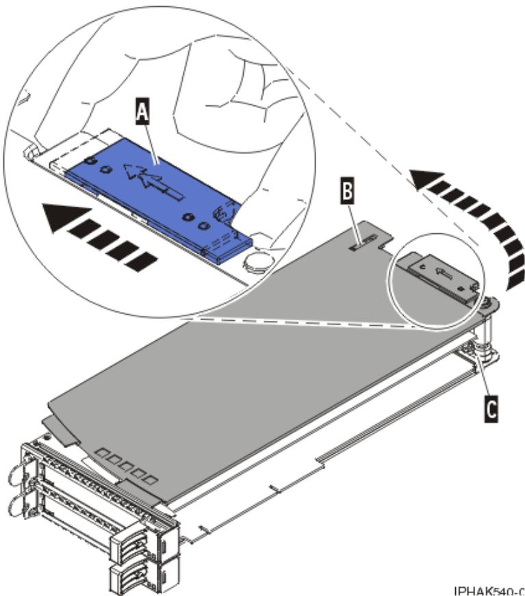
Figure 124. PCI adapter cassette cover replaced
