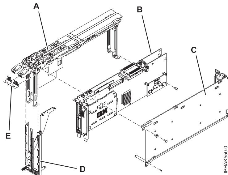
*Figure 48. PCI-X double-wide, quad-channel Ultra320 SCSI RAID Controller and the main parts that make up the cassette assembly*
