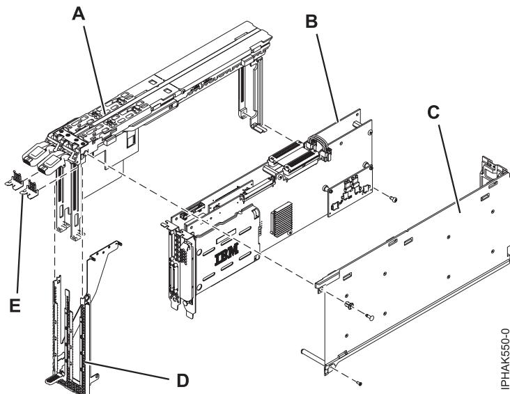
Figure 62. PCI-X double-wide, quad-channel Ultra320 SCSI RAID Controller and the main parts that make up the cassette assembly.
