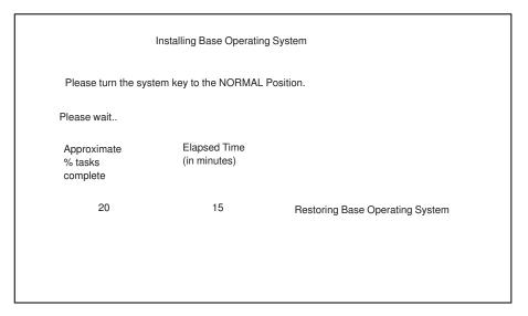
This second screen signals the start of the BOS installation, reporting the rate of completion and duration.
