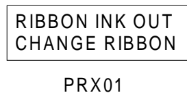
Figure 4-3. Ribbon Fault Display
