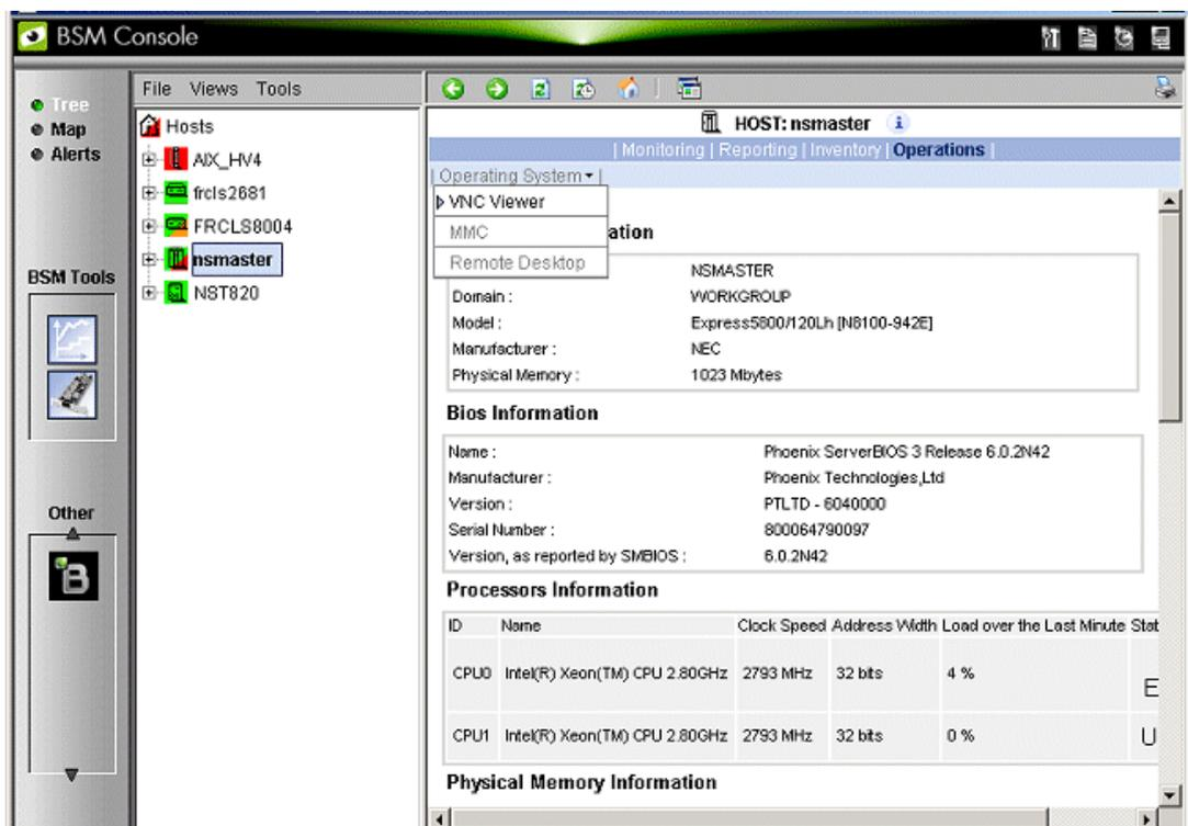
Figure 2-17 Starting UltraVNC Viewer on a Host
