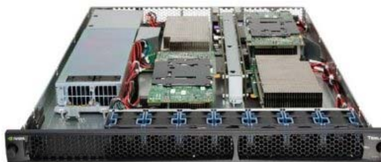
Figure F-7. NVIDIA Tesla S1070 accelerator
