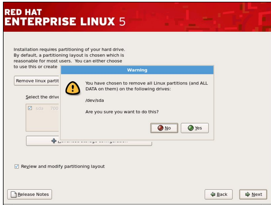
Figure 3-9. Confirmation to remove existing partitions
