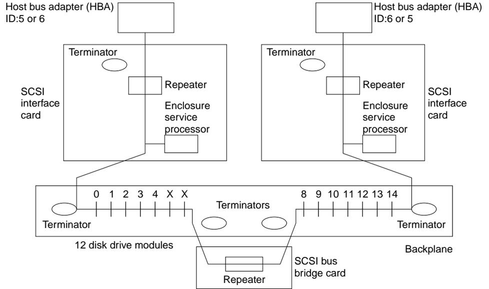
Figure 5. Single Bus, Two Initiators, 12 Disk Drive Modules
