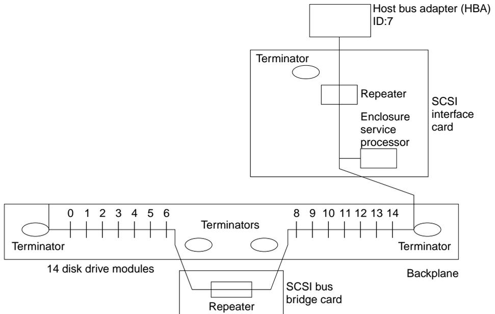
Figure 4. Single Bus, One Initiator, 14 Disk Drive Modules
