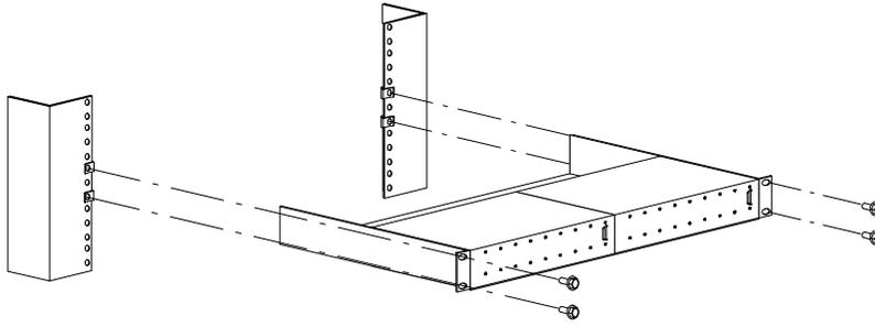
Figure 96. Installation of the FC-AL hub support in the rack
