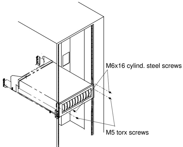
Figure 40. Securing the DAS 5300 to the rack
