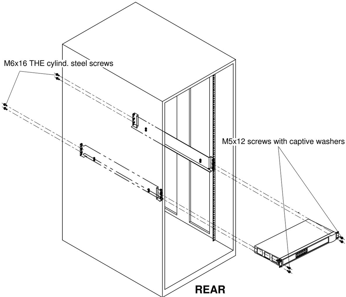
Figure 105. Installing the cluster hub in the rack
