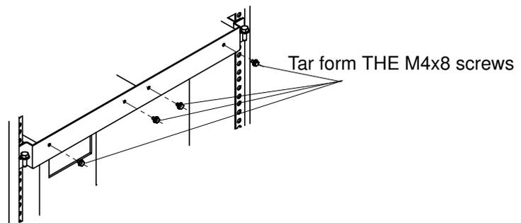
Figure 58. Securing the spacer trays of the two DC SPSs to the support plate at the front of the rack
