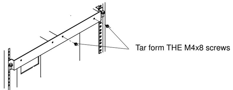
Figure 25. Securing the SPS to the support plate at the front of the rack
