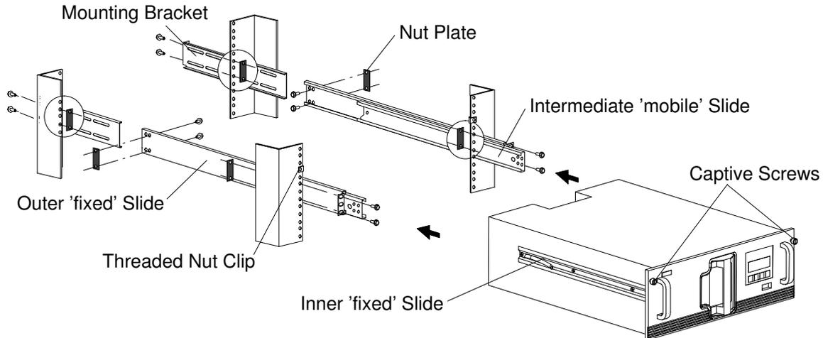
Figure 98. Installation of the Overland library drawer slides
