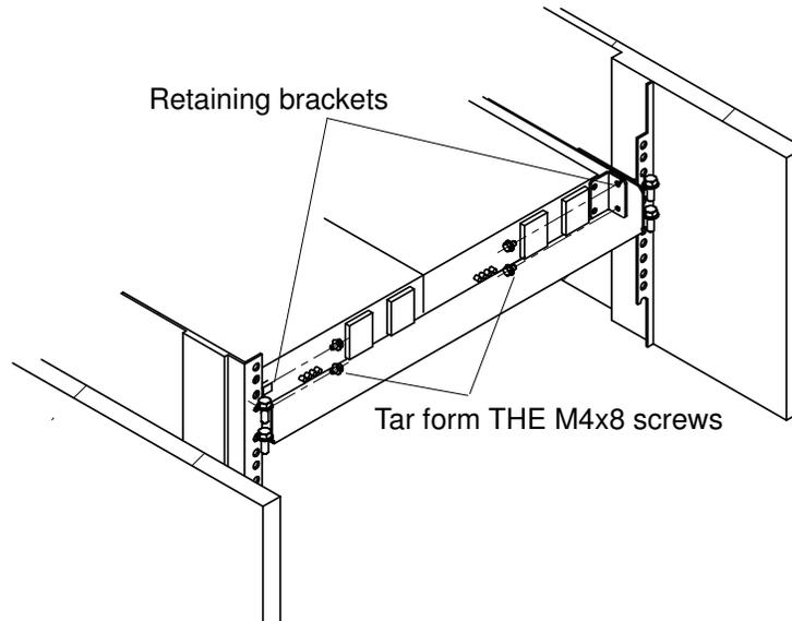
Figure 27. Position of the side retaining brackets of the SPS
