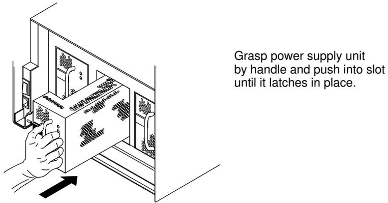
Figure 83. Replacing DAS 3x00 power supplies into the drawer
