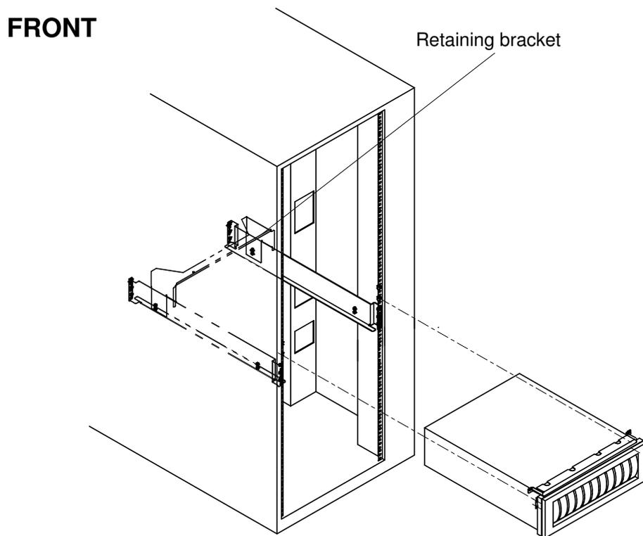
Figure 39. Positioning the DAS 5300 in the rack
