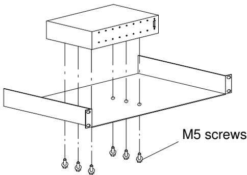
Figure 94. Installation of one FC-AL hub on the support
