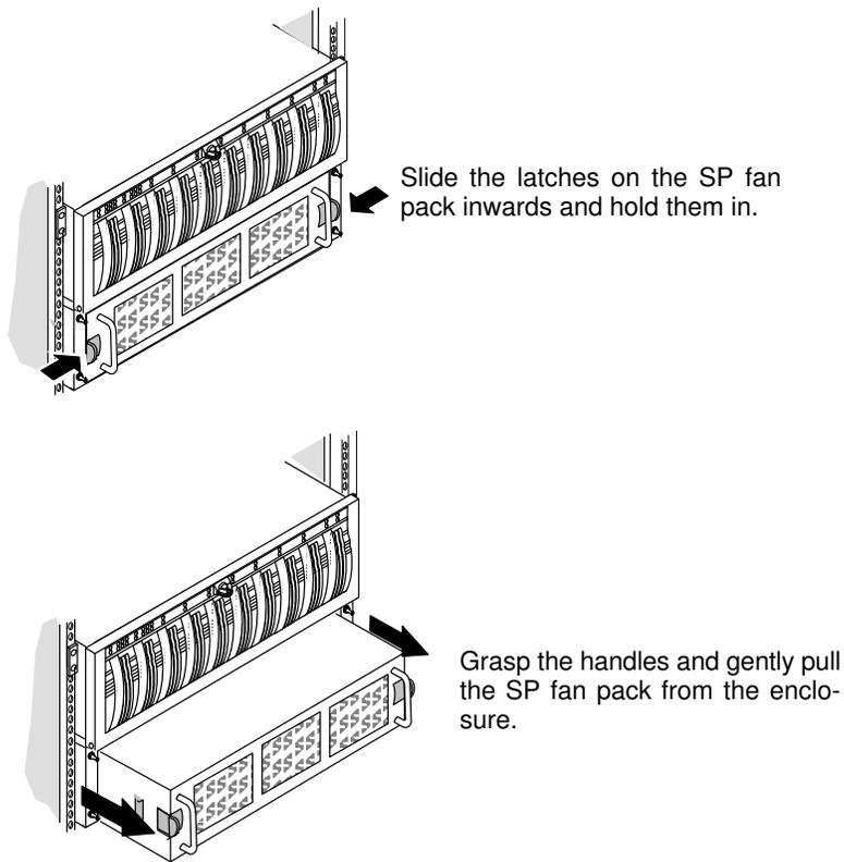
Figure 5. Removing the SP fan pack from the DAS 5700/4500 drawer
