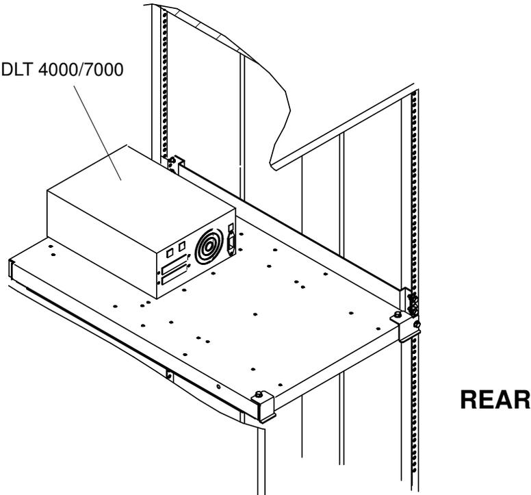
Figure 100. Position of the DLT 4000/7000 on the support plate.
