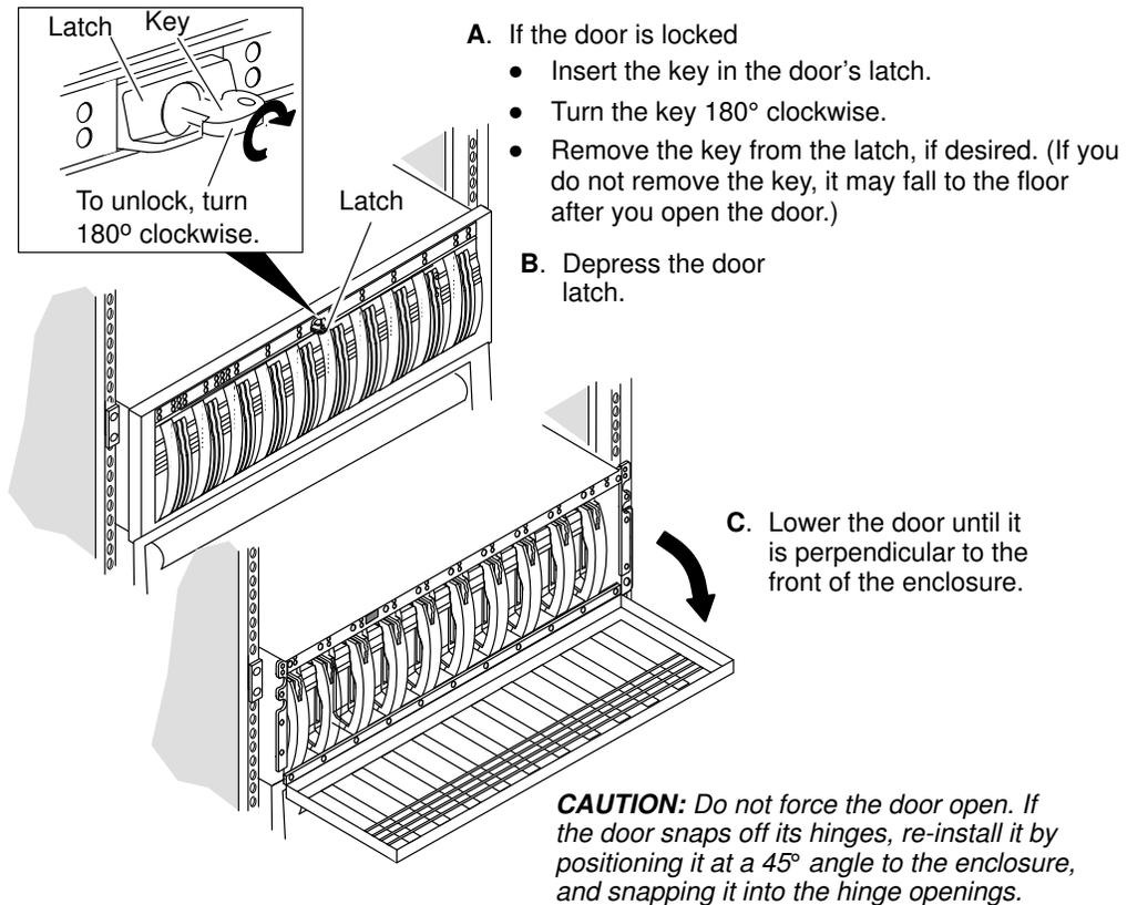
Figure 2. Opening the front door of the DAS 5700/4500
