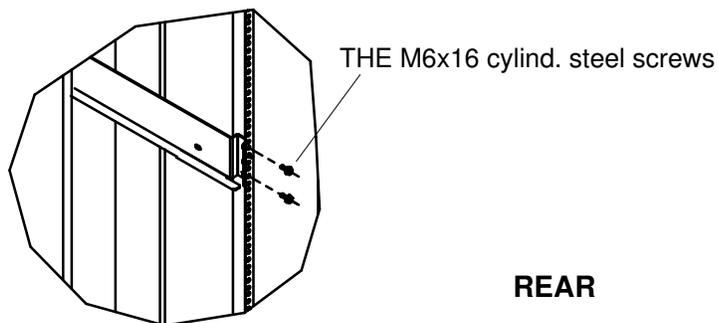
Figure 111. Securing the rails of the Fibre Channel switch at the rear of the rack
