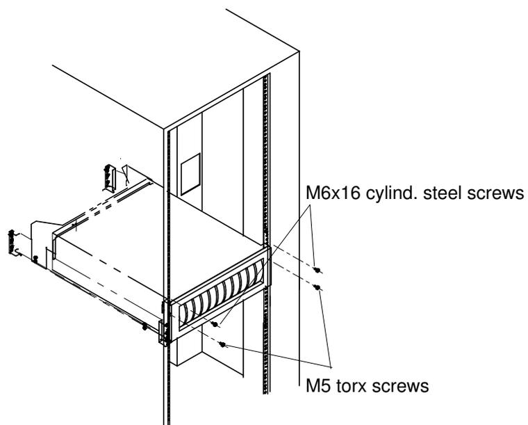
Figure 68. Securing the DAE5000 to the rack
