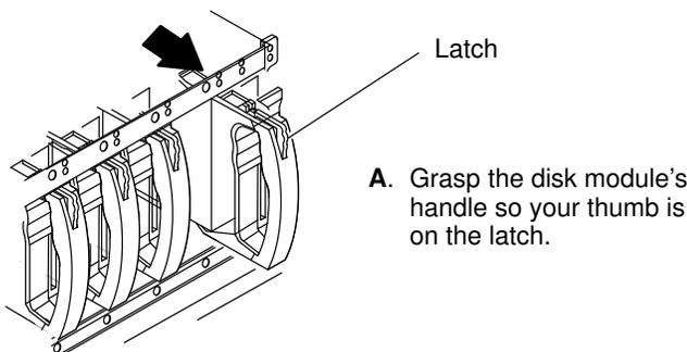
Figure 61. Removing DAE5000 disk modules from the drawer
