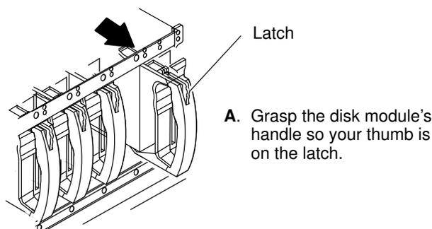
Figure 3. Removing DAS 5700/4500 disk modules from the drawer
