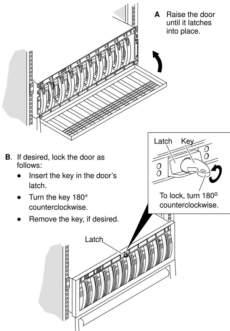
Figure 47. Replacing the front door of the DAS 5300 drawer
