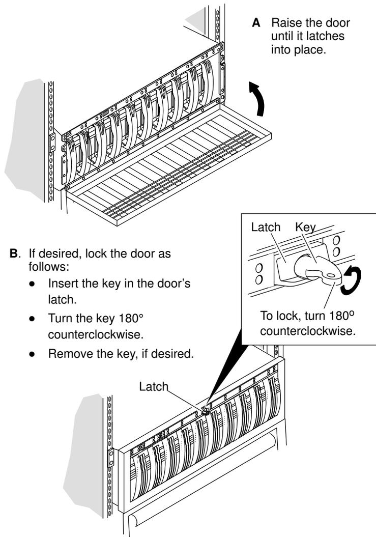
Figure 19. Replacing the front door of the DAS 5700/4500 drawer
