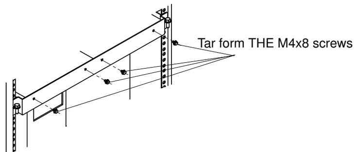
Figure 29. Securing the SPSs to the support plate at the front of the rack
