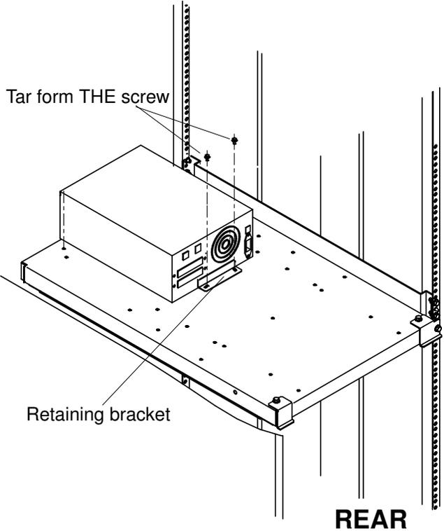
Figure 101. Position of the DLT 4000/7000 retaining bracket.
