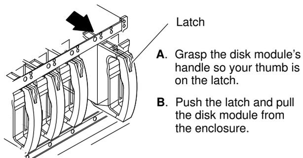
Figure 32. Removing DAS 5300 disk modules from the drawer
