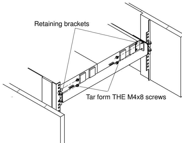
Figure 56. Position of the side retaining brackets of the DC SPS
