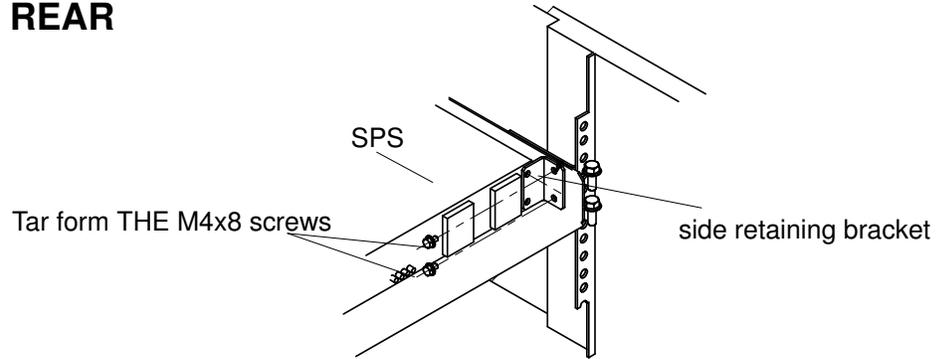
Figure 23. Fixing the side retaining bracket of the SPS to the rack
