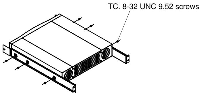
Figure 110. Fixing the side attachment brackets to the Fibre Channel switch
