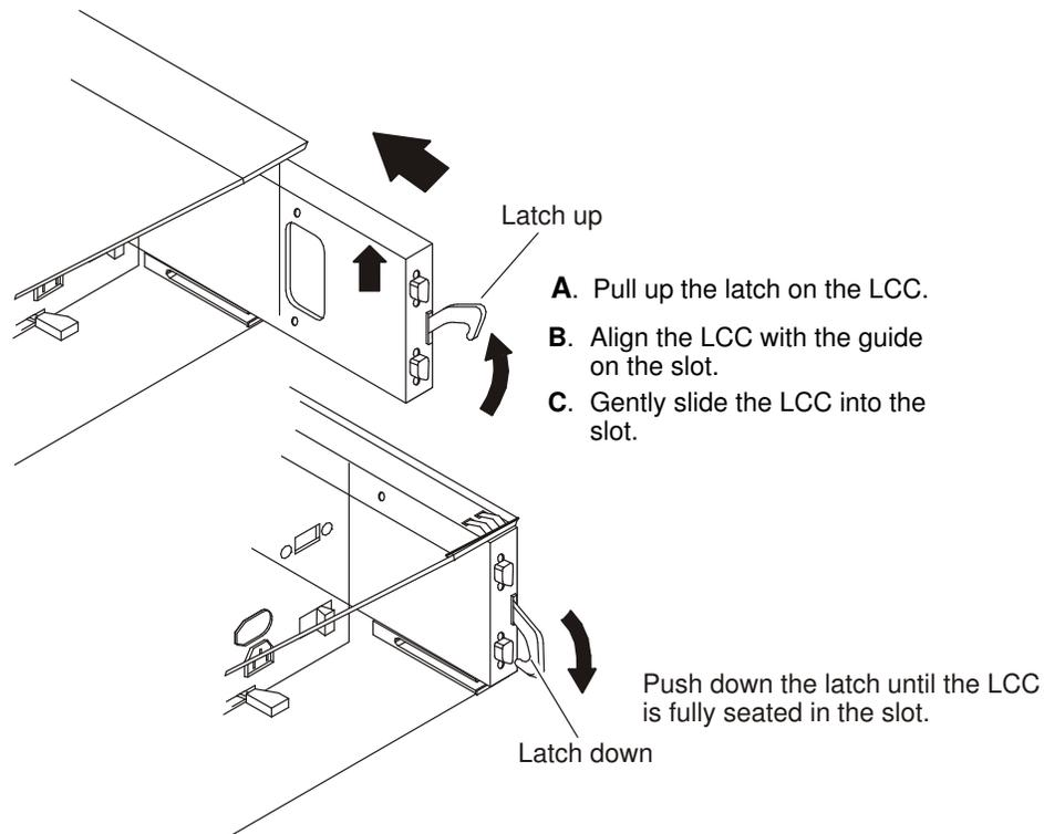
Figure 45. Replacing storage processors (SP) from the DAS 5300
