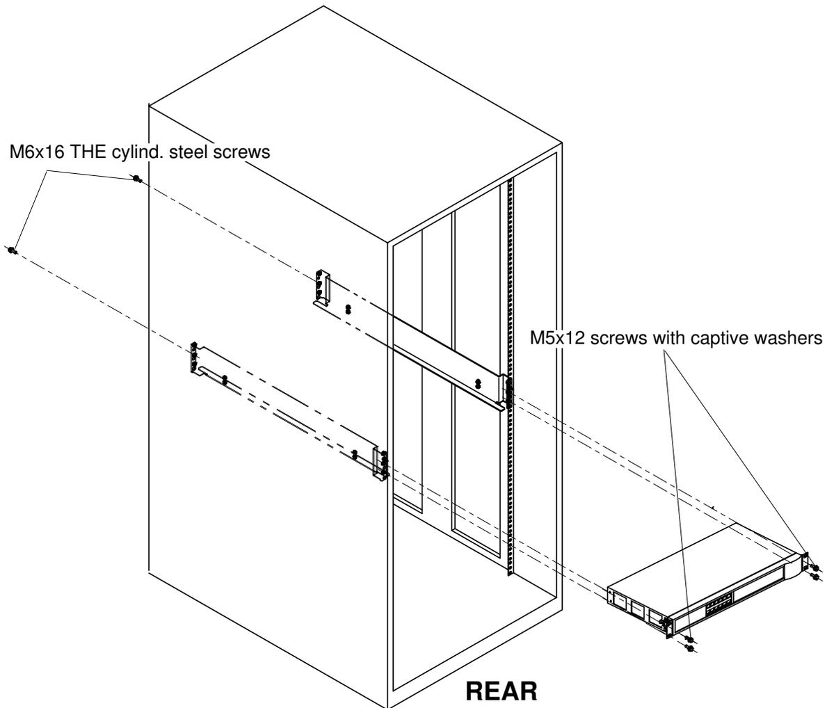
Figure 107. Installing the cluster hub in the rack
