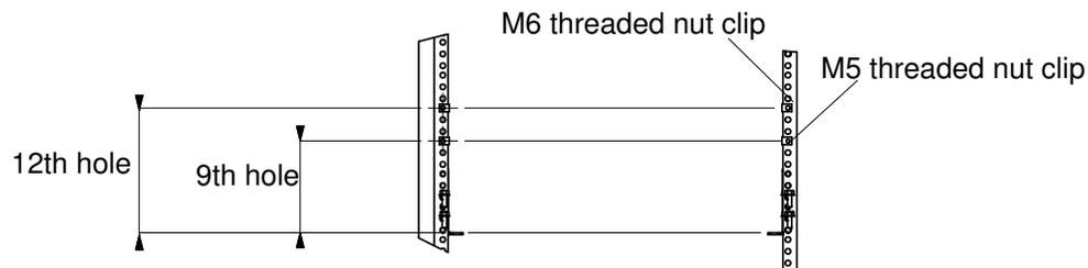
Figure 65. Positioning threaded nut clips needed to fix the DAE5000 to the rack
