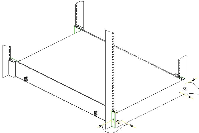
Figure 118. Fixing the ground braids
