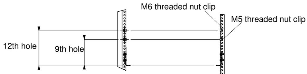
Figure 37. Positioning threaded nut clips needed to fix the DAS 5300 to the rack
