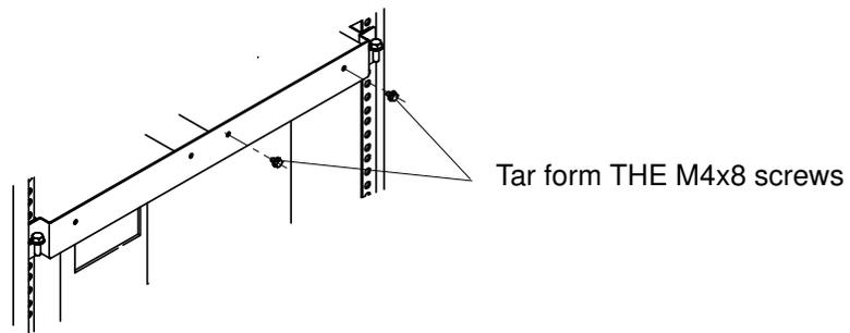
Figure 54. Securing the spacer tray of the DC SPS to the support plate at the front of the rack
