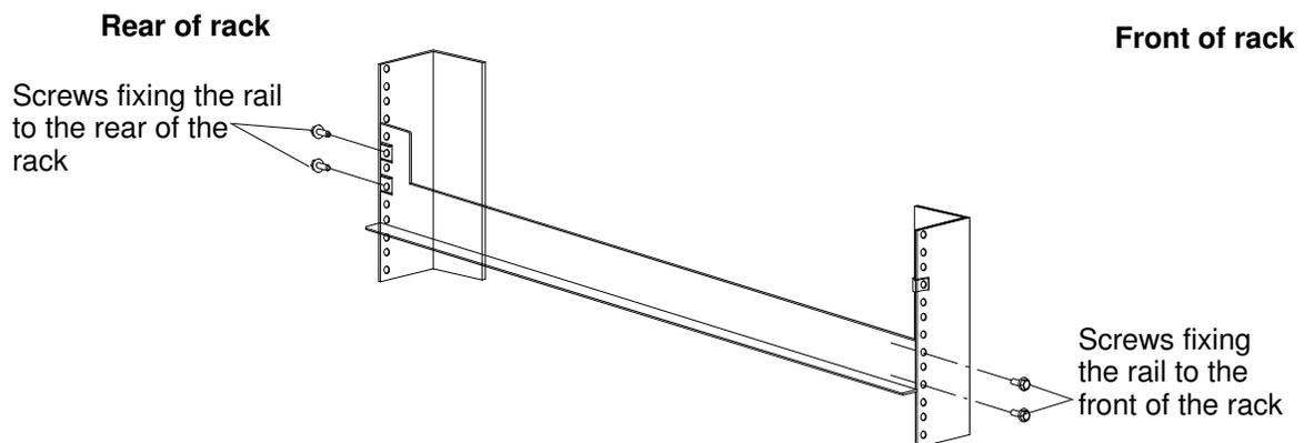
Figure 89. Position of one of the DAS 2900 rails in the rack
