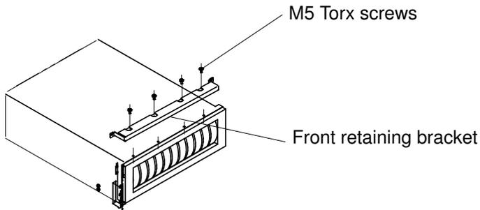
Figure 38. Securing the front retaining bracket to the DAS 5300
