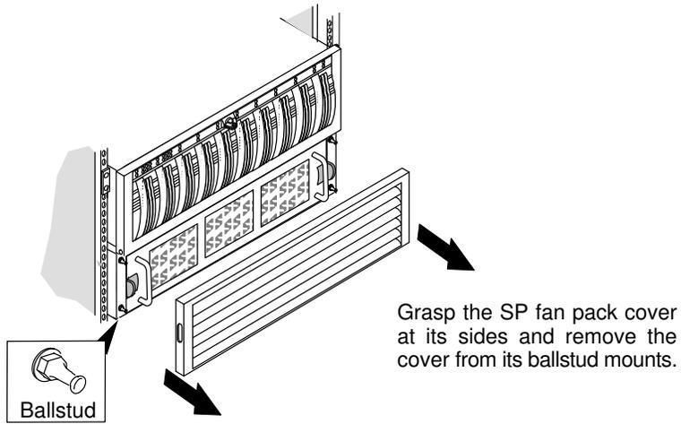
Figure 4. Removing the SP fan pack cover of the DAS 5700/4500
