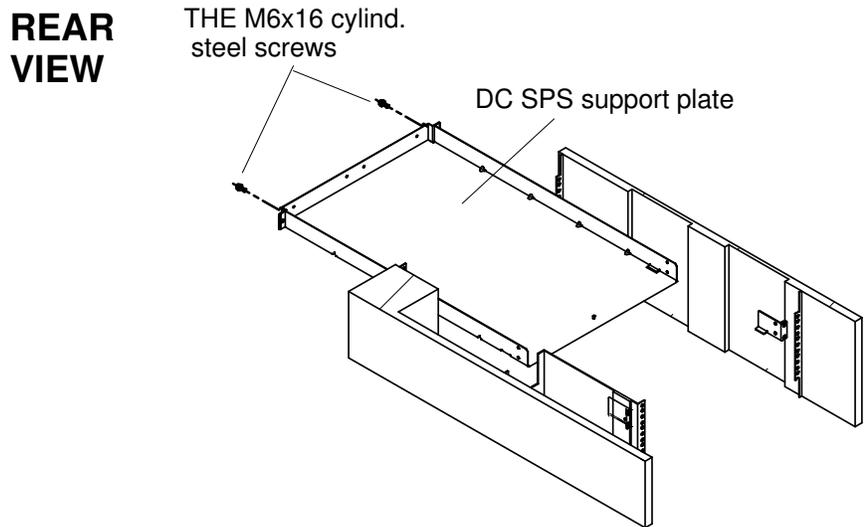
Figure 49. Positioning the DC SPS support plate
