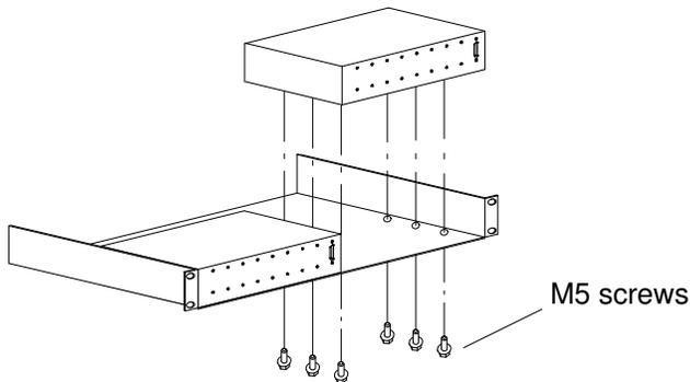
Figure 95. Installation of two FC-AL hubs on the support
