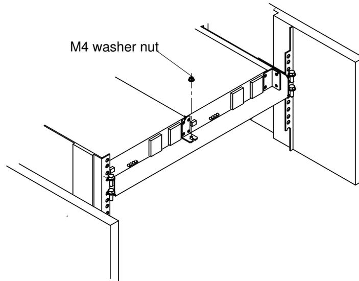
Figure 59. Fixing the M4 washer nut to the support plate of the DC SPS
