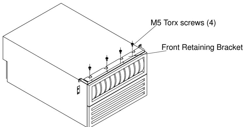
Figure 10. Position of the front retaining on the DAS 5700/4500
