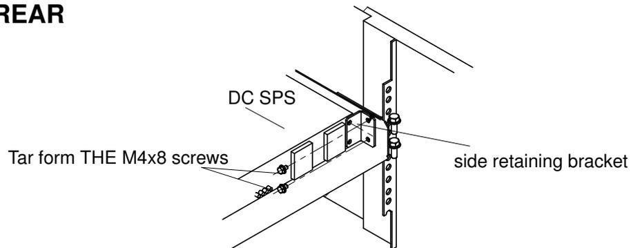
Figure 52. Fixing the side retaining bracket of the DC SPS to the rack
