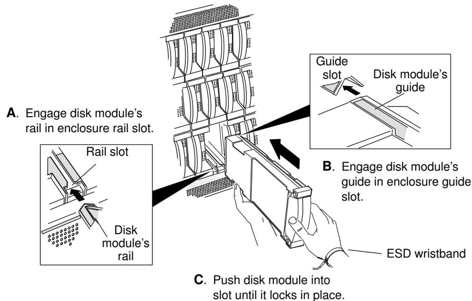
Figure 81. Replacing DAS 3x00 disks into the drawer
