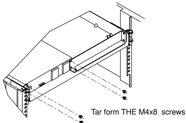
Figure 53. Securing the DC SPS to the side retaining bracket and to the filler panel
