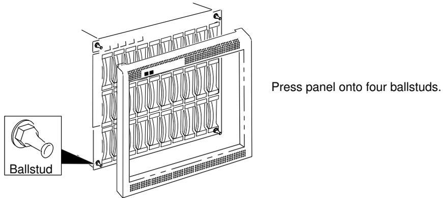
Figure 82. Replacing DAS 3x00 front panel
