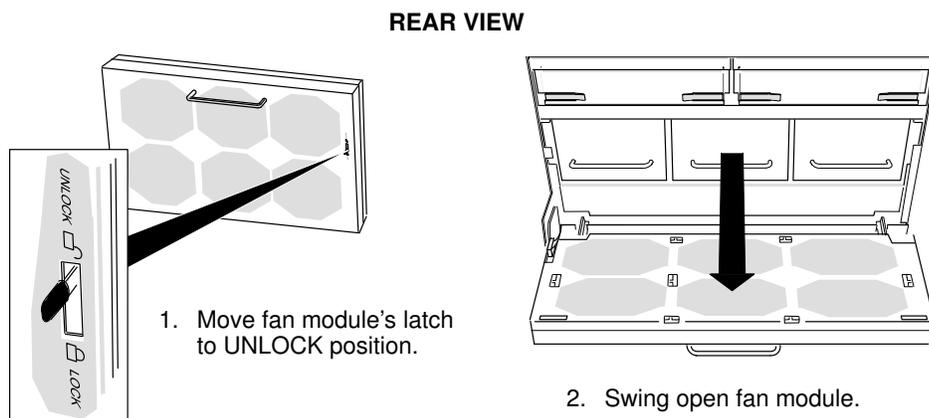
Figure 84. Opening the fan module of the DAS 2900
