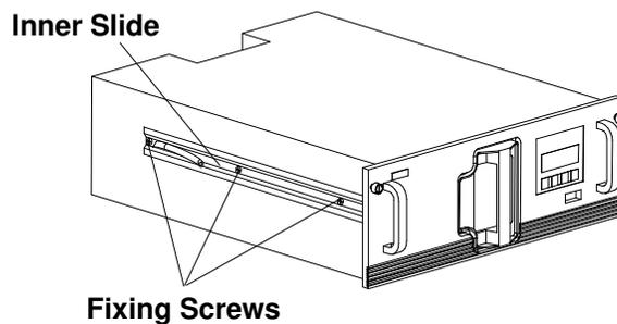
Figure 97. Overland drawer with inner slides mounted
