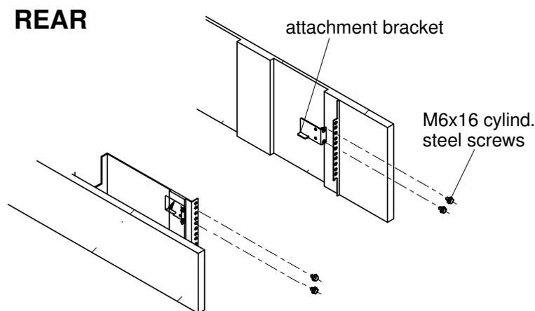
Figure 20. Positioning the attachment brackets of the SPS support plate
