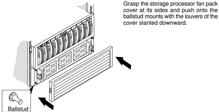
Figure 18. Replacing the storage processor fan pack cover on the DAS 5700/4500 drawer
