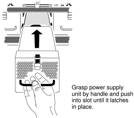
Figure 93. Replacing the DAS 2900 power supplies into the drawer
