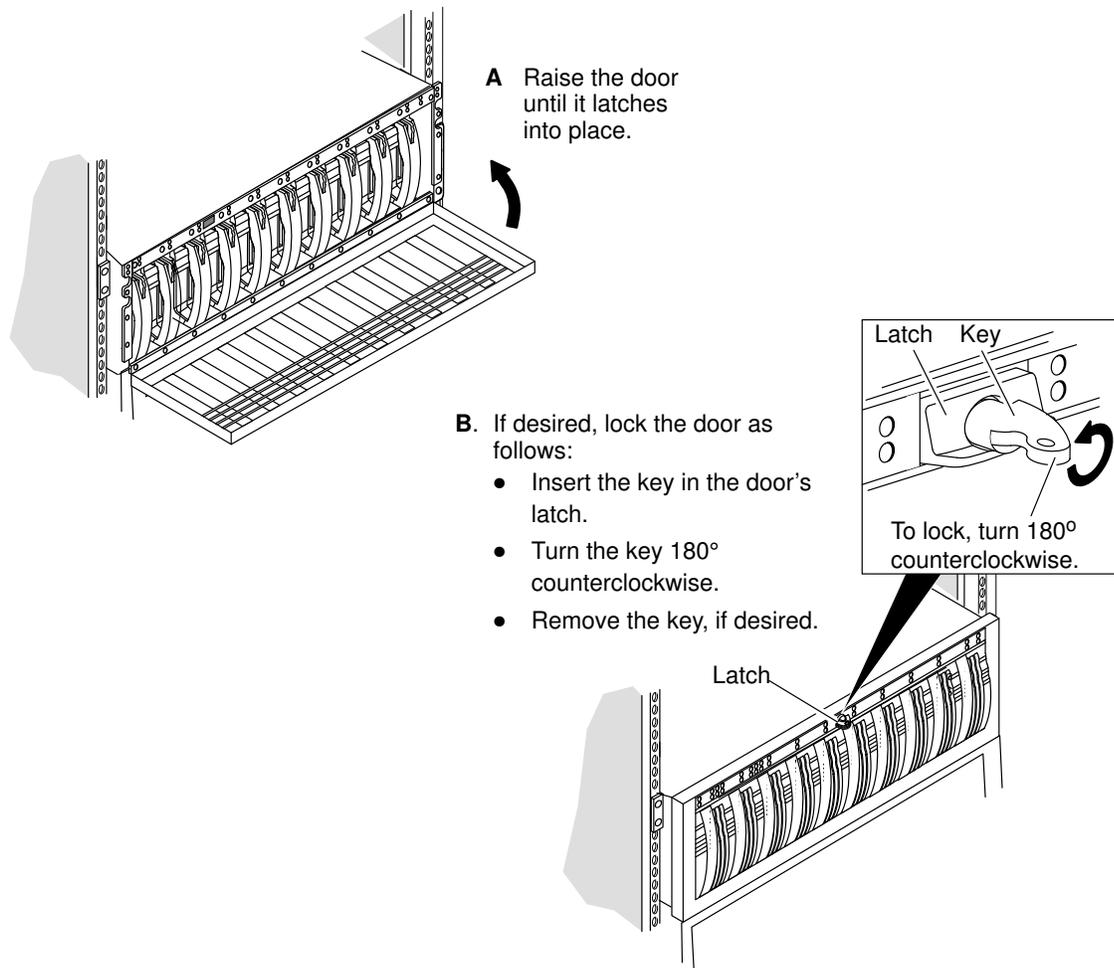
Figure 74. Closing the front door of the DAE5000
