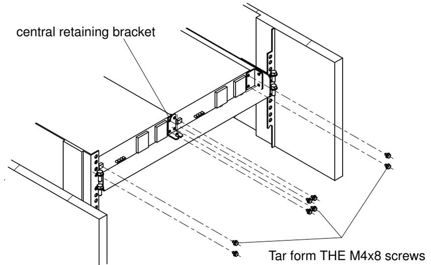
Figure 57. Securing the two DC SPSs to the side and central retaining brackets
