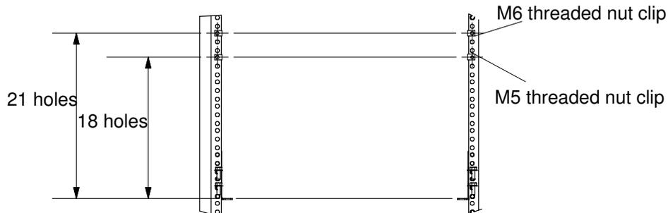
Figure 9. Position of the threaded nut clips at the front of the rack for a DAS 5700/4500
