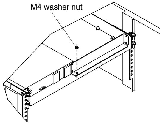
Figure 26. Fixing the M4 washer nut to the support plate of the SPS
