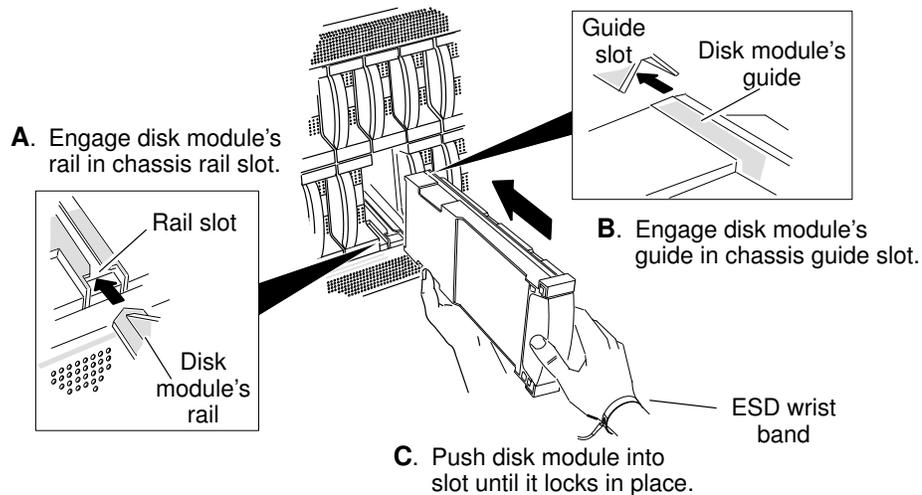
Figure 91. Replacing DAS 2900 disks into the drawer
