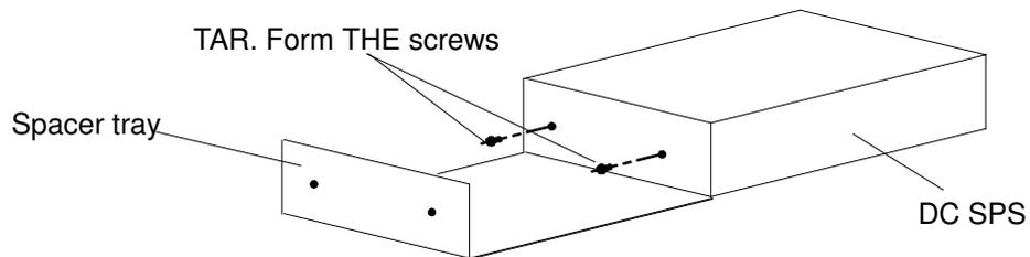
Figure 50. Positioning the spacer to the DC SPS
