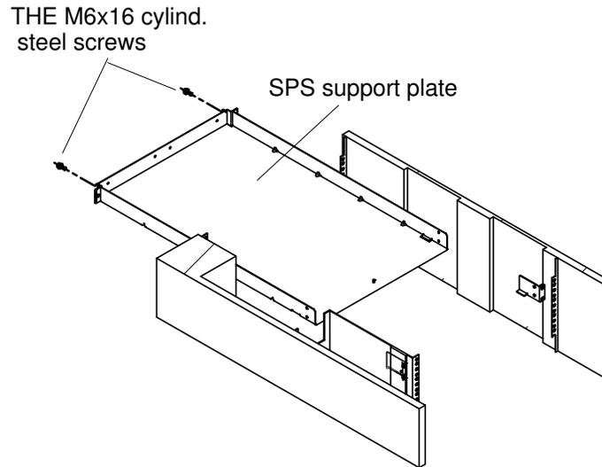
Figure 21. Positioning the SPS support plate
