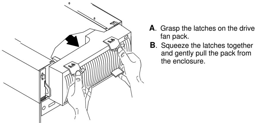
Figure 34. Removing the drive fan pack from the DAS 5300 drawer
