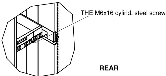
Figure 113. Securing the Fibre Channel switch at the rear of the rack
