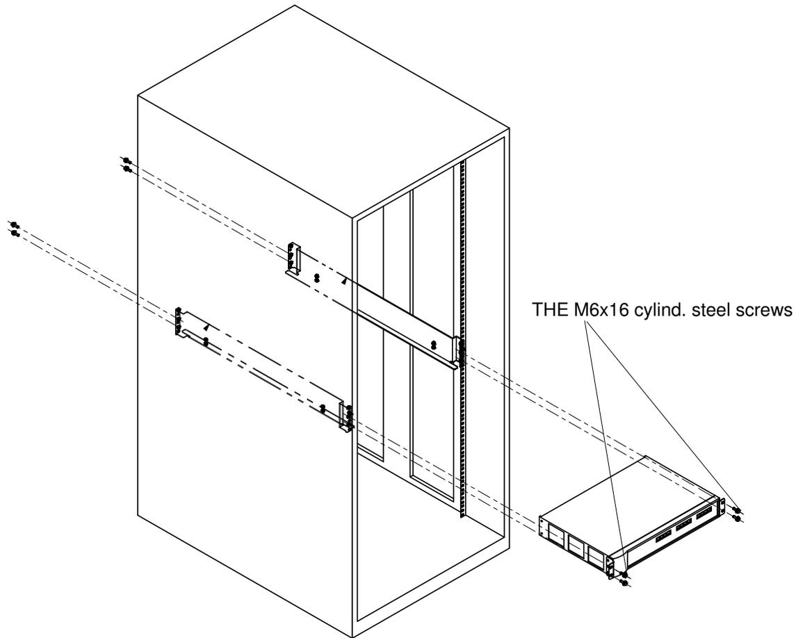
Figure 109. Installing the Ethernet switch inside the rack
