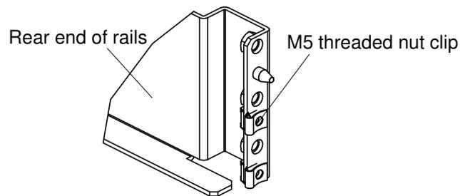
Figure 106. Position of the threaded nut clips on the rails for the cluster hub
