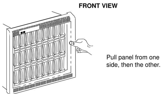
Figure 77. Removing the DAS 3x00 front panel
