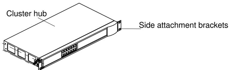
Figure 103. Position of the side attachment brackets on the cluster hub
