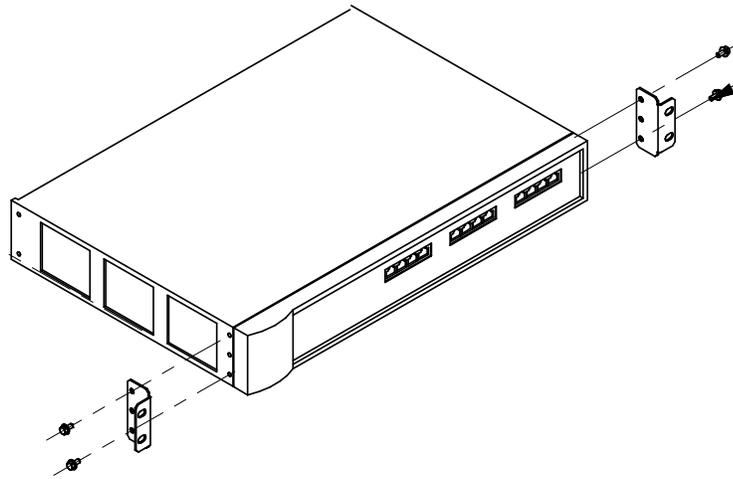
Figure 108. Fixing the side attachment brackets to the Ethernet switch
