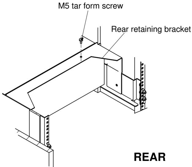
Figure 69. Securing the rear retaining bracket to the DAE5000
