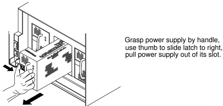
Figure 76. Removing DAS 3x00 power supplies from the drawer
