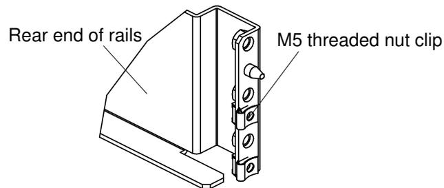
Figure 104. Positioning nut clips on the cluster hub rails
