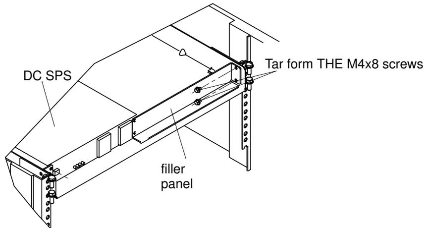
Figure 51. Position of the DC SPS filler panel
