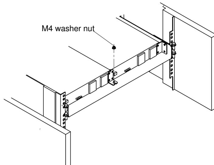
Figure 30. Fixing the M4 washer nut to the support plate of the SPS
