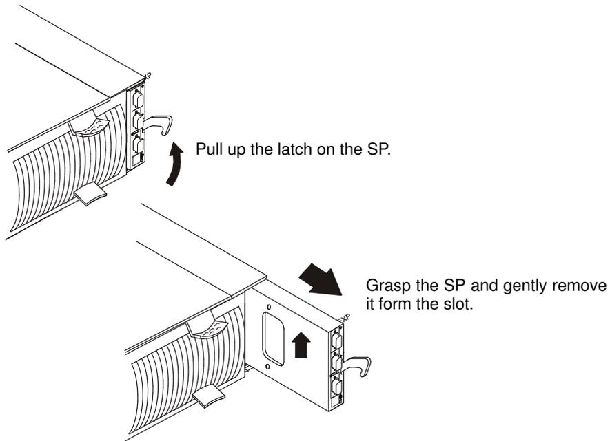
Figure 33. Removing storage processors (SP) from the DAS 5300
