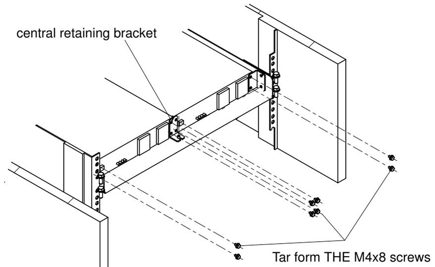
Figure 28. Securing the two SPSs to the side and central retaining brackets
