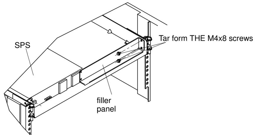
Figure 22. Position of the SPS filler panel
