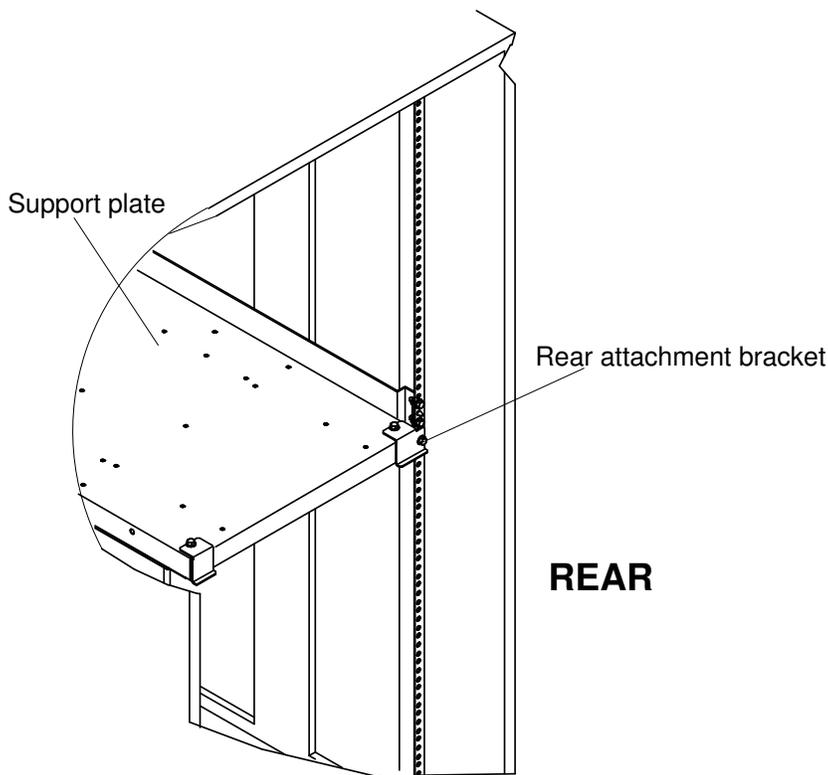
Figure 99. Rear attachment bracket of the support plate
