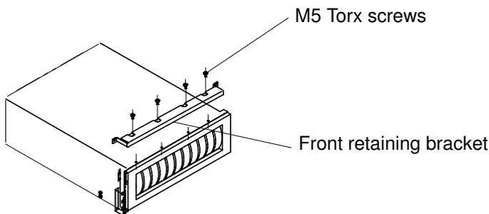
Figure 66. Securing the front retaining bracket to the DAE5000
