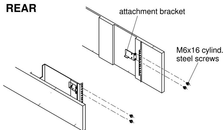
Figure 48. Positioning the attachment brackets of the DC SPS support plate
