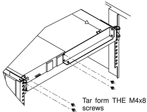
Figure 24. Securing the SPS to the side retaining bracket and to the filler panel
