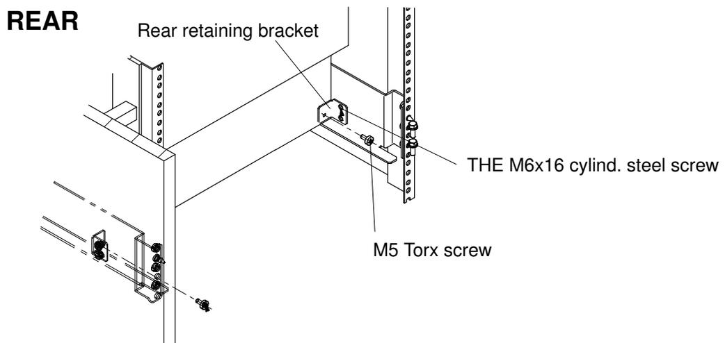
Figure 12. Securing the DAS 5700/4500 at the rear of the rack
