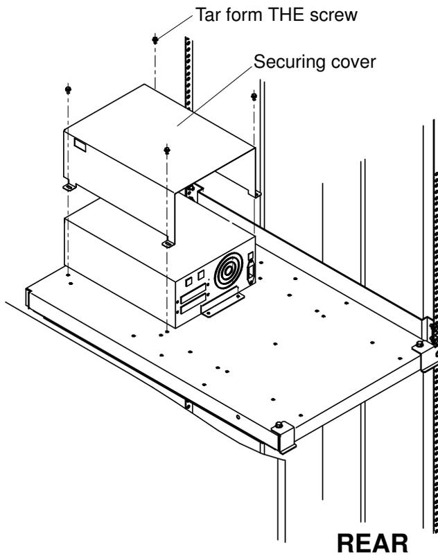
Figure 102. Positioning the securing cover on the DLT 4000/7000
