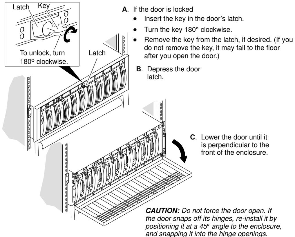
Figure 31. Opening the front door of the DAS 5300
