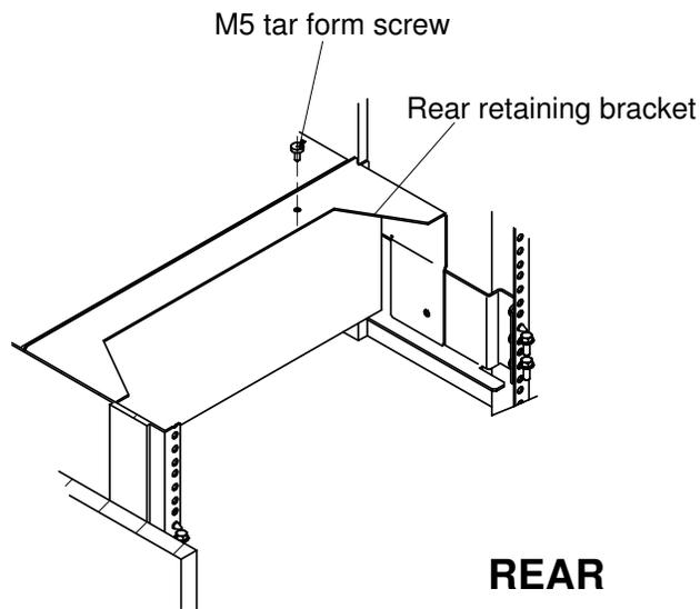
Figure 41. Securing the rear retaining bracket to the DAS 5300
