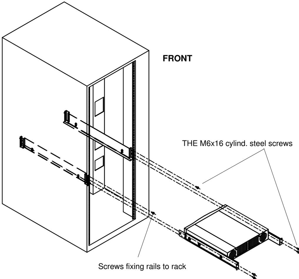
Figure 112. Installing the Fibre Channel switch inside the rack
