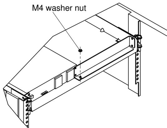
Figure 55. Fixing the M4 washer nut to the support plate of the DC SPS
