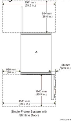
Figure 2. Service clearances for single-frame systems with slimline doors (with alternative right-side service clearance)
