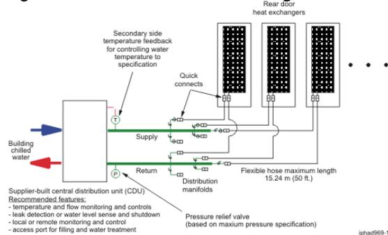
The following figure shows a typical cooling solution and defines the components of the primary cooling loop and the components of the secondary cooling loop.
