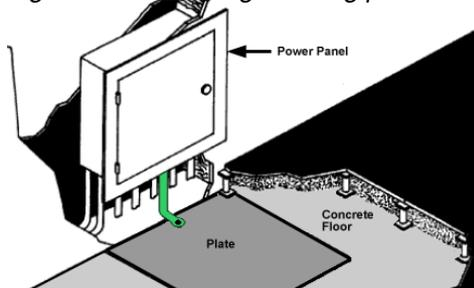
The preferred connection is with a braided strap. If a braided strap is not available, the connection should consist of no. 12 AWG (3.3 mm or 0.0051 in.) or larger conductor and should not be more than 1.5 m (5 ft.) long. To minimize this length, the preferred connection of this braided strap or conductor is to the nearest portion of the enclosure on the panel, if the enclosure is electrically continuous from the green-conductor common point to this point of connection.
