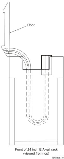
Lay hoses side-by-side as they run between the heat exchanger and the supply and return manifolds, and allow the hoses to freely move. Leave enough slack in the hoses below the rear door so that minimum forces are exerted on the door when the hoses are attached and operating. When routing hoses, avoid sharp bends that cause hose kinks, and avoid hose contact with sharp edges.
