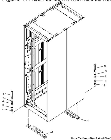
2. Place the mounting plates (item 1 in Figure 1), front and back, in the approximate mounting position under the system rack.
