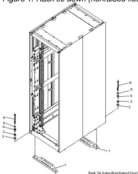
2. Place the mounting plates (item 1 in Figure 1), front and rear, in the approximate mounting position under the system rack.
