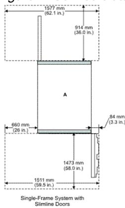
Figure 2. Service clearances f/75 single frame systems with slimline doors (with alternative right-side service clearance)
