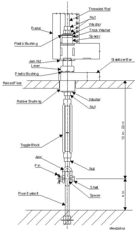
Figure 7. Turnbuckle assembly frame tie down hardware for 304.8 mm to 558.8 mm (12 in. to 22 in.) raised floor (Part number 44P3000)
