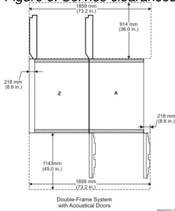
Refer to the figure in [Raised-floor requirements and preparation](#) for service clearances shown in a raised-floor installation.
