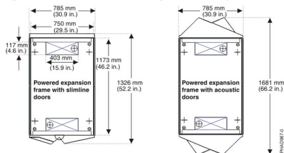
*Figure 2. Plan view for double-frame systems with slimline doors and acoustical doors*
