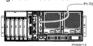
Figure 4. Model ESCALA PL 6450R and 91/94 base PCI-X expansion tower rear view with J14 connection
