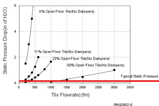
Floor tiles in typical data centers deliver between 100 and 300 cfm. By optimizing the flow utilizing some of the guidelines set forth in this document, it may be possible to realize flows as high as 500 cfm. Flow rates as high as 700-800 cfm per tile are possible with tiles with the highest percent-open rating. Floor tiles must be aligned in the cold aisles with the intake locations on the equipment.
