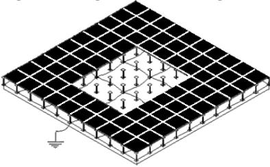
Stranded bare or insulated conductor of at least no. 8 AWG (8 mm or 0.0124 in.) copper is required. This conductor provides a low-impedance path and is strong enough to make physical damage unlikely. Any connection method is acceptable as long as it provides a reliable electrical and mechanical connection.
