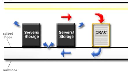
A higher return air temperature can be tolerated in underfloor air distribution without affecting the design conditions of the overall room. The underfloor design takes into consideration a heat transfer factor through the raised metal floor and also provides some reheated air to control the relative humidity before it enters the room.
