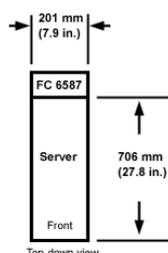
The feature code 6587 is a decorative rear cover that has sound-deadening capability. This cover is for servers that do not have external I/O attached to a high speed link (HSL) loop. The cover cannot be used if HSL cables are attached to the server.
