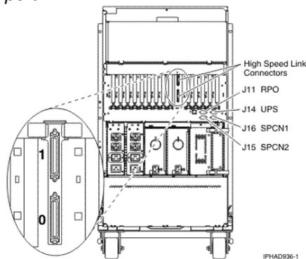
**Note:** The 8-way, 12-way, and 16-way processor configurations for the model ESCALA PL 850R/PL 1650R/R+ consists of several 4-way processors connected together. The uninterruptible power supply converter cable must be connected to the 4-way drawer that has the operator's panel on the front of the unit.
