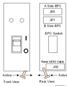
The preceding figure illustrates the back of the machine UEPO panel with the room EPO cable plugging into the machine. Notice the switch actuator. After it is moved to make the cable connection possible, the room EPO cable must be installed for the machine to power on.
