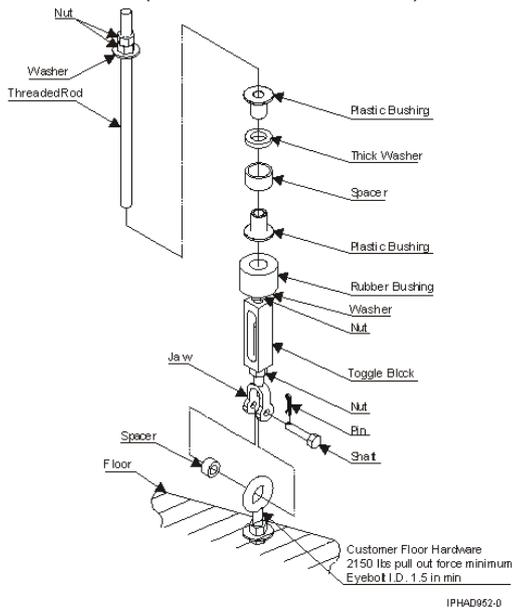
Figure 6. Turnbuckle assembly frame tie down hardware for 304.8 mm to 558.8 mm (12 in. to 22 in.) raised floor (Part number 44P3000)
