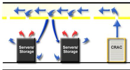
To maximize the cooling capability of such an arrangement, it is imperative to align the supply discharges with the cold aisles and the return grilles with the hot aisles. The supply discharges should force air directly down into the cold aisles and not use diffusers that distribute air laterally. Such diffusion can cause cool air to migrate undesirably into the return air path prior to having the opportunity to transfer heat from the equipment.
