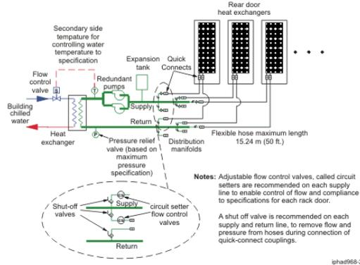
The following figure shows an example of an off-the-shelf modular cooling distribution unit. The actual number of rear door heat exchangers connected to a secondary loop depends on the capacity of the cooling distribution unit that is running the secondary loop.
