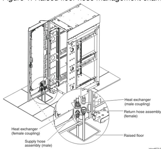
Figure 2. Raised floor hose management example 1; tile cut out size and position for 24-inch EIA-rail racks.
