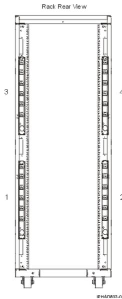
Power distribution units (PDUs) are required with 7014 racks. If a PDU is not defaulted or ordered, a power cord is provided with each individual rack-mounted drawer for connection to a country-specific utility mains receptacle or uninterruptible power supply. See the individual rack-mounted drawer specifications for the appropriate power cords. The following PDU is available for the 7014 racks:
