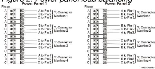
The following figure shows another way of distributing the unbalanced load evenly. In this case, the three-pole breakers are alternated with two-pole breakers.
