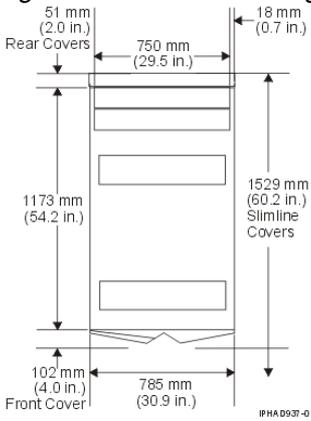
**Attention:** When moving the rack, note the caster swivel diameters shown in the following figure. Each caster swivels in an approximate 130 mm (5.1 inch) diameter.
