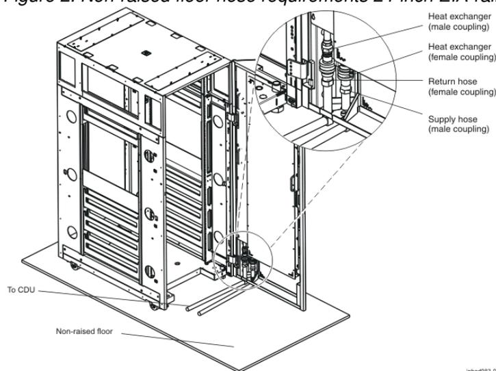
Hoses exiting the heat exchanger can be routed in a manner similar to that of power cables in a non-raised floor data center. For example, place the hoses side-by-side and allow them to move freely as they approach the rack (within approximately 3 m (10 ft.) of the rack). When the door is opened, it is acceptable for the hoses to move slightly and rotate in parallel at the coupling interface inside the door. As the door is closed, the hoses rotate back to their original positions.
