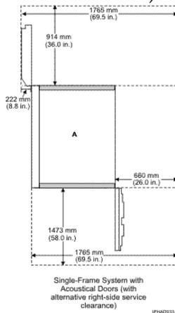
Front service access is necessary on the model 185/75 to accommodate a lift tool for the servicing of large drawers (the processor books and I/O drawers). Front and rear service access is necessary to accommodate the lift tool for servicing of the optional integrated battery backup.
