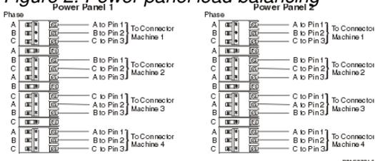
The following figure shows another way of distributing the unbalanced load evenly. In this case, the three-pole breakers are alternated with two-pole breakers.
