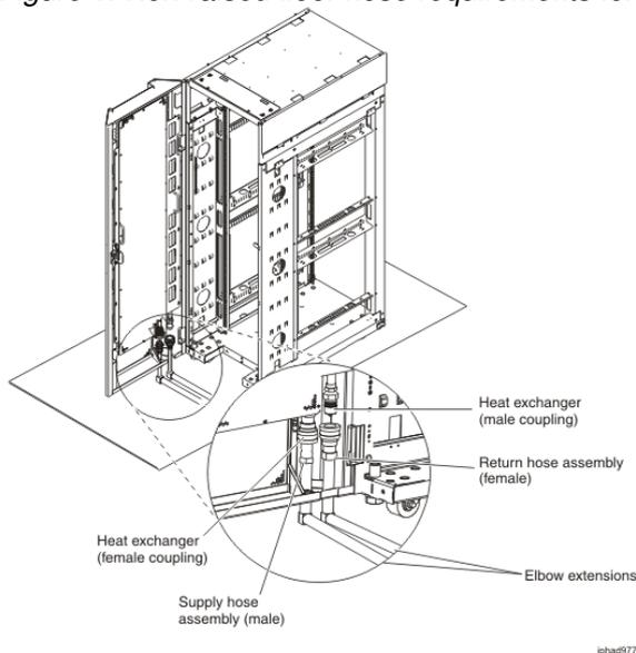
Figure 2. Non-raised floor hose requirements 24-inch EIA-rail rack
