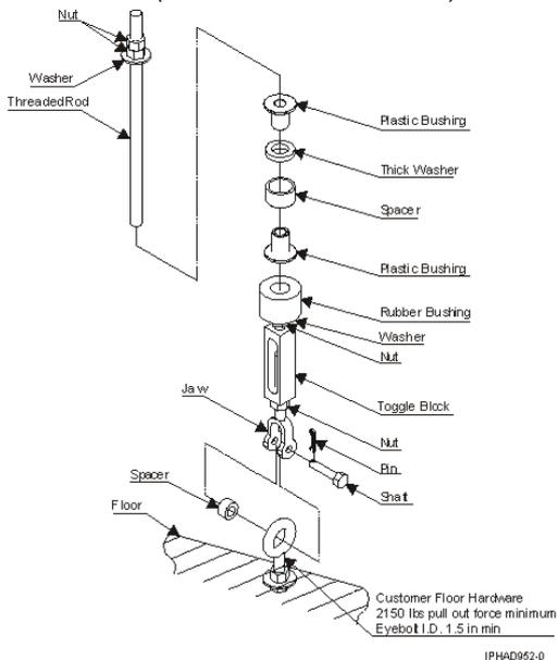
Figure 6. Turnbuckle assembly frame tie down hardware for 304.8 mm to 558.8 mm (12 in. to 22 in.) raised floor (Part number 44P3000)
