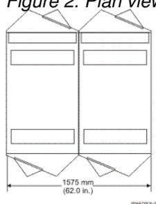
**Attention:** When moving the rack, note the caster swivel diameters shown in the following figure. Each caster swivels in an approximate 130 mm (5.1 inch) diameter.
