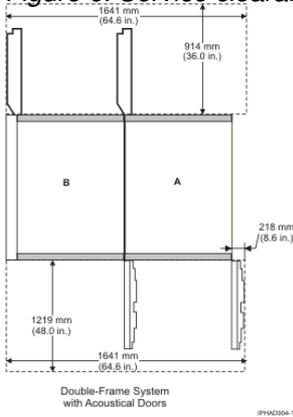
Refer to the figure in [Raised-floor requirements and preparation](#) for service clearances shown in a raised-floor installation.
