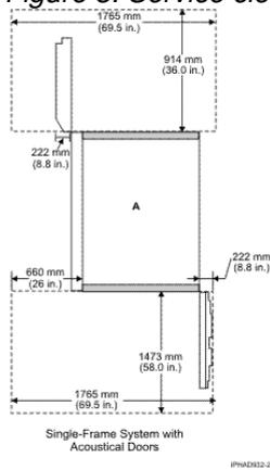
Figure 4. Service clearances f/75 single-frame systems with acoustical doors (with alternative right-side service clearance)
