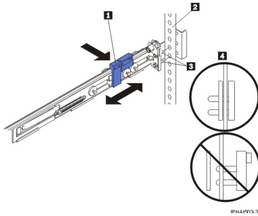
**Attention:** Ensure that the pins 3 are fully extended through the mounting flange and the slide rail 4.
