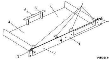
2. Position the modem in the tray 4 or 7 with the front of the modem facing the front of the tray. Slide the front of the modem under the two retainer tabs 8.
