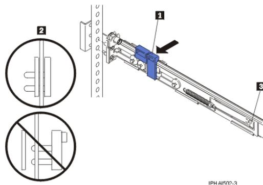
If you need to adjust the slide-rail length, lift the tab 3 and extend the rail-adjustment bracket from the back of the slide rail until it is the appropriate length.
