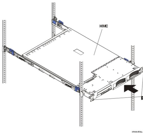
8. If the shipping brackets impede the HMC from fully setting into the rack enclosure, remove the shipping brackets by pressing on the tab 1 as indicated on the shipping bracket, and slide the shipping bracket off the slide rail. Repeat this step for the other shipping bracket. Store the shipping bracket for future use. The following figure shows a side view of the side rail and the shipping bracket tab:
