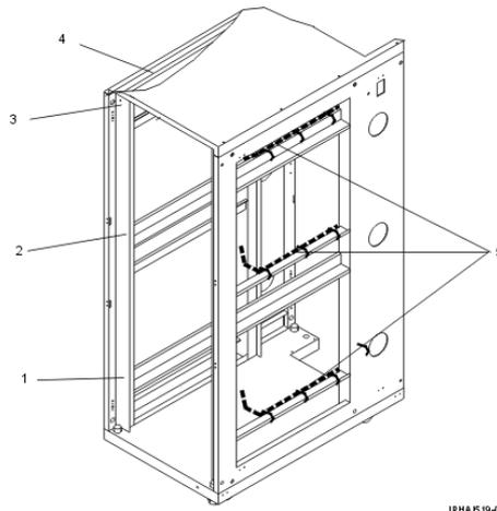
11. Secure the power cord and data cables 3 to the horizontal rail using the hook-and-loop cable ties 2. The modem is indicated by 1 and the cable clamps are indicated by 4. For more detail, see the following illustration:
