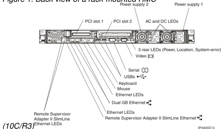
Figure 2. Back view of a rack-mounted HMC
