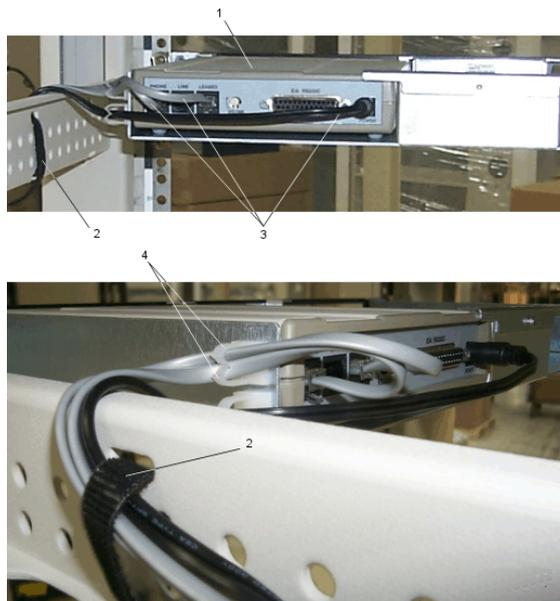
**Note:** Before securing the cables and cord, ensure that the connector on each cable or cord is accessible to its destination (such as the data cable reaching the HMC and the power cord from the power supply reaching the PDB).
