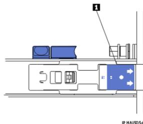
**Note:** You must reinstall the shipping brackets on the slide rails before you transport the rack enclosure to another location with the HMC installed. To reinstall the shipping bracket, reverse this step.
