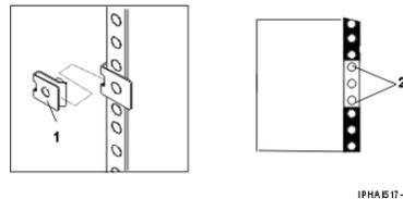
4. Position the modem tray at the selected installation location, and slide the modem tray into the rack. Ensure that the mounting screw holes on the modem tray align with the nut clips installed on the rack front vertical rails.
