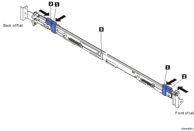
3. Position the rail so that the pins on the back rail-locking carrier align with the holes on the back rail-mounting flange. Press the blue tab 1 to release the rail-locking carrier and secure the back of the slide rail onto the back rack-mounting flange.
