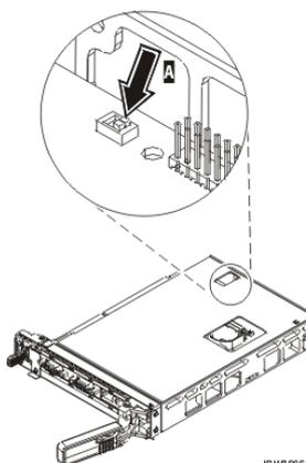
6. Reinsert the service processor into the managed system. See [Replace the model ESCALA PL 850R/PL 1650R/R+ service processor assembly](#).
