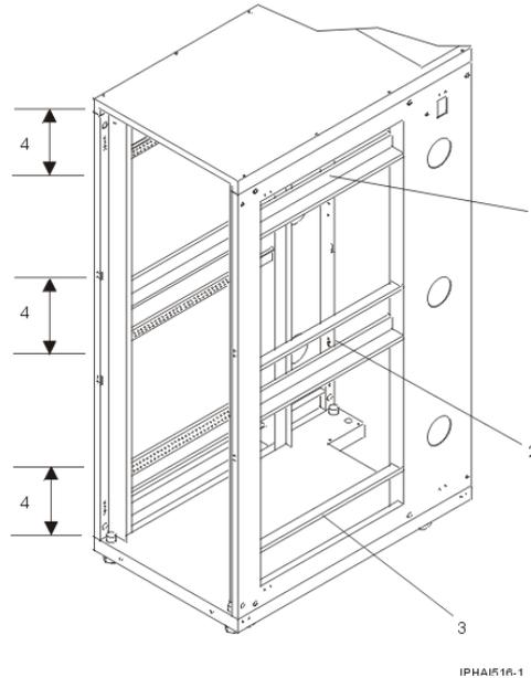
3. Install nut clips 1 on each of the front vertical rails of the rack at the selected EIA installation location 2 as shown in the following illustration.
