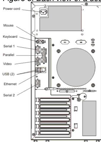
Figure 4. Back view of a stand-alone HMC (10C/04)
