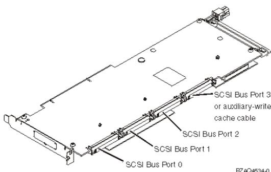
2. Attach the cable to the SCSI port on the auxiliary-write cache adapter.
