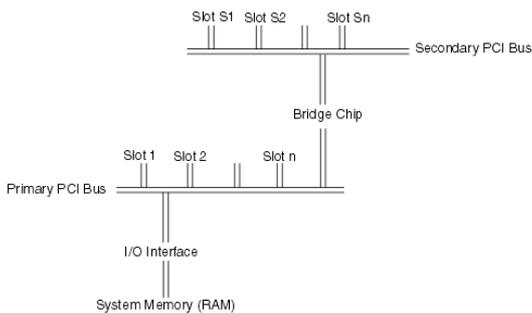
Because the slots on the secondary PCI bus must pass through the bridge chip, certain adapters on a secondary PCI bus might experience lower performance.
