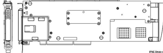
A physical cable connection is required between the 5708 adapter and SCSI port 4 of a 2780 or 2757 adapter. Both the 5708 adapter and the disk-controller adapter it is connected to must be installed in the same physical system unit or expansion unit, and must be installed in the same partition.
