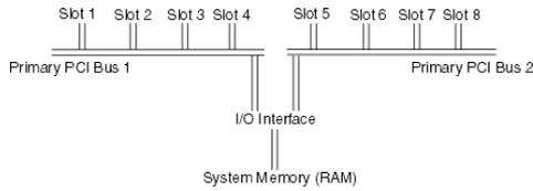
This design can improve I/O performance over the secondary bus method because the I/O interface has created multiple parallel paths into the system memory.
