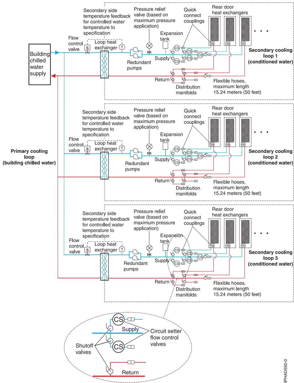
Figure 31. Primary and secondary cooling loops
