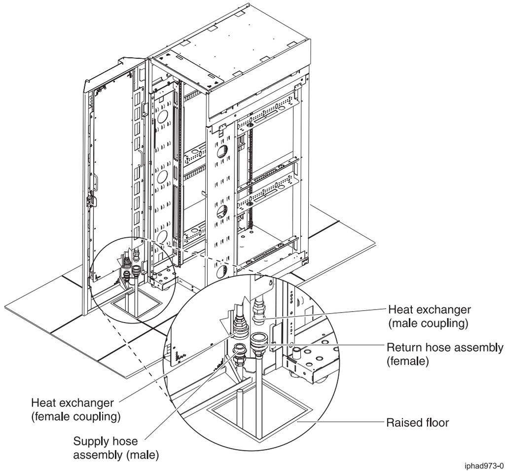
Figure 35. Raised floor hose management example 1; tile cut out size and position for 19-inch EIA-rail racks.
