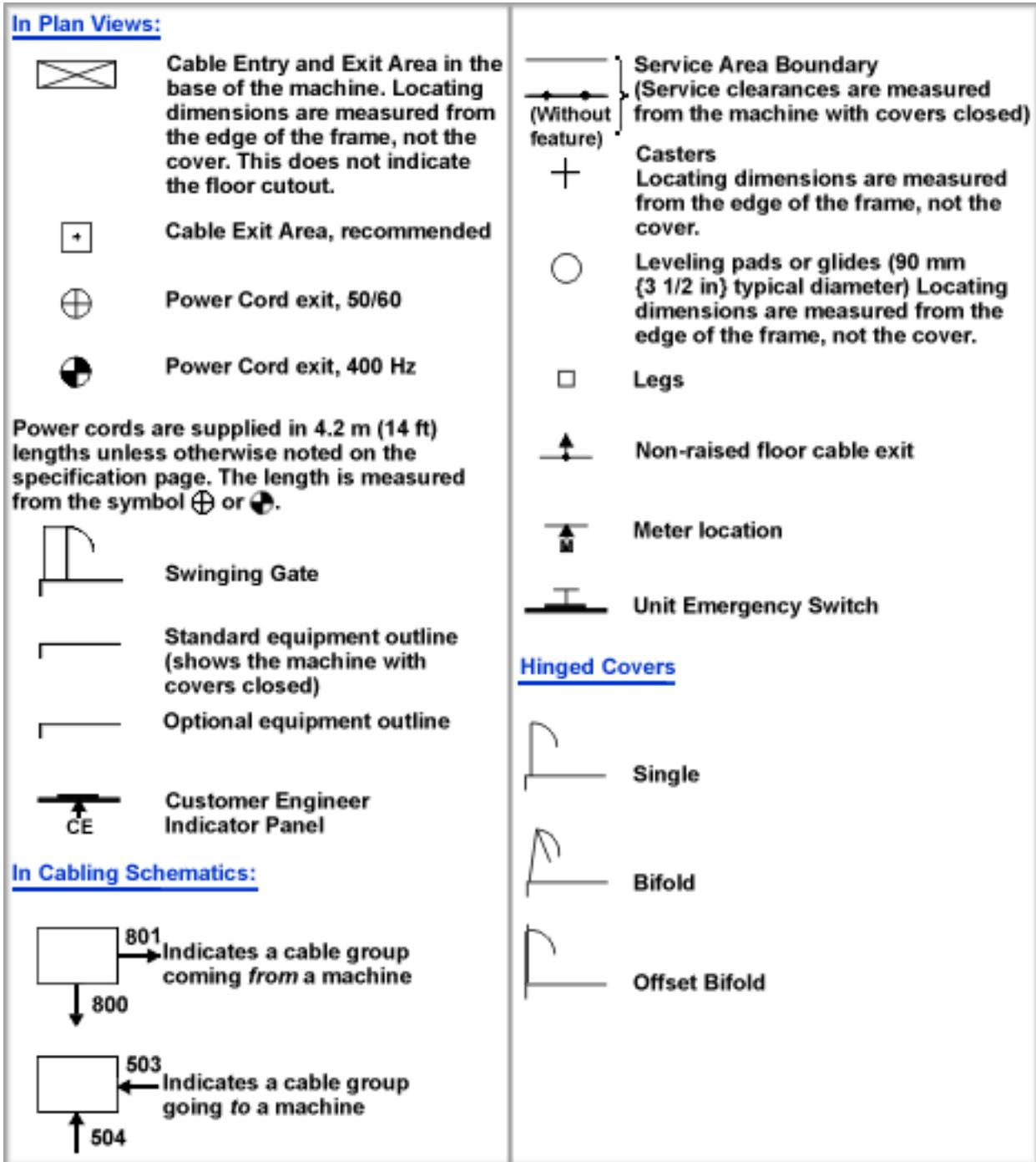
Figure 5. Standard symbols to create floor layouts
