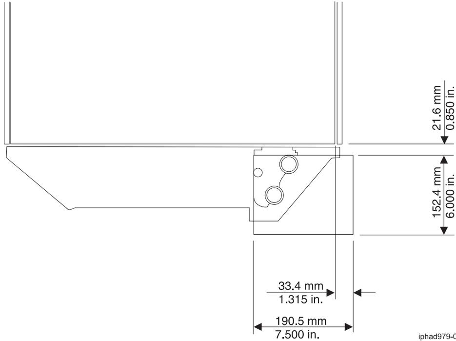
Figure 38. Raised floor hose management example 1; Tile cut out definition and location for 24-inch EIA-rail racks
