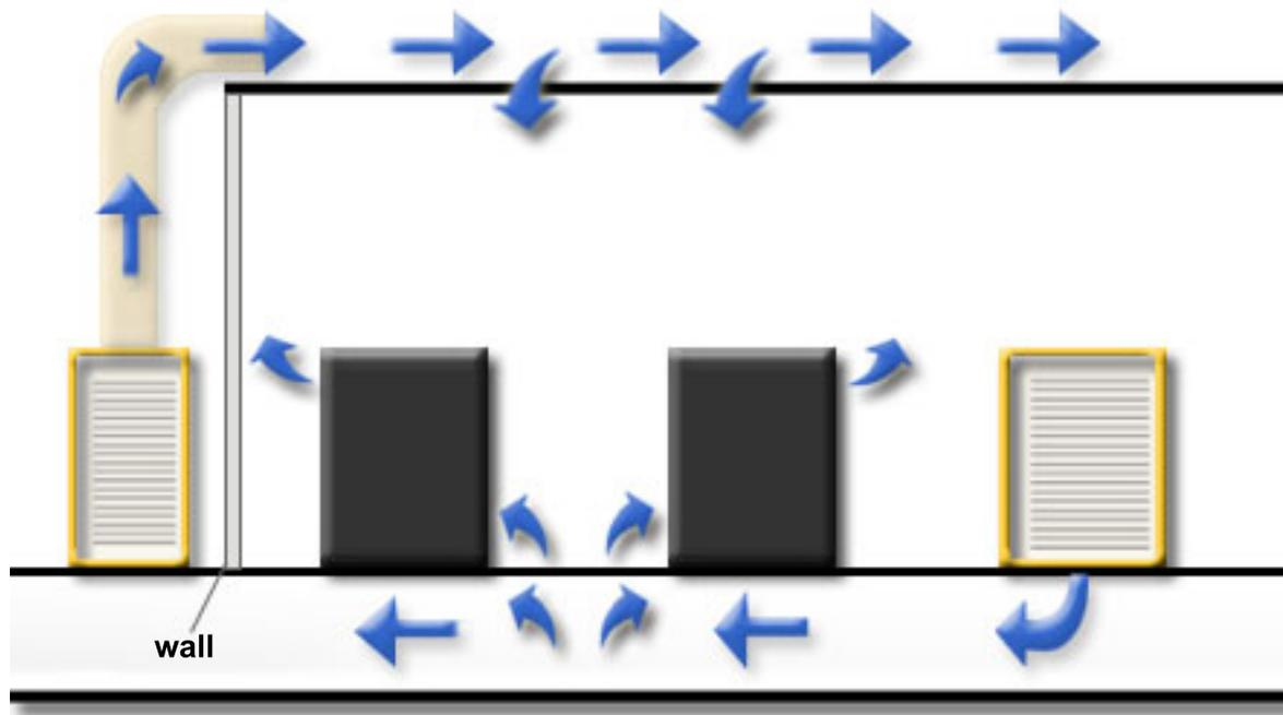
Figure 22. Combination overhead and underfloor air conditioning system
