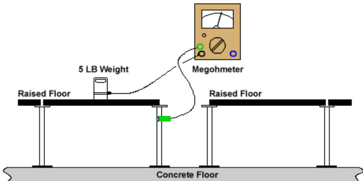
Figure 1. Typical test connection to measure floor conductivity
