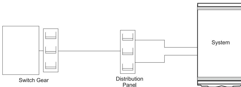
Figure 14. Single distribution panel - Dual circuit breakers
