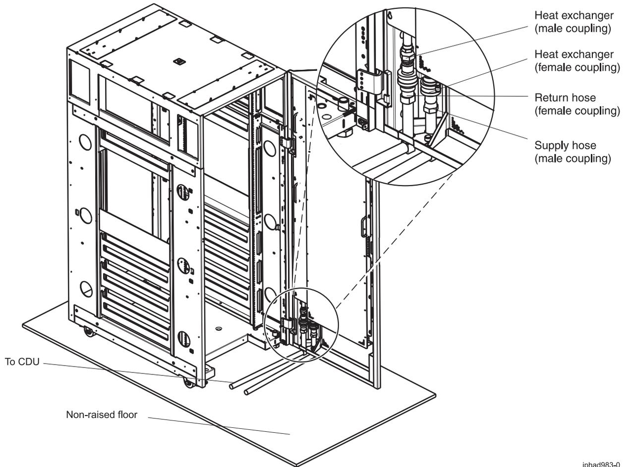
Figure 44. Non-raised floor hose requirements 24-inch EIA-rail rack
