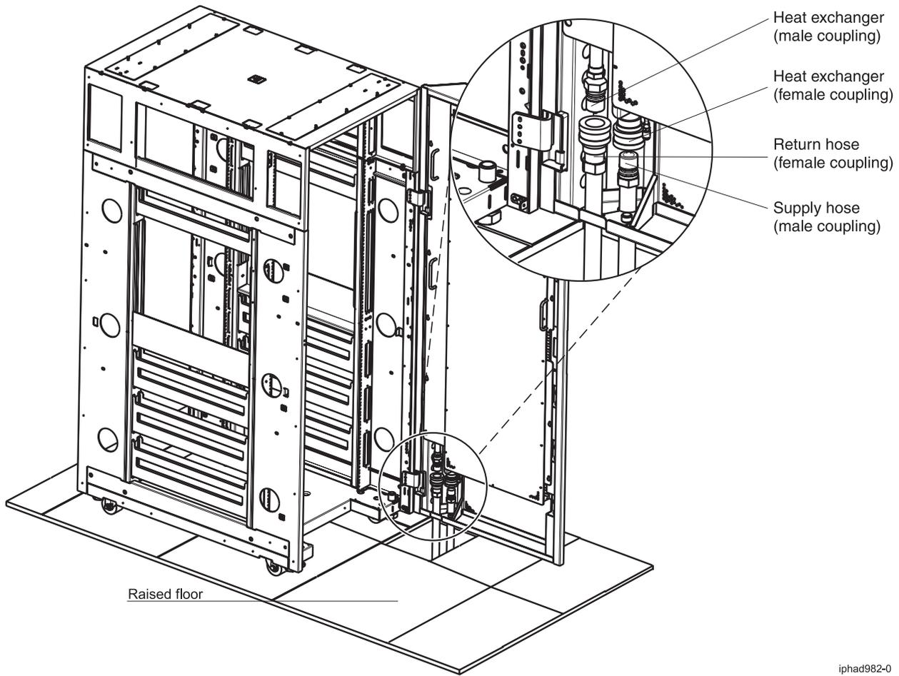
Figure 36. Raised floor hose management example 1; tile cut out size and position for 24-inch EIA-rail racks.
