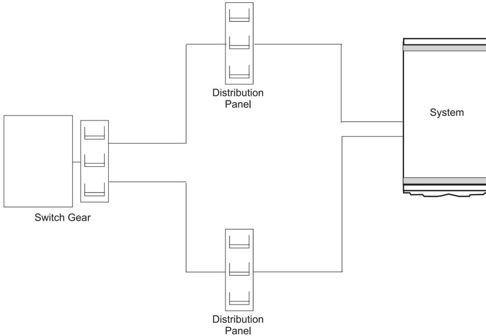
Figure 13. Dual power installation - Redundant distribution panel
