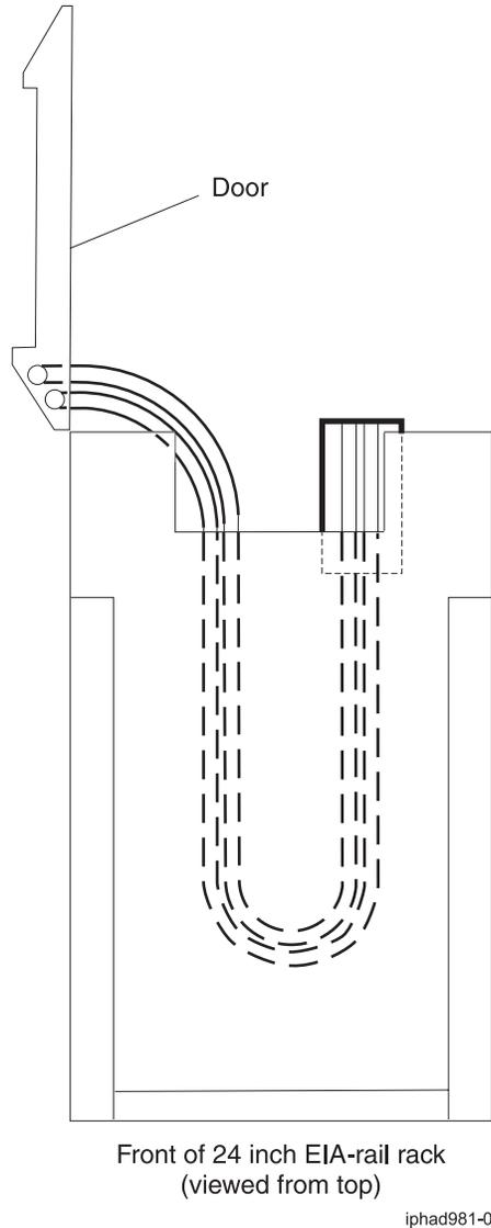
Figure 42. Raised floor and non-raised floor hose management example 2; loop under the 24-inch EIA-rail rack with door open
