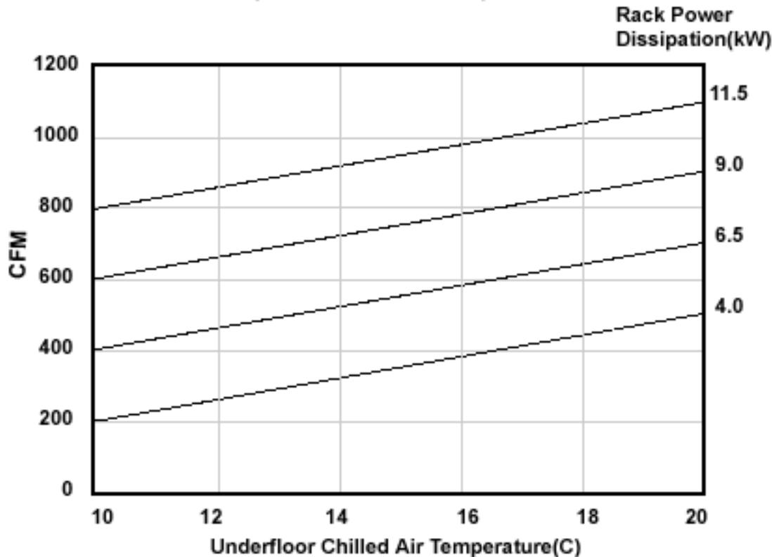
To determine the chilled air flowrates for higher altitudes add 1/2 C to the underfloor air temperature for every 1000 ft increase in altitude
