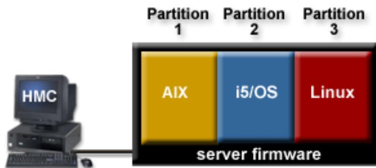
In this figure, you can see the logical partitions and the server firmware on the server. The *server firmware* is code that is stored in system flash memory on the server. The server firmware directly controls the resource allocations on the server and the communications between logical partitions on the server. The HMC connects with the server firmware and specifies how the server firmware allocates resources to the managed system.
