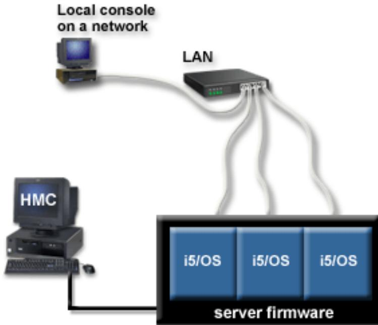
The following figure shows a partitioned IBM System i model with an HMC and local consoles directly attached to the server.
