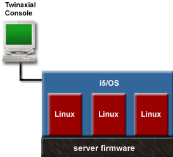
This figure illustrates the IBM i logical partition and the Linux logical partitions that are managed by the IBM i logical partition. The user creates and configures the Linux logical partitions on the server by accessing SST over the twinaxial console.
