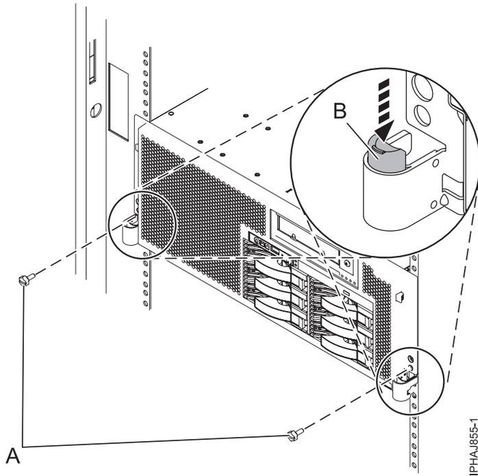
Figure 29. Releasing the rack latches
