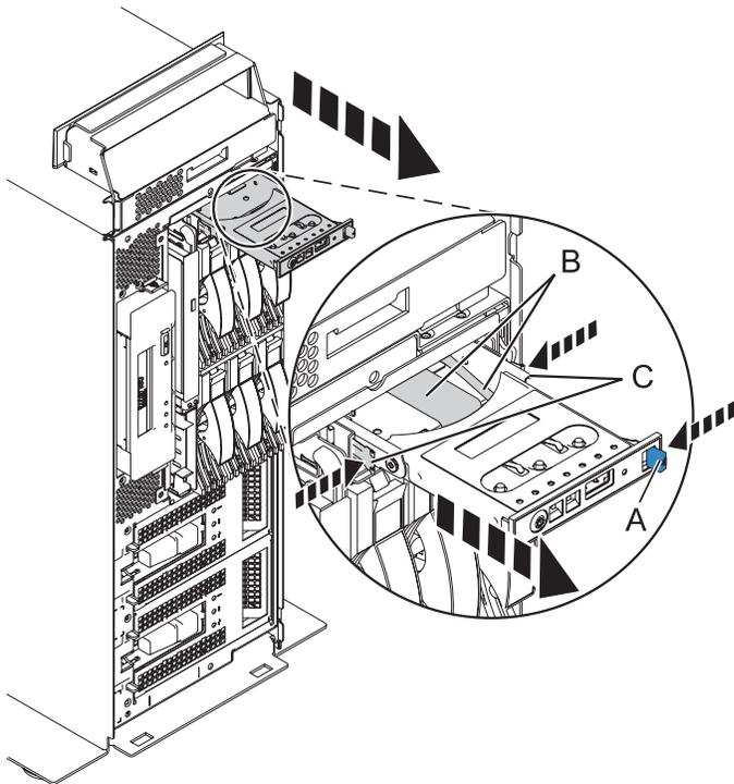
Figure 6. Control panel removal from a stand-alone system unit
