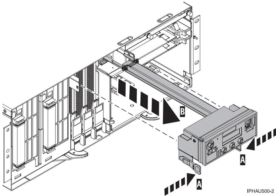
Figure 3. Control panel removal
