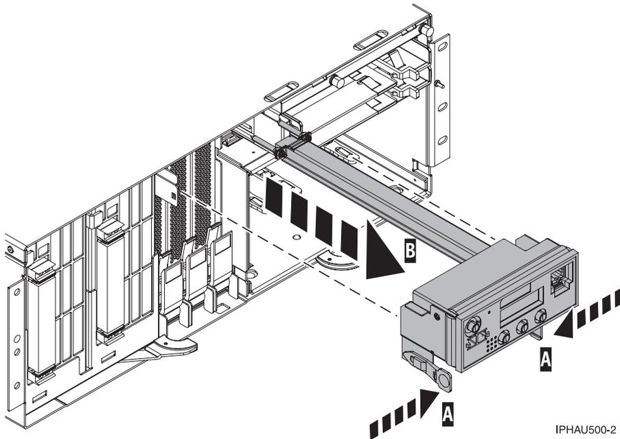
Figure 1. Control panel removal
