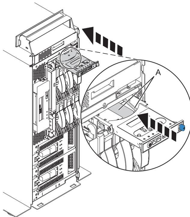
Figure 8. Control panel replacement in a stand-alone system unit
