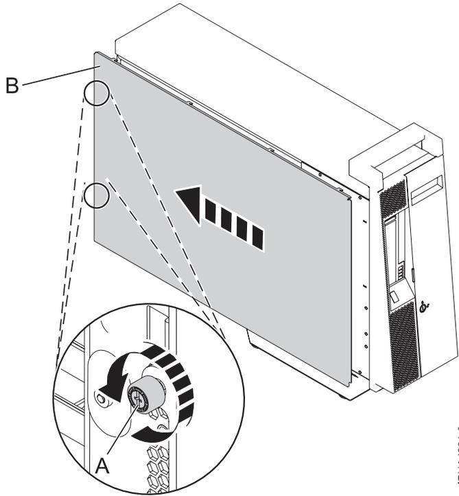
Figure 17. Removing the service access cover from the stand-alone model
