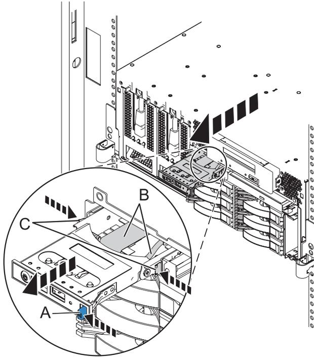
Figure 5. Control panel removal from a rack-mounted system unit
