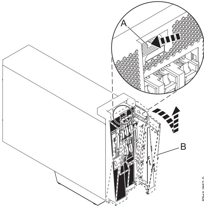
Figure 21. Remove the door from the model
