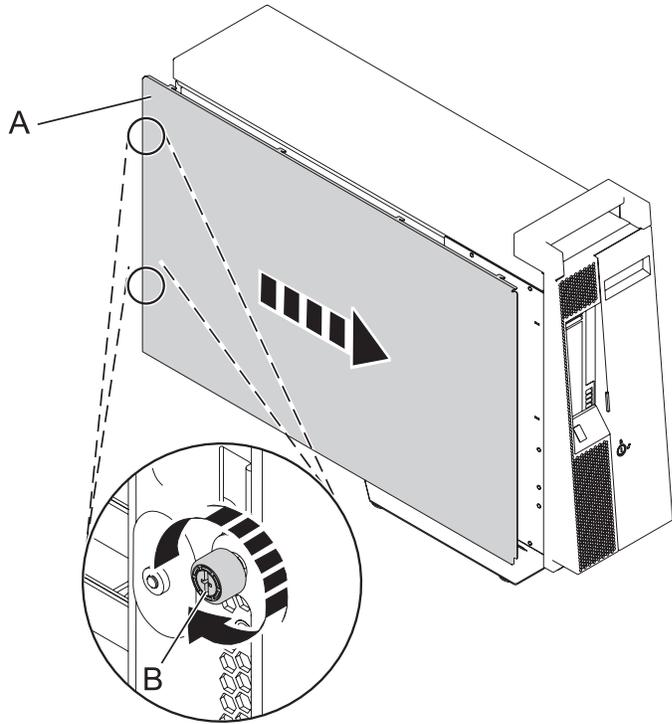
Figure 18. Installing the service access cover on a stand-alone model
