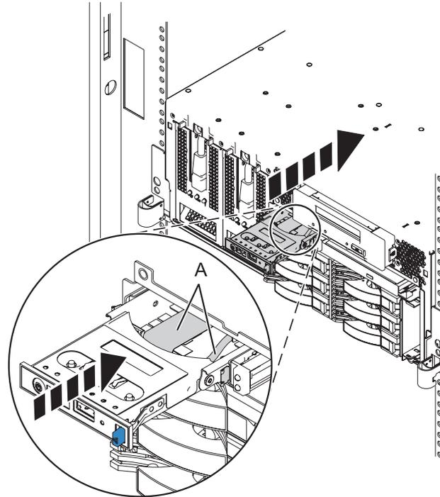
Figure 7. Control panel replacement in a rack-mounted system unit
