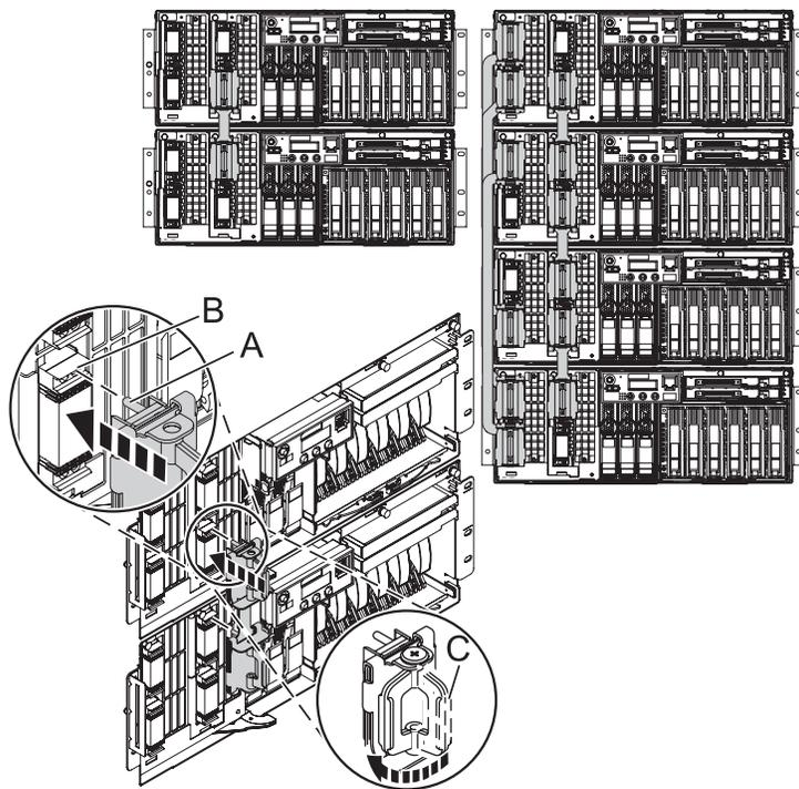
7. Align the guide pins **A** with the connector **B** on the system unit.
