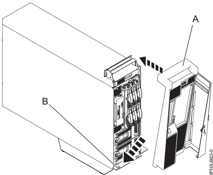
Figure 22. Replacing the cover on the model
