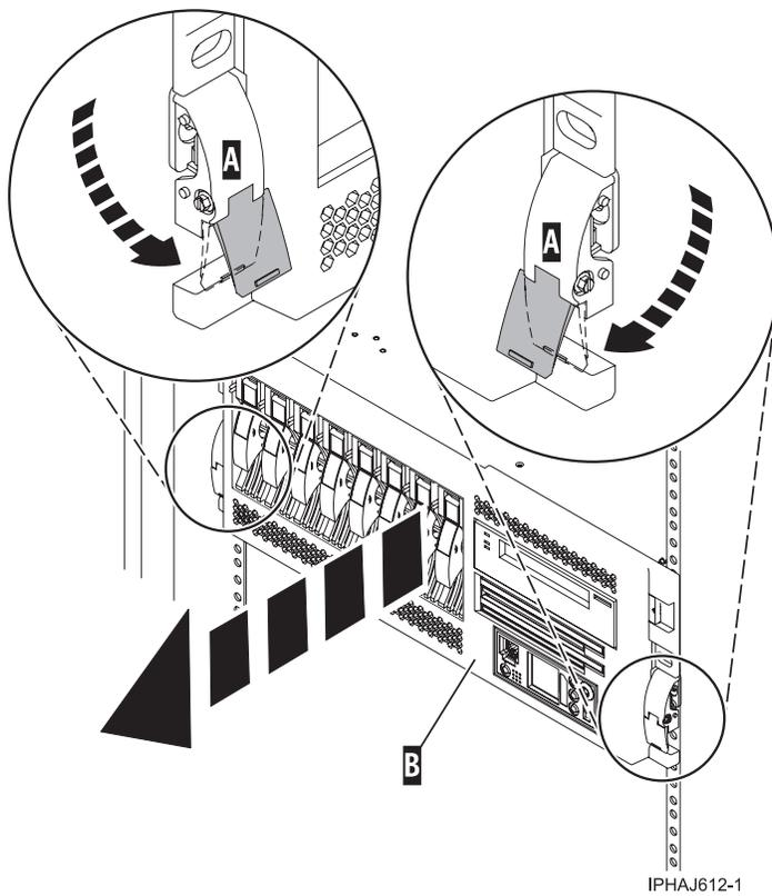
Figure 26. Releasing the rack latches
