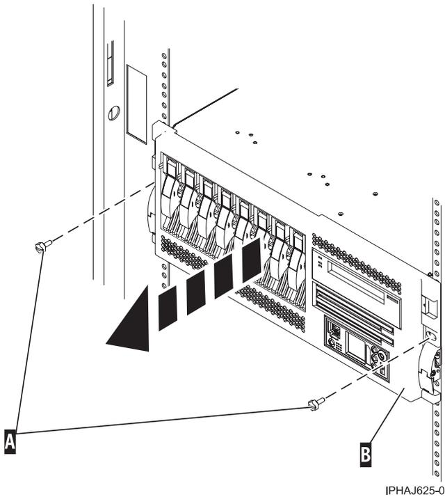
Figure 25. Removing the thumbscrews from the system and rack
