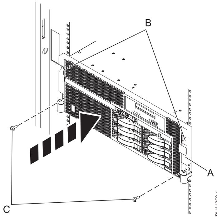
Figure 20. Installing the front cover on a rack-mounted model
