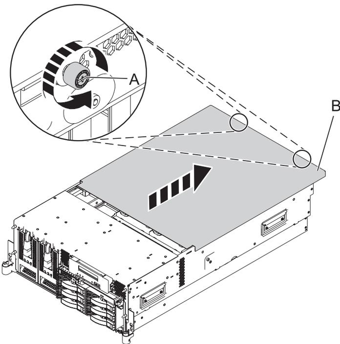
Figure 15. Remove the service access cover from a rack-mounted model
