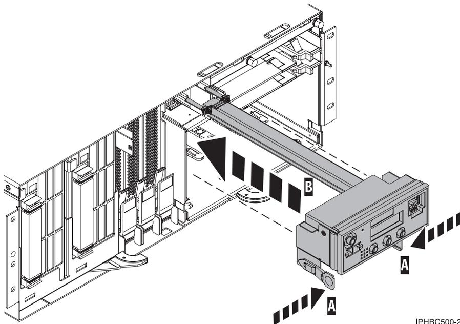
Figure 2. Control panel replacement
