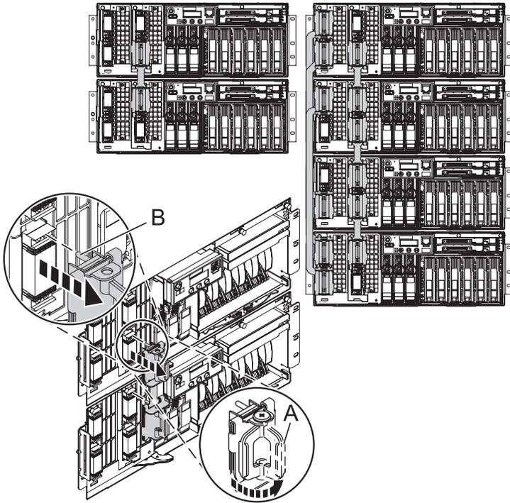
7. Carefully pull the connector from the system.
