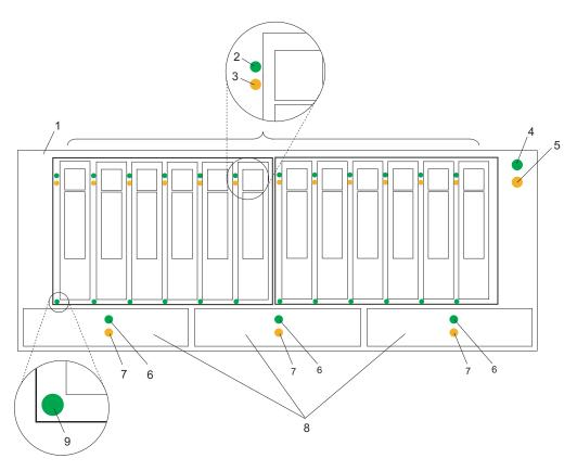
Figure 6. I/O enclosure front view showing maintenance LEDs
