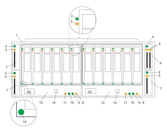
Figure 7. I/O enclosure rear view showing maintenance LEDs
