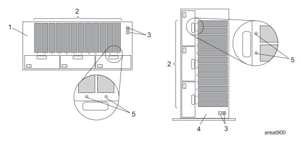
Figure 1. Front view of your I/O enclosure
