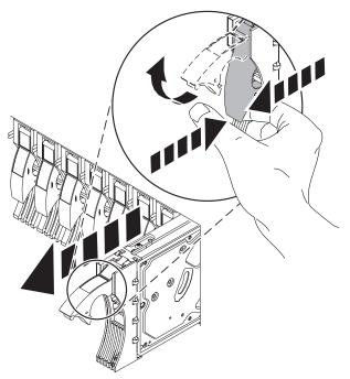
Loosen and pull out on the thumbscrew B to release the disk-drive bezel C from the disk drive, as shown in the graphic.
