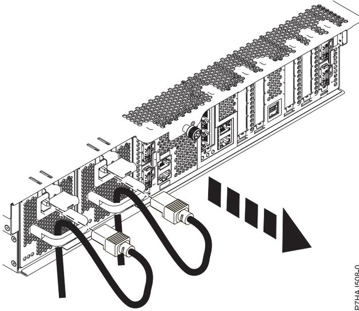
Figure 15. Removing the power cords
