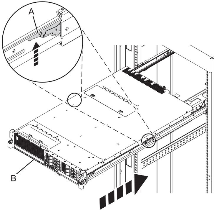
Figure 13. Unlocking the safety rail latches
