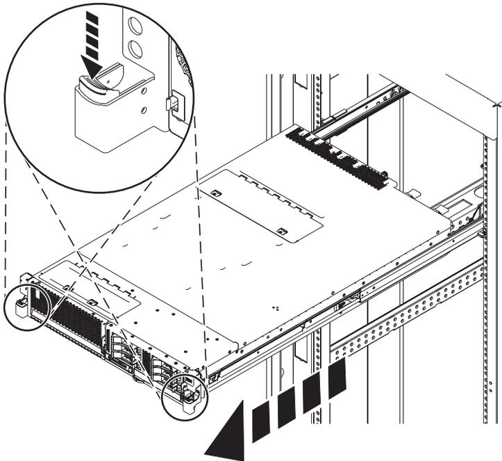
Figure 12. Placing the system in the service position
