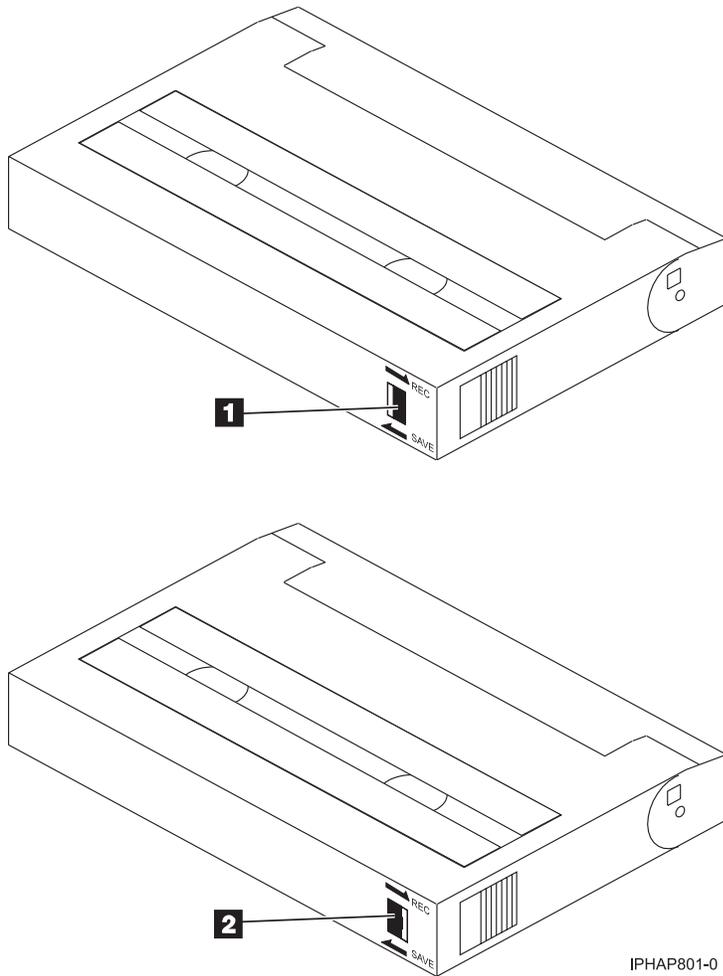
When the switch is set to the left in the SAVE position **1**, data cannot be written to or read from the tape (data is saved).
