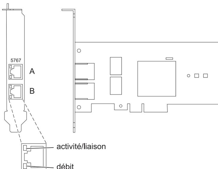
Figure 36. Carte PCI Express Ethernet 10/100/1000 Base-TX 2 ports
