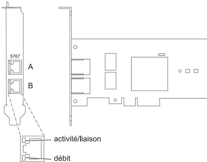
Figure 49. Carte PCI Express Ethernet 10/100/1000 Base-TX 2 ports
