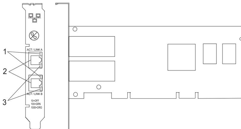
Figure 40. Adaptateur 2 ports 10/100/1000 Base-TX Ethernet PCI-X
