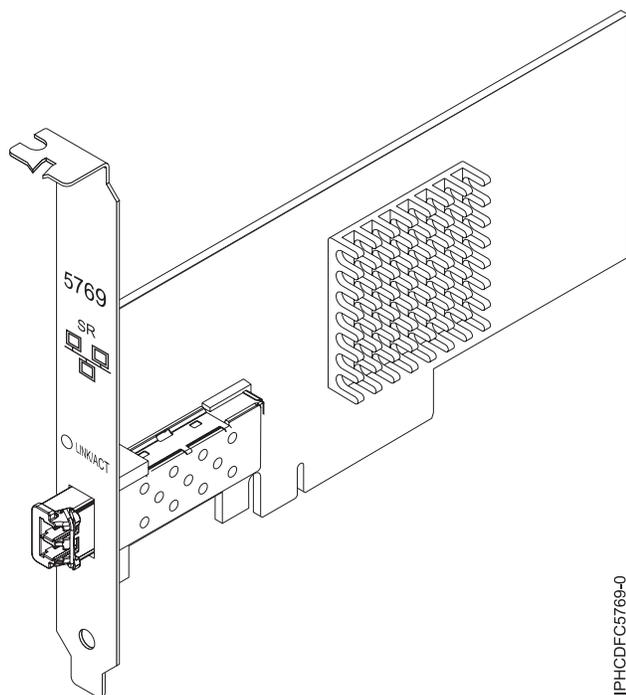
Figure 51. carte PCIe 10 Gigabit Ethernet-SR
