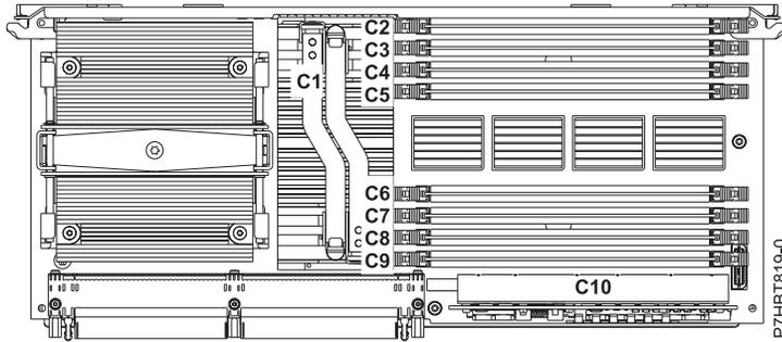
Figure 9. Processor voltage regulator module, location C1.
