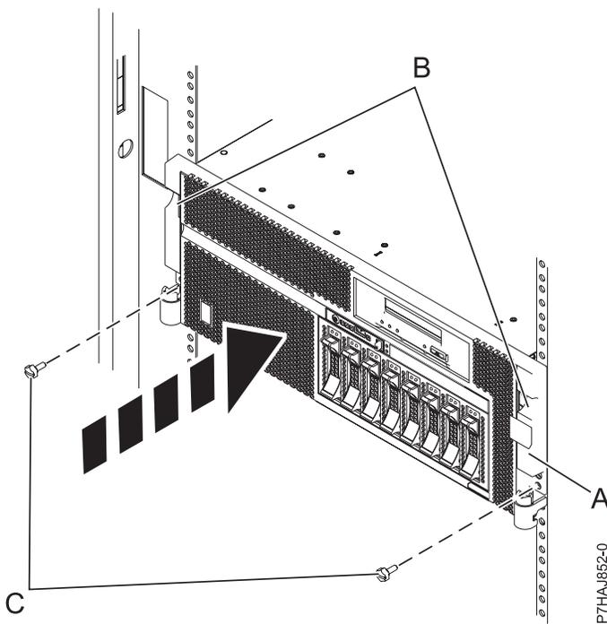
Figure 22. Replacing the thumbscrews
