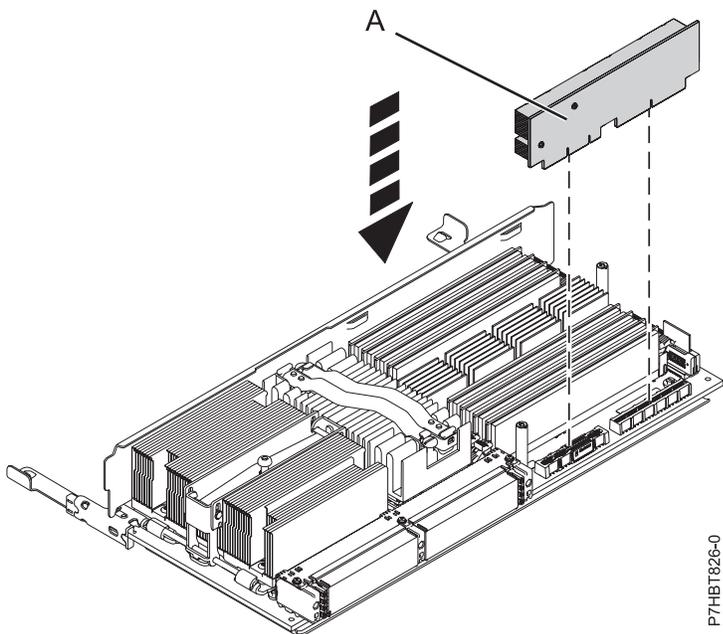
Figure 8. Installing the memory voltage regulator module
