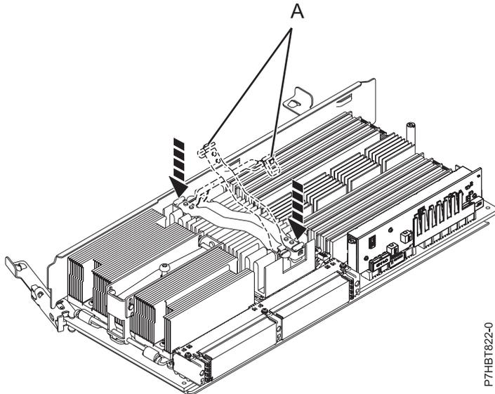
4. Install the airflow cover as shown in the following figure.
