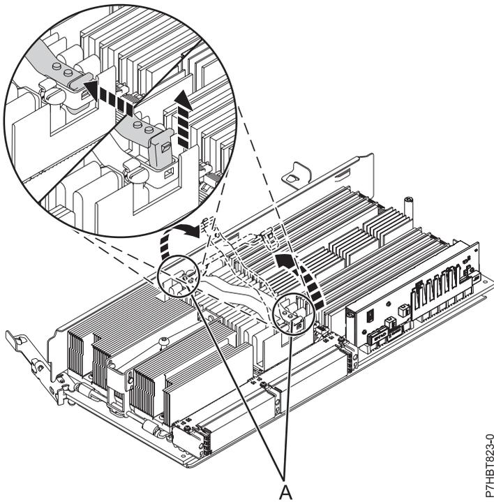
Figure 11. Unlocking the processor voltage regulator module arms
