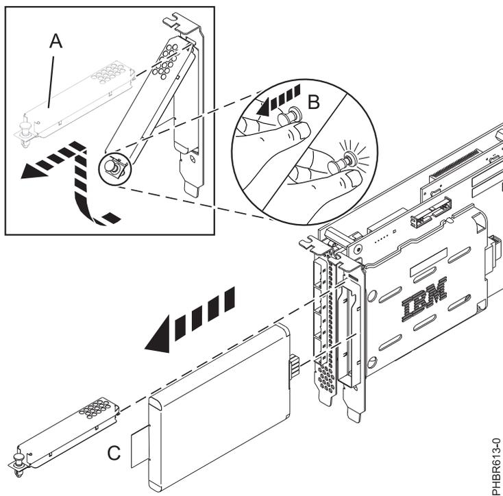
Figure 28. Replacing the 572F/575C cache battery
