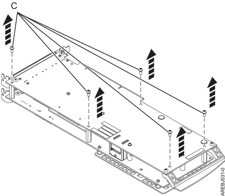
Figure 30. Location of screws on the 572F/575C card set adapter
