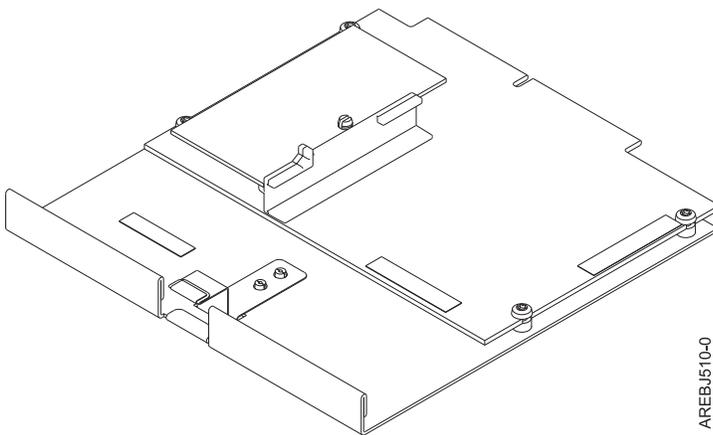
Figure 4. CCIN 57B8 planar RAID enablement card
