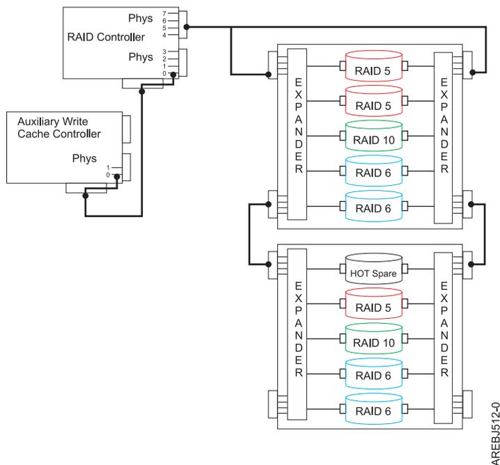
Figure 22. Example RAID and AWC controller configuration
