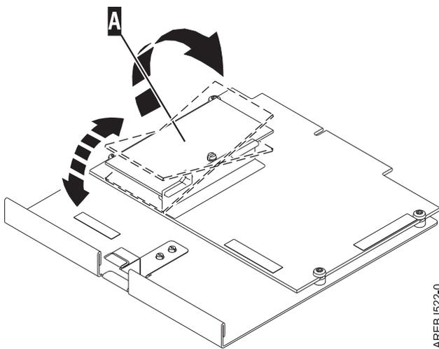
3. Unseat the connector on the cache directory card by wiggling the two corners over the connector, using a rocking motion. Then lift the cache directory card off the connector and out of the guides on the plastic support rail.
