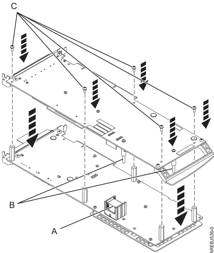
Figure 34. Reassembling the cards
