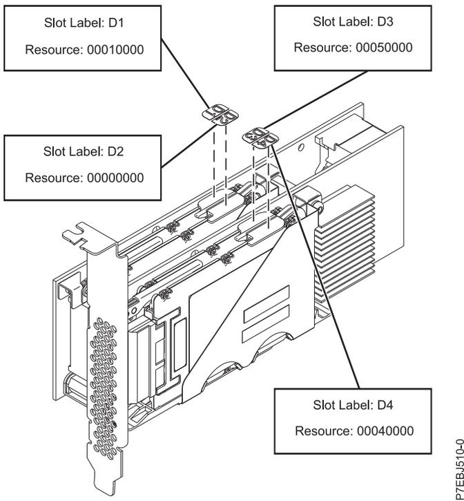
Figure 37. SAS resource locations for CCIN 57CD PCIe SAS RAID and 3 Gb x8 SSD Adapter
