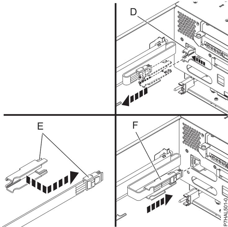
Figure 49. SAS cable connections
