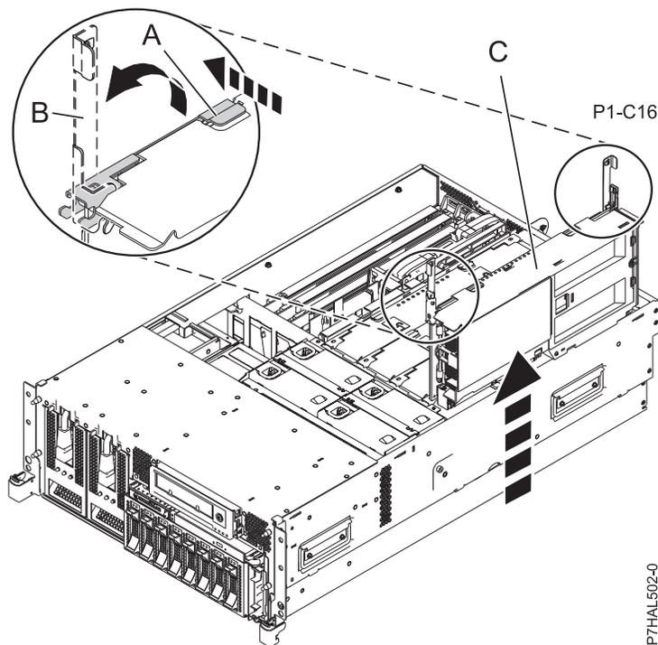
6. Remove the fans and fan cage from the system by doing the following steps:
