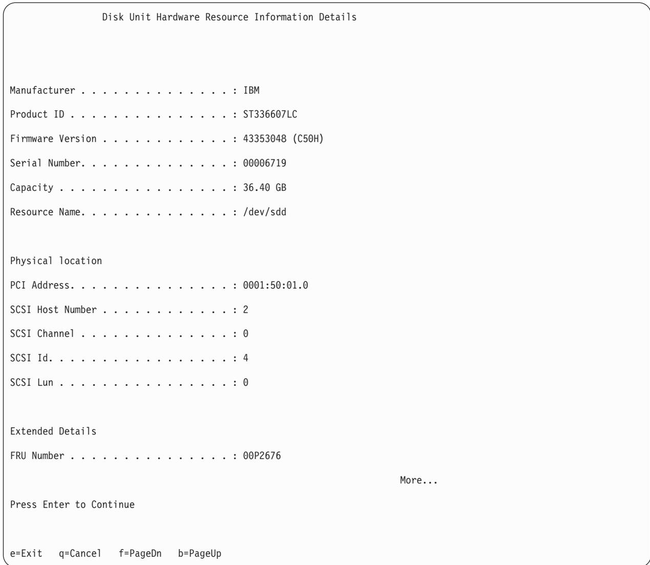
Figure 75. Example Disk Hardware Resource Information Details display
