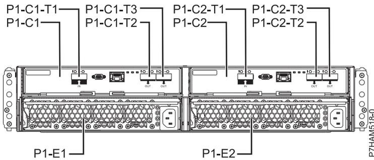
Figure 64. Rear view of the 5887 disk-drive enclosure
