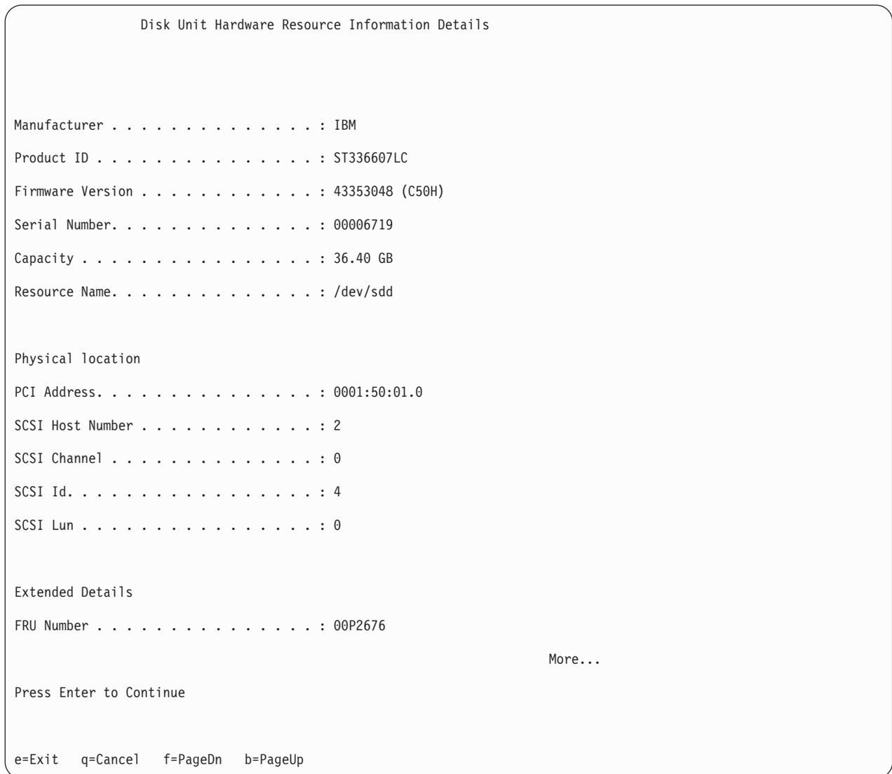
Figure 28. Example Disk Hardware Resource Information Details display
