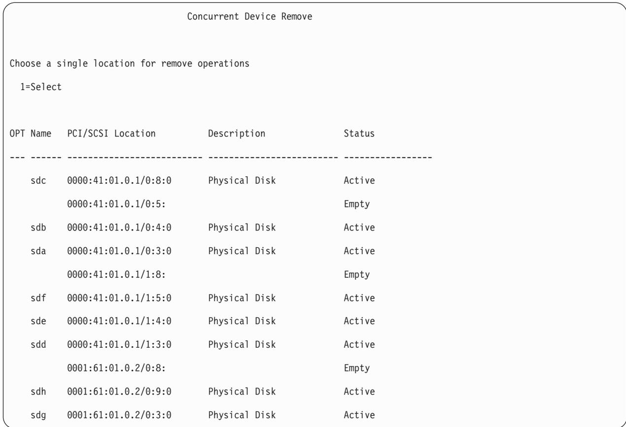
Figure 29. Example Concurrent Device Remove display
