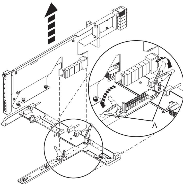
Figure 100. Removing the SAS conduit card from the midplane
