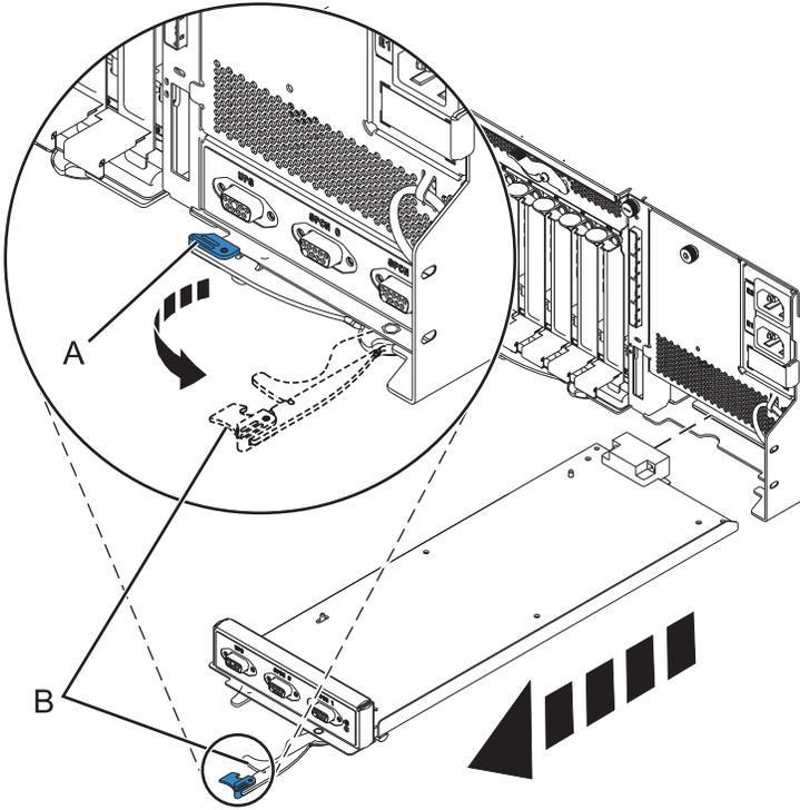
Figure 96. Remove the enclosure management controller
