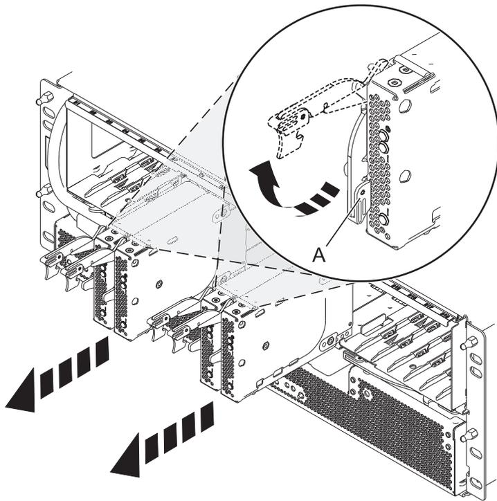
Figure 102. Removing the SAS expander card.
