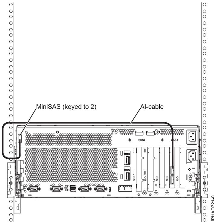
**Notes:** The second connector on the adapter can be used to attach a disk expansion or media expansion drawer.
