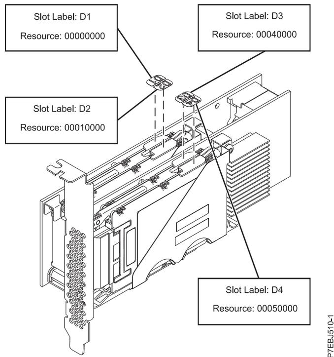
Figure 60. PCIe RAID and SSD SAS adapter locations
