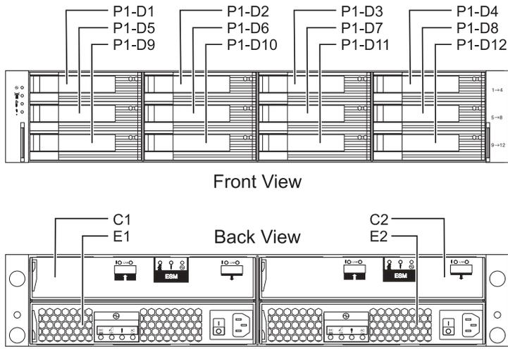
Figure 66. Disk drive locations for the 5886 disk-drive enclosure
