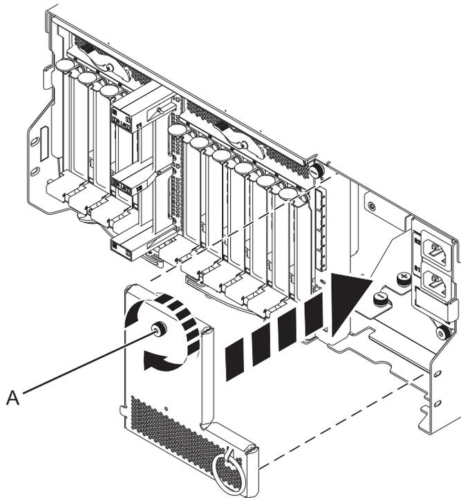
Figure 86. Installing the power cord plate
