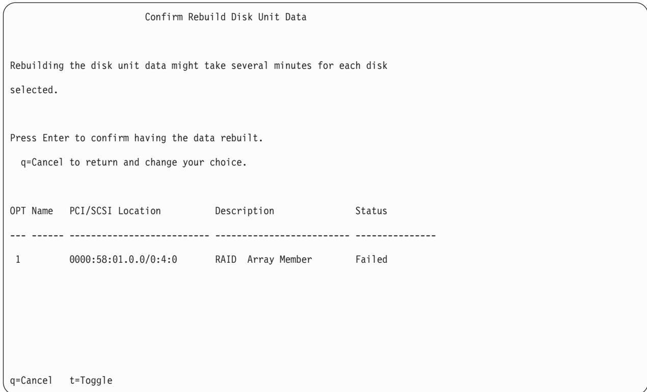
Figure 83. Example Confirm Rebuild Disk Unit Data display
