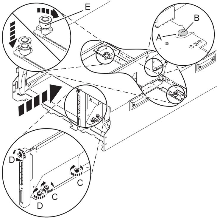
Figure 85. Installing the SAS conduit card and the midplane
