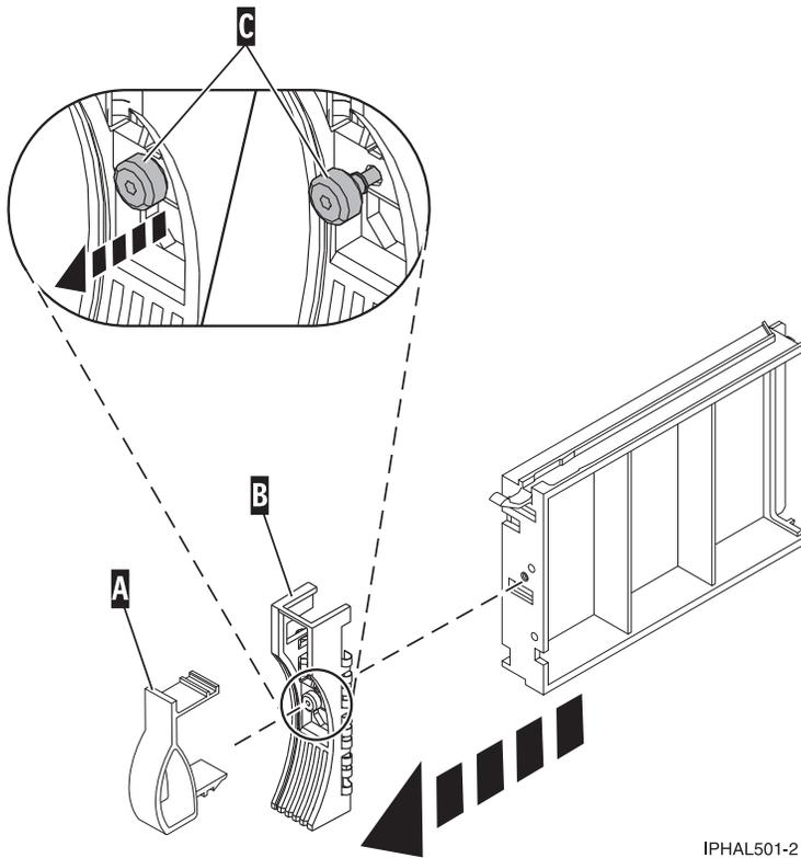
Figure 55. Removing a disk drive bezel
