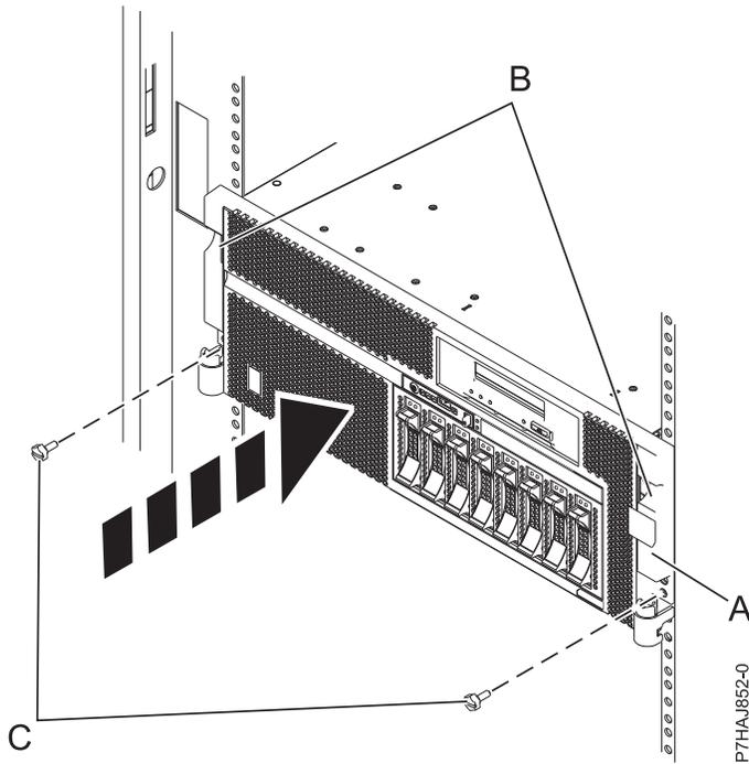
Figure 106. Installing the front cover
