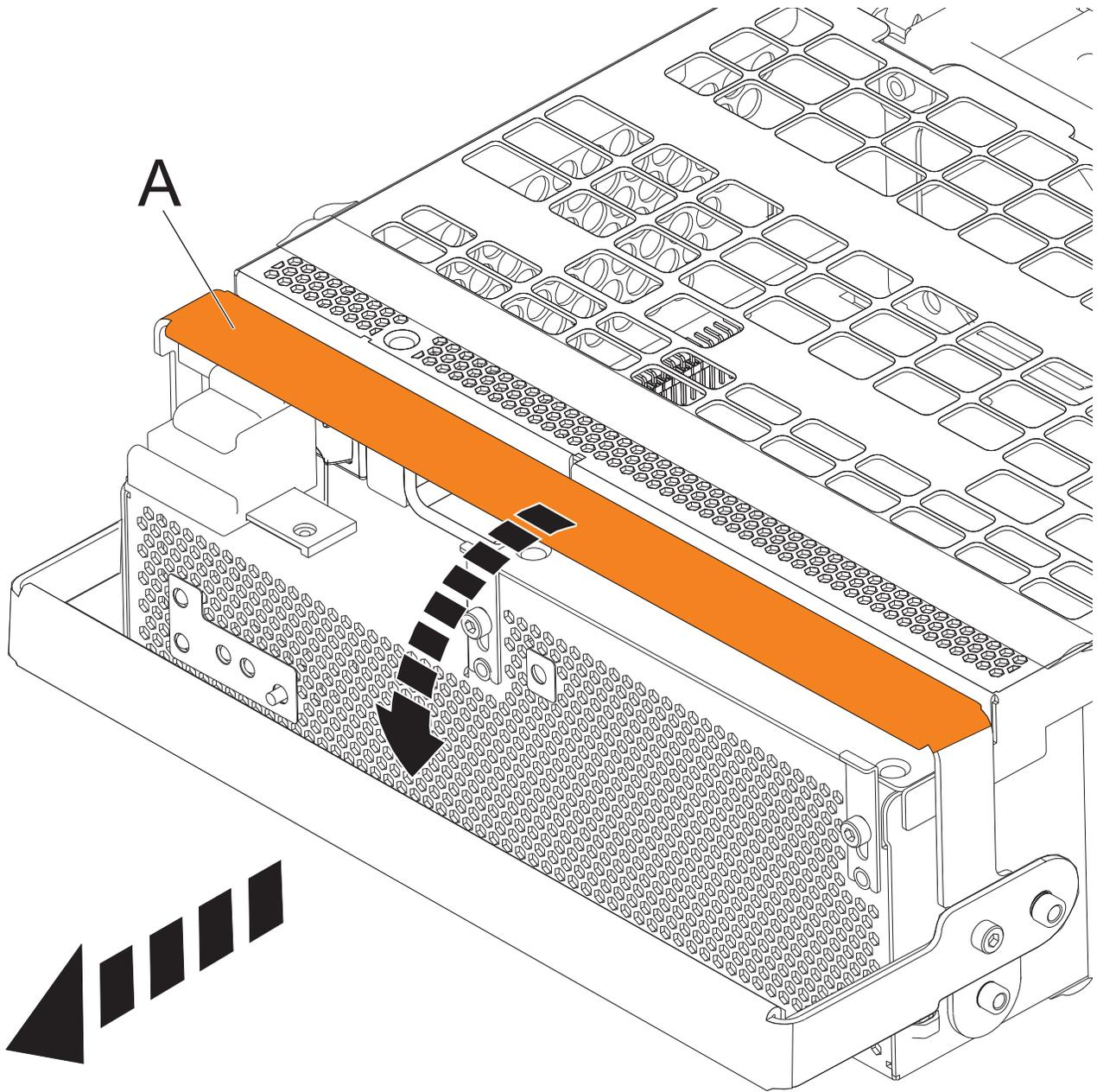
Figure 95. Remove the offline converter assemblies
