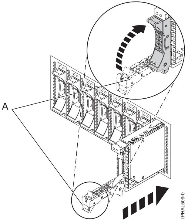
Figure 2. Installing a small-form factor disk drive
