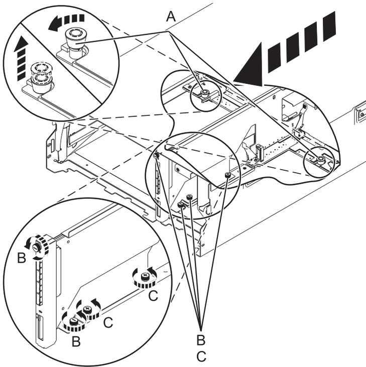
Figure 99. Removing the SAS conduit card and midplane
