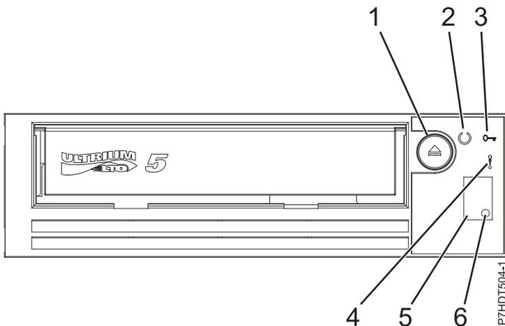
Figure 2. Front view of half high LTO Drive
