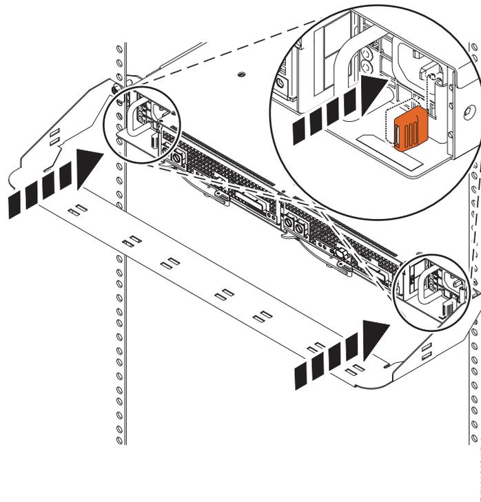
Figure 3. Docking the power supply
