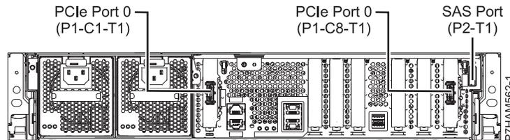
Figure 29. Model 31E/2C connections for PCIe storage enclosures
