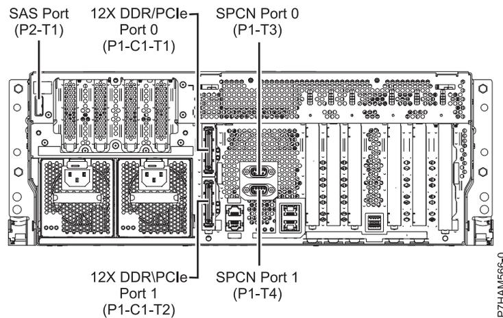
Figure 25. Model 02E/4C connections for expansion units, disk drive enclosures, and PCIe storage enclosures
