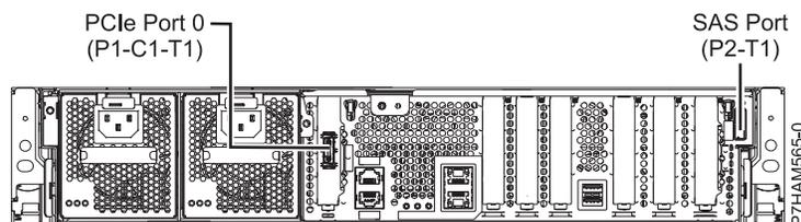
Figure 27. Model 31E/1C connections for disk drive enclosures and PCIe storage enclosures
