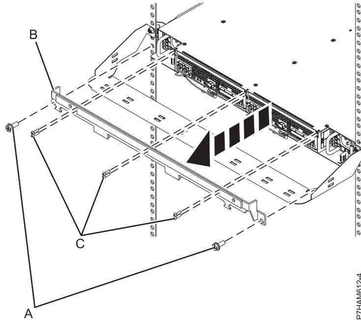
Figure 2. Removing the rear shipping bracket
