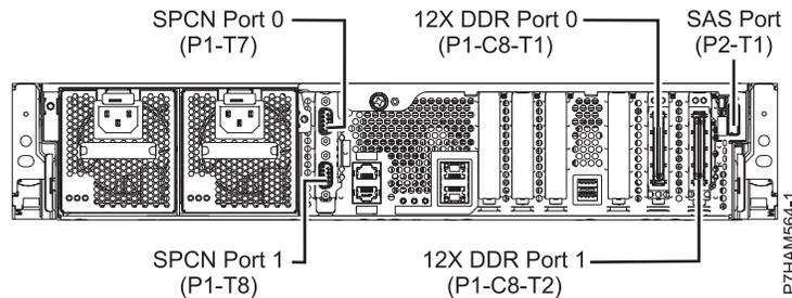
Figure 28. Model 31E/2C connections for expansion units and disk drive enclosures
