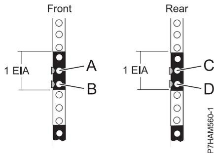
Figure 8. Marking the installation locations
