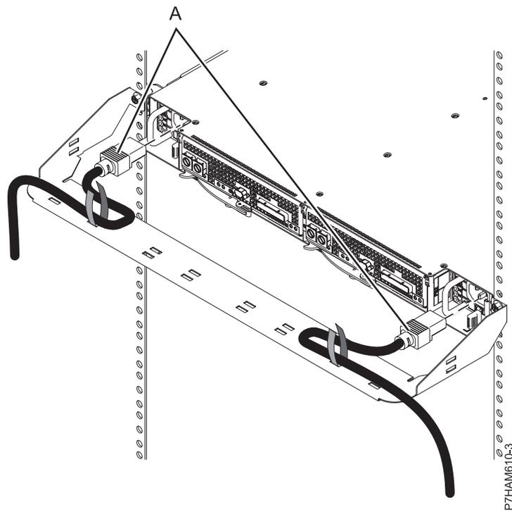
Figure 6. Installing the power cords
