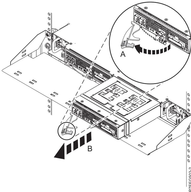
Figure 1. Removing an ERM assembly from the enclosure
