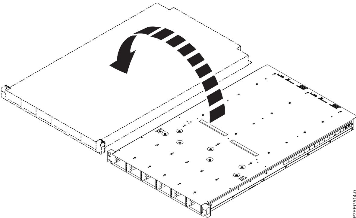
Figure 18. Turning the enclosure top side up
