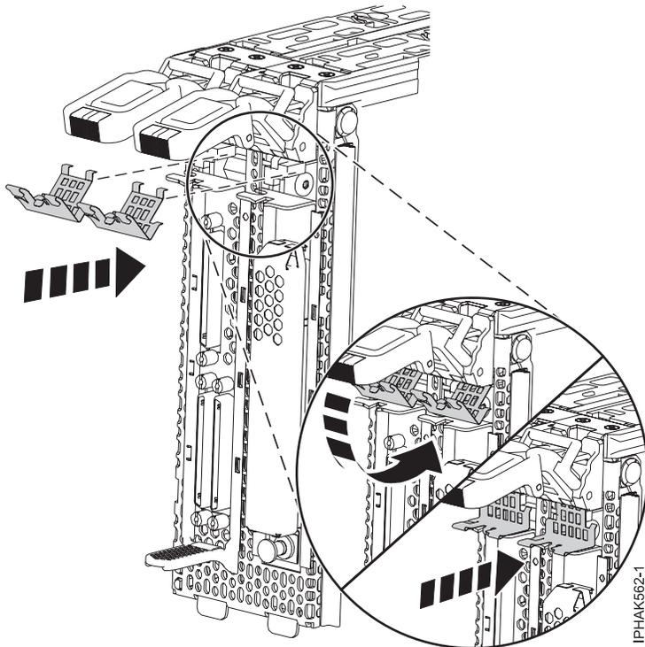
Figure 60. Inserting the two metal clips into the front of the assembly
