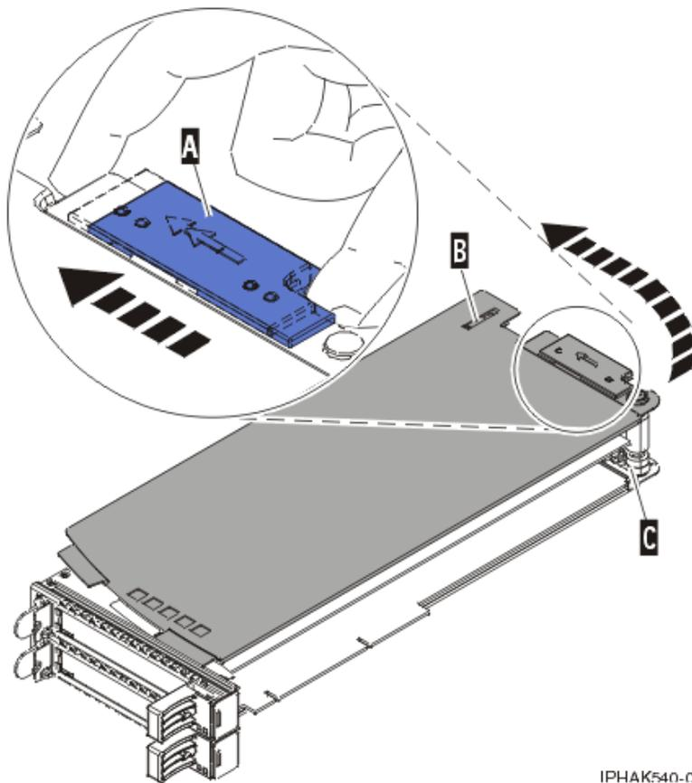
Figure 149. PCI adapter cassette cover replaced
