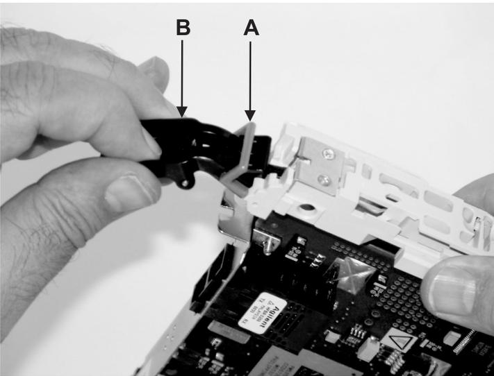
a. Lower the lever (B) on the cassette linkage assembly until it moves into the down position (the adapter or blank filler should move up into the cassette assembly).
