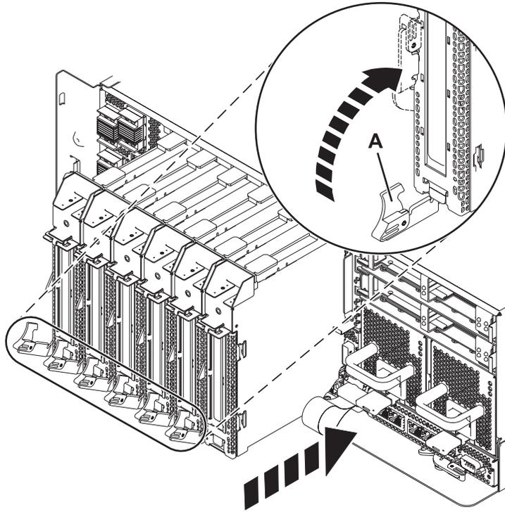
Figure 10. PCI adapter cassette installed in the system unit
