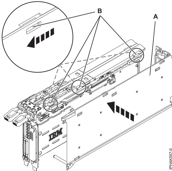
Figure 55. Installing the cover
