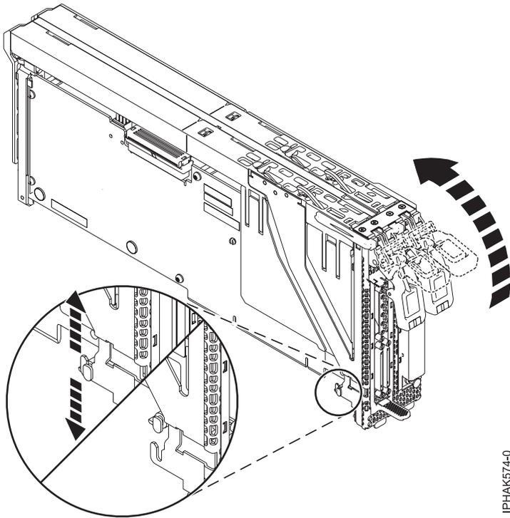
Figure 67. Detaching the face plate
