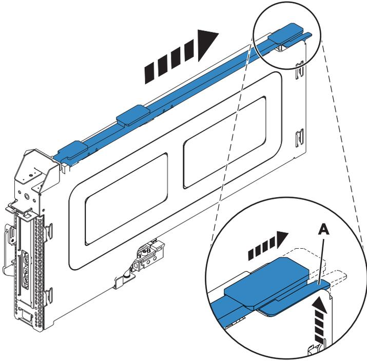
Figure 20. PCI adapter cassette guide rail removed
