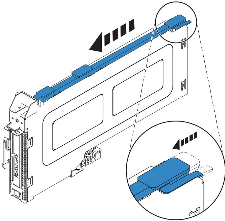
Figure 24. PCI adapter cassette guide rail locked
