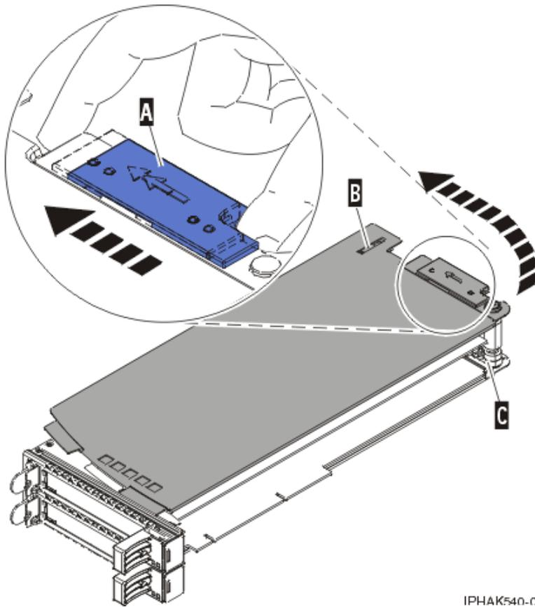
Figure 43. PCI adapter cassette cover replaced
