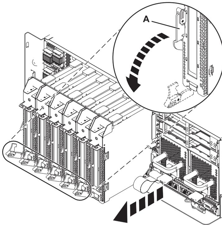
Figure 7. PCI adapter cassette removed from the system unit
