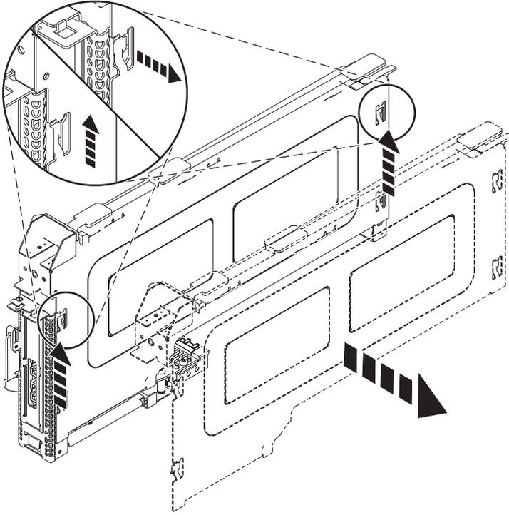
Figure 16. PCI adapter cassette cover removed
