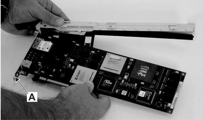
Remove the adapter from the cassette linkage assembly by rotating the bottom of the tailstock **A** out as shown in the illustration. Store the adapter in a safe place.
