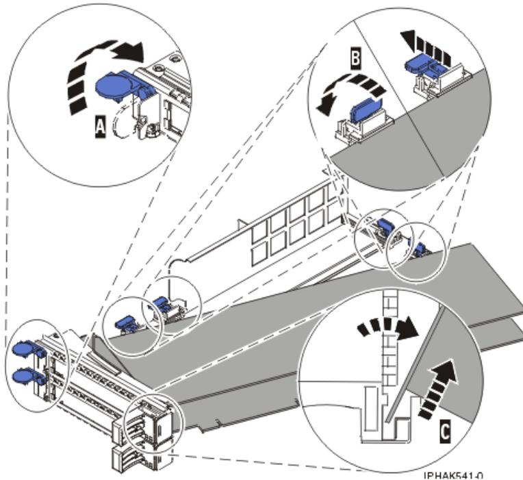
Figure 119. Adapter removed from the PCI adapter cassette
