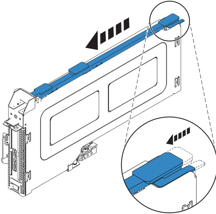
Figure 19. PCI adapter cassette guide rail locked
