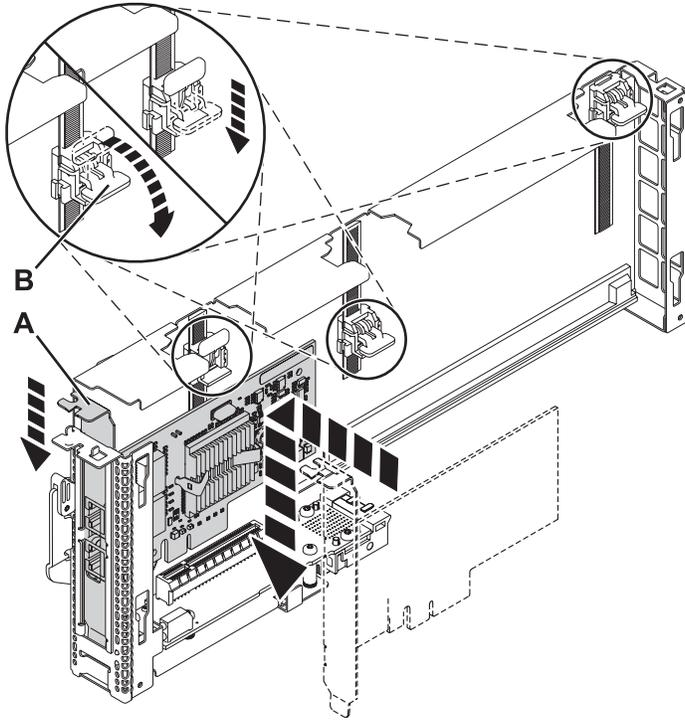
Figure 17. Adapter installed into the PCI adapter single-width cassette
