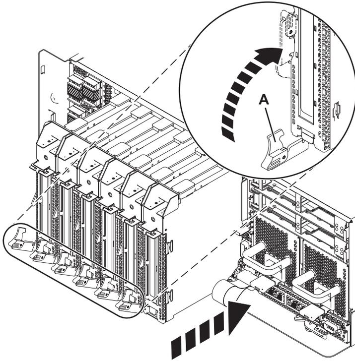
Figure 12. PCI adapter cassette removed from the system unit
