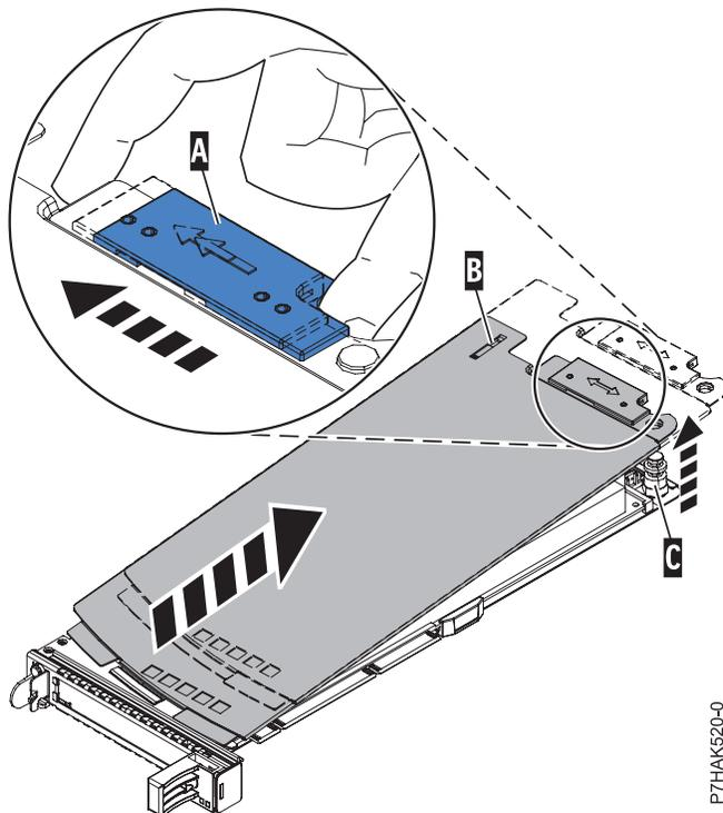
Figure 129. PCI adapter cassette cover removed
