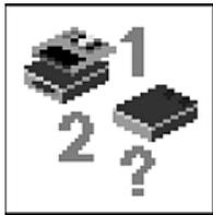
This selection enables you to view and change the custom boot list (the sequence in which devices are searched for operating system startup code).
