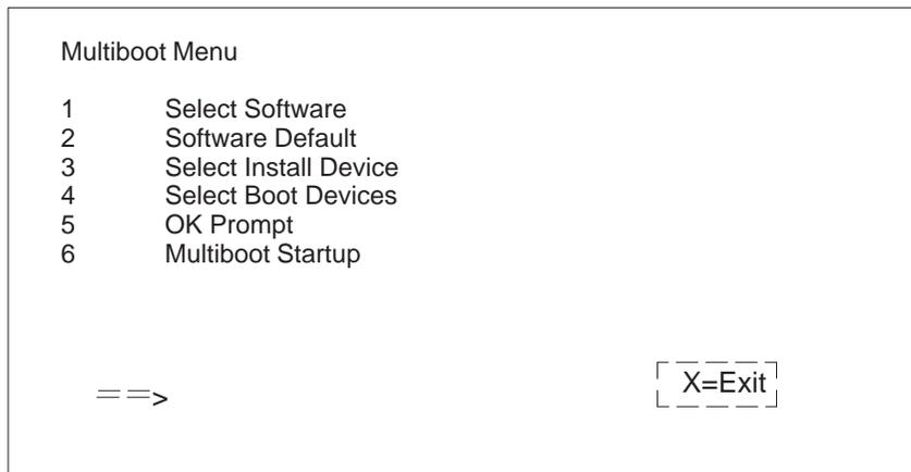
**Select Software:** If supported by the operating system, this option shows the names of the operating system installed. This option may not be supported by all operating systems.
