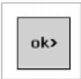
**OK Prompt:** Enables you to go directly to the Open Firmware command prompt. The Open Firmware command prompt is used for debugging and device driver development. For more information about the operation of the Open Firmware command prompt, refer to IEEE Standard 1275.
