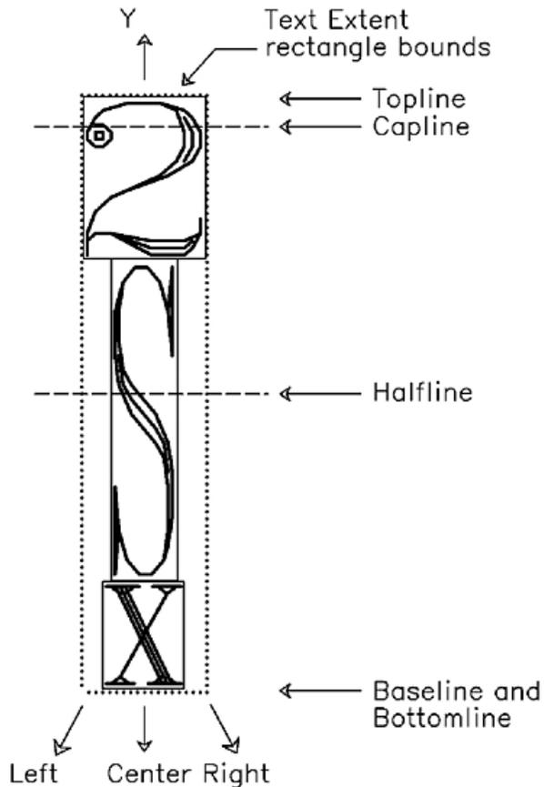
Figure 8. Alignment of a text string specified with path up or down. This illustration shows how vertical alignment can affect characters.
