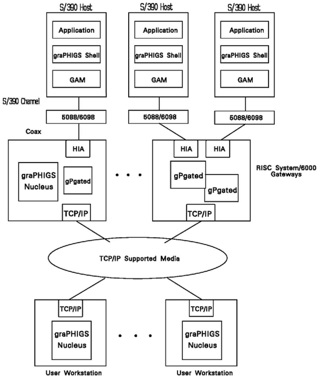
Figure 2. GDDM/graPHIGS API Application to graPHIGS API Remote Nucleus Flow. This diagram depicts a distributed graPHIGS application running on various hardware configurations which are attached through a central TCP/IP network. Several S/390 Host systems are shown running instances of the graPHIGS application and Shell, using the GAM to communicate across an IBM 5088 or 6098 communications controller to network-connected RS/6000 gateway systems.
