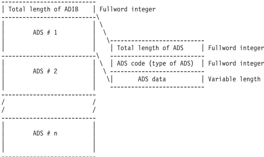
The ADS code identifies the type of ADS. The ADS data is a variable length field and is dependent on the type of ADS.
