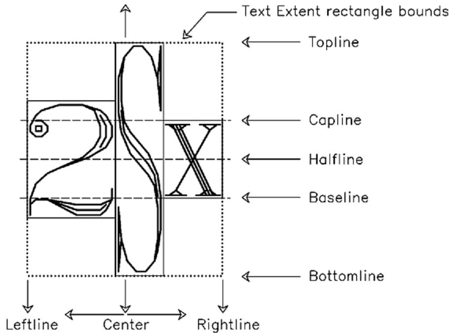
*Figure 7. . This illustration shows how horizontal alignment can affect characters.*
