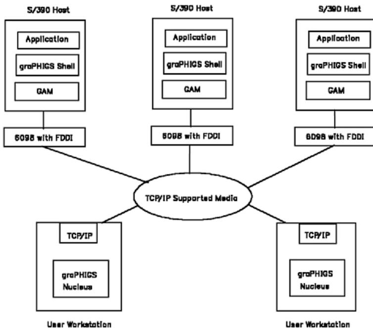
Figure 3. *graPHIGS/GAM Direct Connection.* This diagram depicts a distributed *graPHIGS* application in which the *S/390* Host systems are using the *GAM* to communicate to network-connected *6098* systems with the *FDDI* feature.
