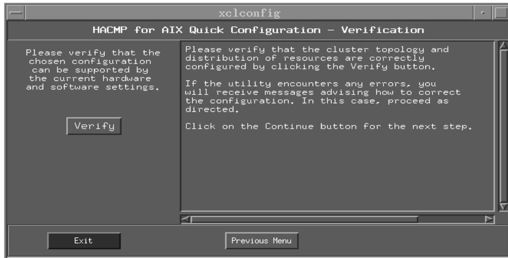
When you click on the **Verify** button, the system runs the HACMP for AIX `/usr/sbin/cluster/diag/clverify` utility. Output is displayed in the Help Information area, and is also logged to the `/tmp/qconfig/clverify.log` file. If errors are noted, correct them as instructed. Verification succeeds if the required hardware and cluster topology are available and properly configured.
