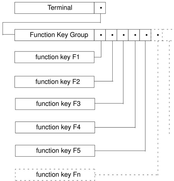
Relational diagram for the definition of an emulated terminal set-up.
