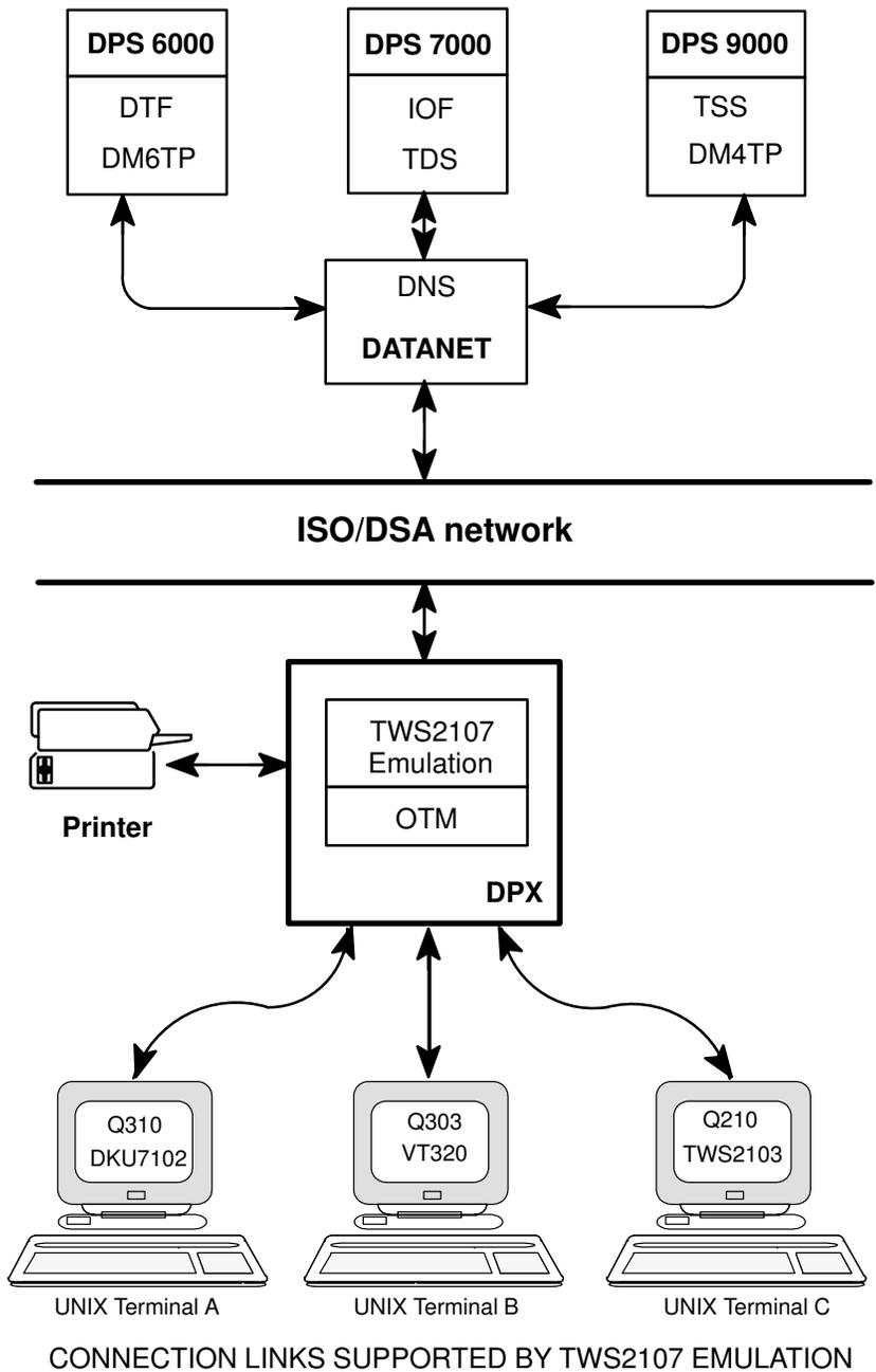
Figure 1. OTM Using TWS2107 Emulation
