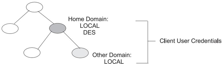
*Figure 14. Credential and Domains. This illustration shows a domain hierarchy. The user's home domain has local and DES credentials. The subdomain only has local credentials. Home and the subdomain are labeled Client User Credentials.*
