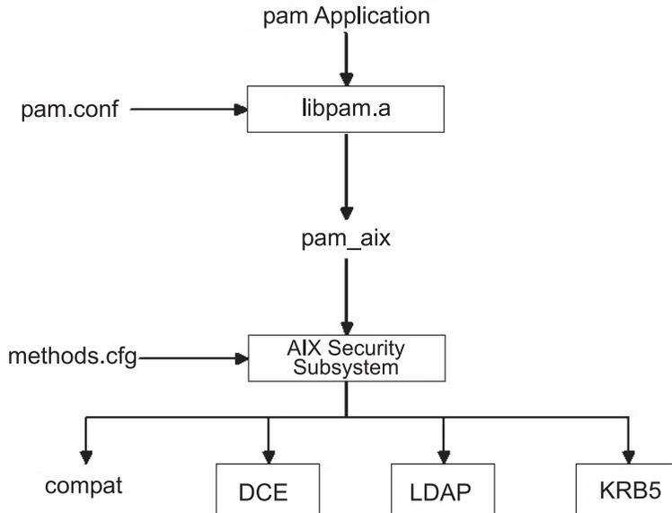
Figure 5. PAM Application to AIX Security Subsystem Path. This illustration shows the path a PAM application API call will follow if the `/etc/pam.conf` file is configured to make use of the `pam_aix` module. As shown in the diagram, the integration allows users to be authenticated by any of the loadable authentication modules (DCE, LDAP, or KRB5) or in UNIX files (`compat`).
