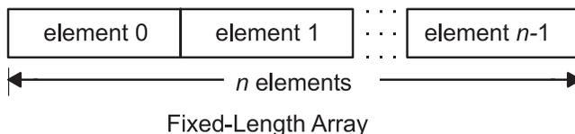
Figure 16. Fixed-Length Array. This diagram shows from the left, element 0, element 1, a series of dots to signify the elements between element 1 and element  $n-1$ . The length is equal to  $n$  elements.
