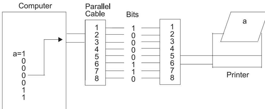
Figure 30. Parallel Communications Port
