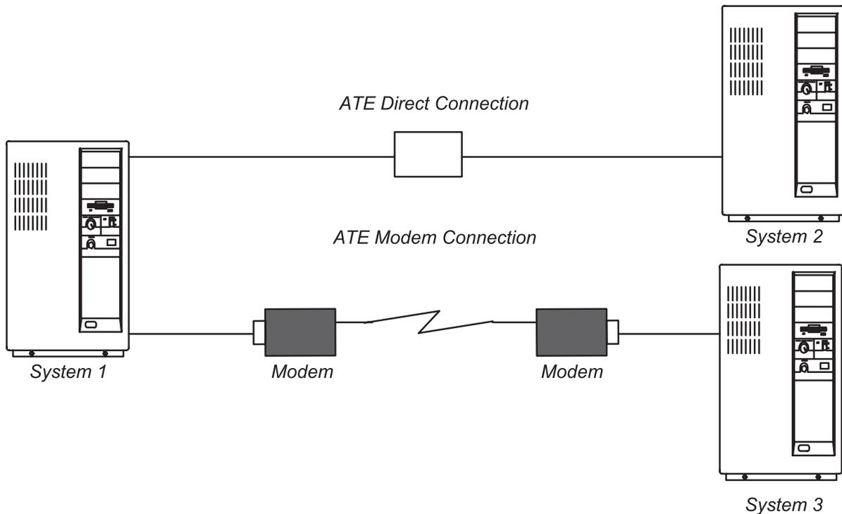
Figure 42. ATE Connection Types
