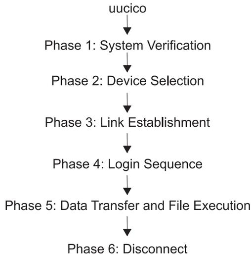
Figure 46. BNU Conversion Flow Diagram. This illustration shows the flow and different phases of BNU conversion. From **uucico** at the top, data is passed to Phase 1-System Verification, then Phase 2-Device Selection, and Phase 3-Link Establishment, then Phase 4-Login Sequence, next Phase 5-Data Transfer and File Execution and last, Phase 6-Disconnect.
