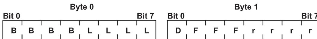
Figure 27. Routing Control Field. This illustration shows byte 0 and byte 1 of a routing control field. The eight bits of byte one are B, B, B, B, L, L, L, L. The eight bits of byte 1 are D, F, F, F, r, r, r, r.
