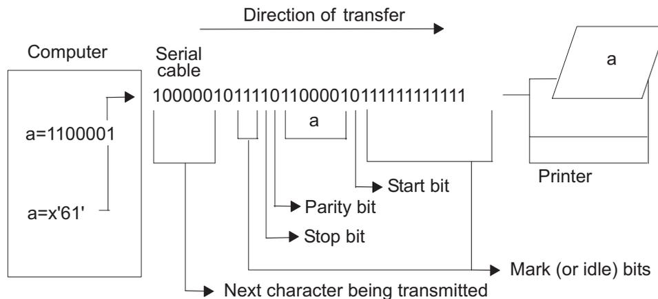
Figure 37. Start, Stop, and Mark Bits
