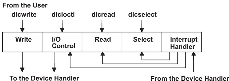
Figure 45. Standard Kernel Device Manager. This illustration shows the internal structure of a DLC device manager. This structure consists of a Write, I/O Control, Read, Select, and Interrupt Handler. The Device Manager receives information from the user where it is passed to the various areas before it is passed on to the Device Handler.
