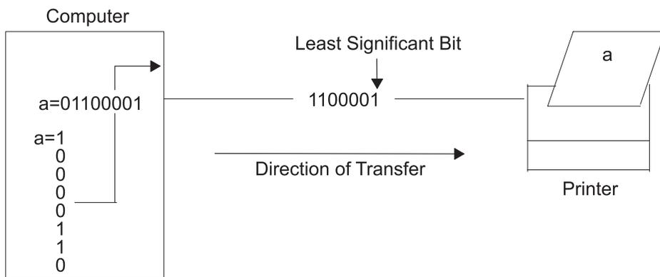
Figure 31. Serial Communications Port
