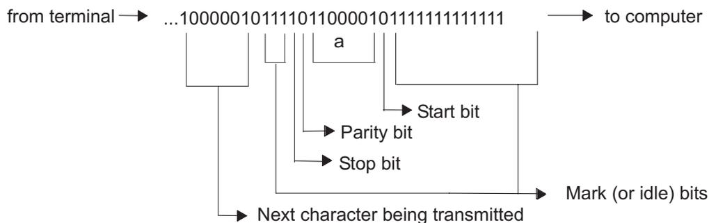
Figure 35. Mark (idle) Bits in the Data Stream
