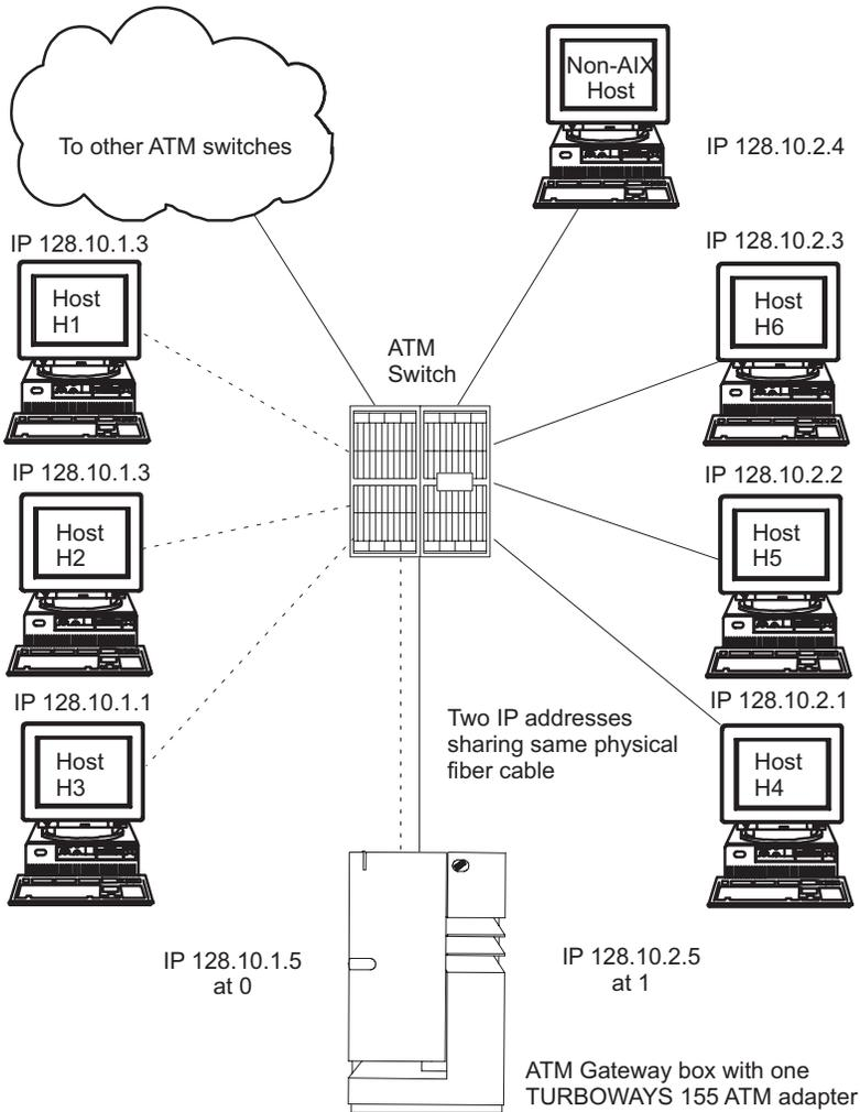
Figure 15. Representative ATM Network. This illustration depicts an ATM network laid out in a typical star topology. In the center of the star is the ATM switch. Numbered IP hosts are branched off of the switch as are links to other ATM switches and one ATM gateway box and adapter.
