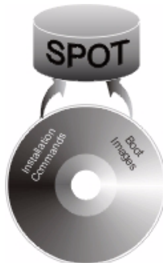
Figure 5. An example of a SPOT resource. This illustration shows that a SPOT resource contains the installation commands used to install the installation images from the LPP_Source resource onto a system. The SPOT is also used to build the necessary boot images to boot a client system.
