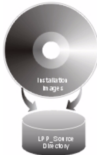
Figure 4. An example of an LPP_Source resource. This illustration shows that when an LPP_Source resource is created, installation images are copied from the product CD-ROM to the LPP_Source directory.
