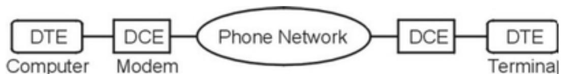
A DTE is any device that drives the transmit data signal and listens to the receive data signal. A DCE is any device that listens to the transmit data signal and drives the receive data signal.
