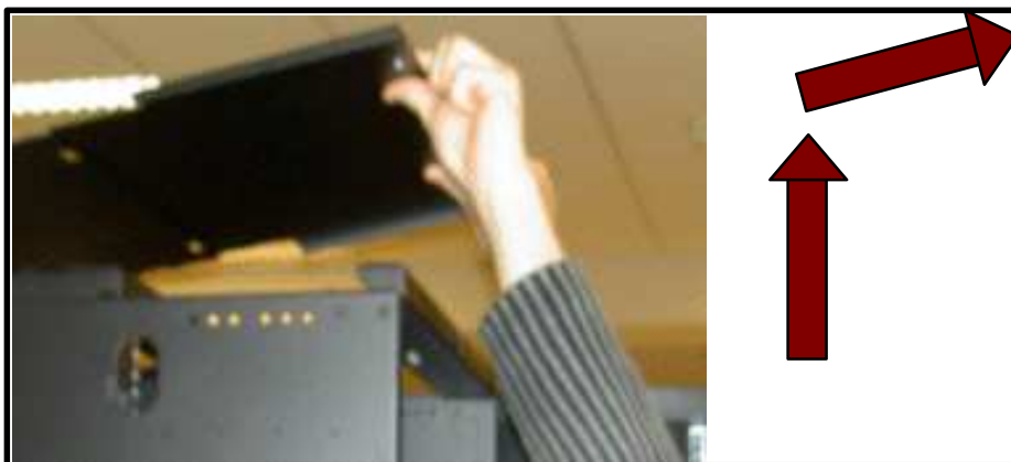
Figure 42. Removing the top cover
