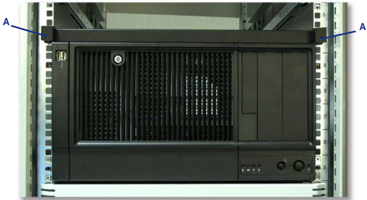
Figure 74: Securing the server to the rack cabinet
