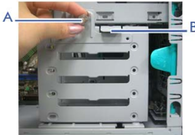
Figure 89: HDD Bracket Screw and Latch
