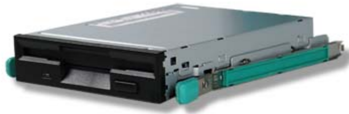
Figure 88: Attaching the Slide Rails
