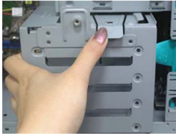
Figure 92: Sliding the HDD Bracket out
