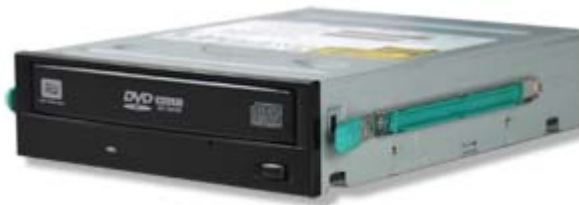
Figure 89: Attaching the Slide Rails
