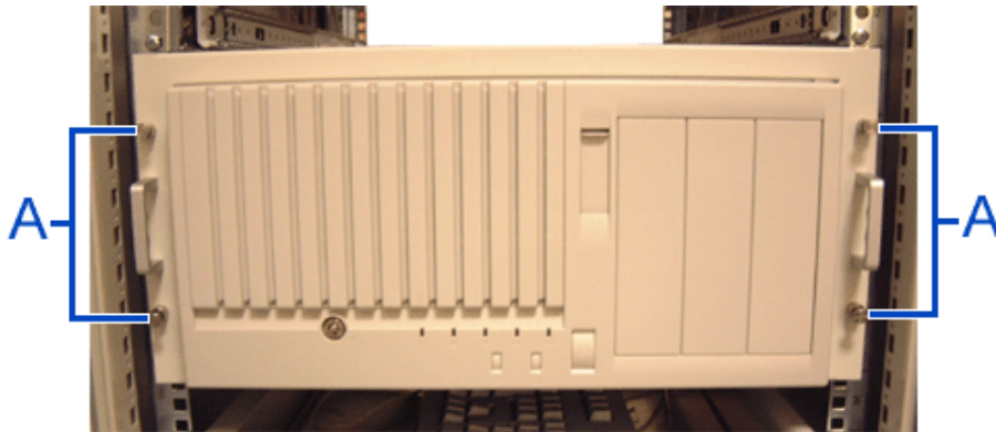
Figure 34: Securing the server to the rack cabinet
