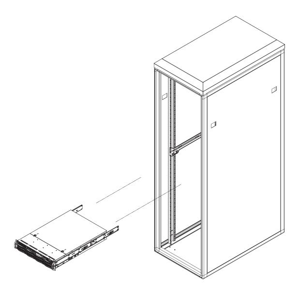
Figure 2-2. Installing the Server into a Rack
