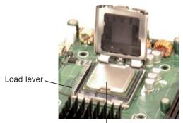
CPU installed in socket
