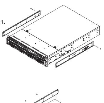
Figure 2-1. Installing Chassis Rails
