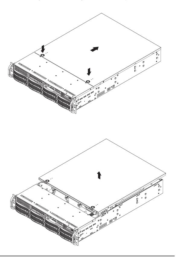
Figure 2-3. Accessing the Inside of the System
