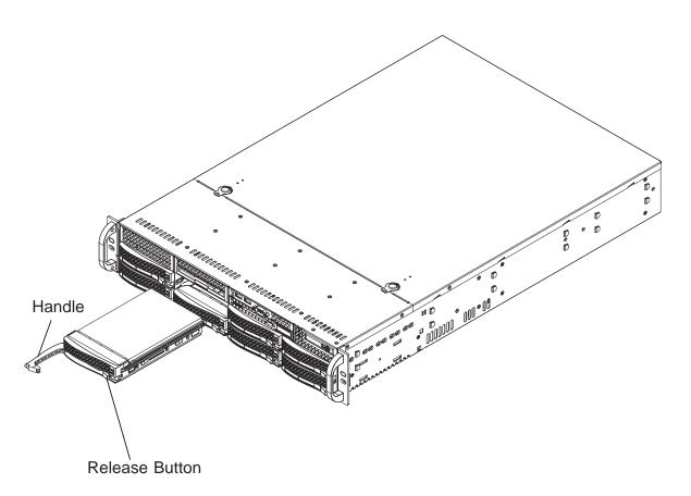
Figure 6-4. Removing a Serial ATA Drive Carrier
