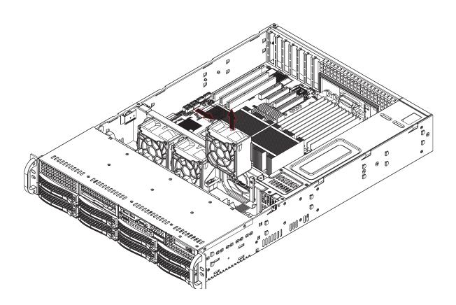
Figure 6-2. Removing System Cooling Fans
