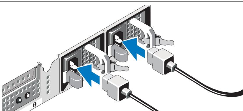
Connect the system's power cable(s) to the system and, if a monitor is used, connect the monitor's power cable to the monitor.
