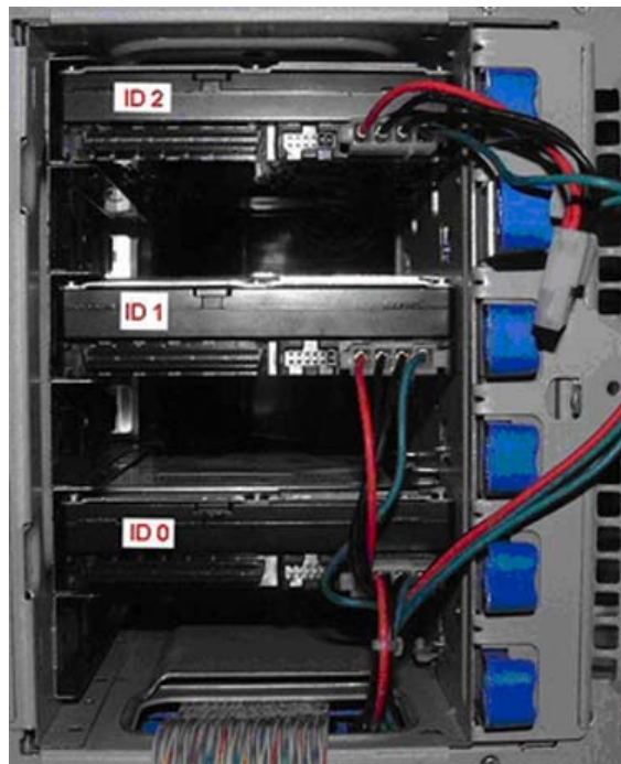
Figure 59: Three SCSI Hard Disk Drives Installed
