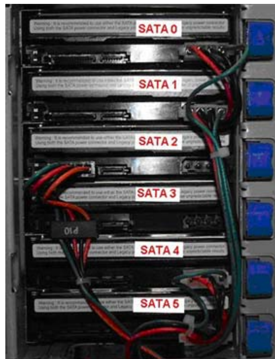
Figure 62: Using a MOLEX Power Port
