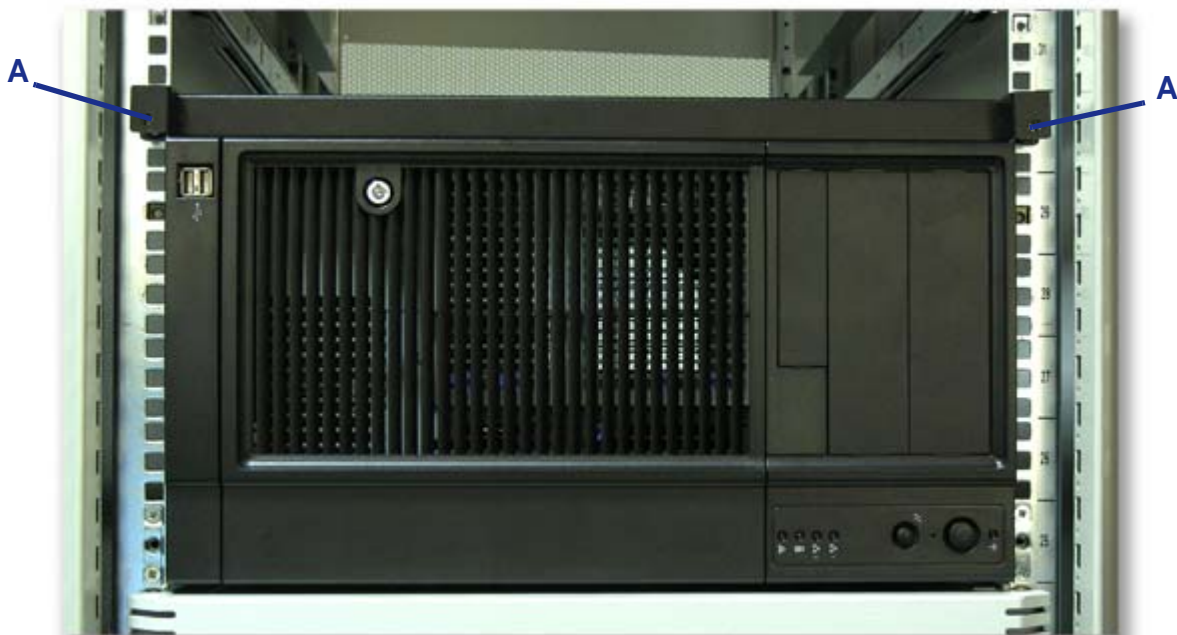
Figure 32: Securing the server to the rack cabinet
